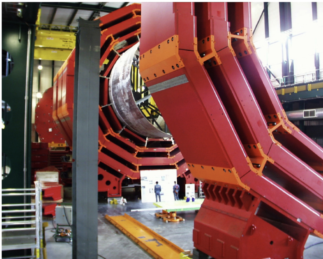
Figure 4.4: A view of the CMS solenoid yoke at an early stage of magnet assembly. The central barrel supports the vacuum chamber of the superconducting coil. At the rear, one of the closing endcap disks is visible [15].
