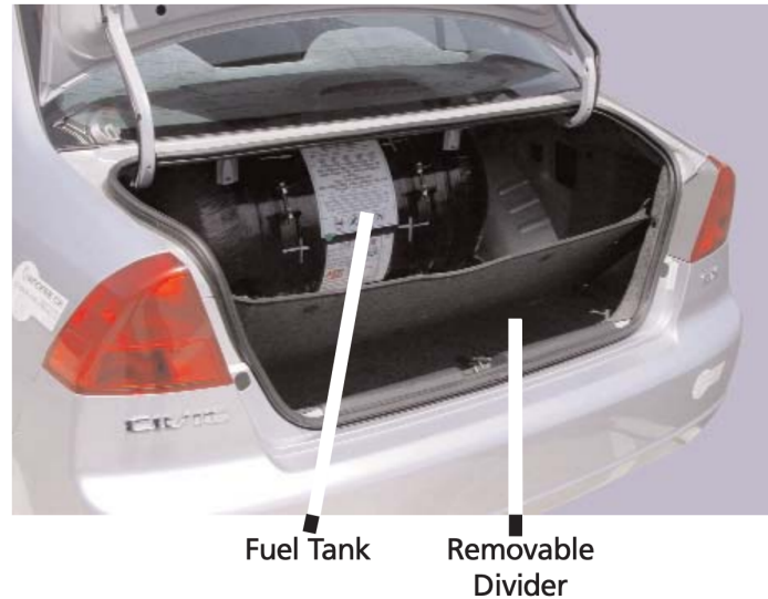
Figure 1.3: Trunk of a Honda Civic showing an 8 gasoline gallon equivalent CNG tank with remaining space. (Source: Honda) [39]
