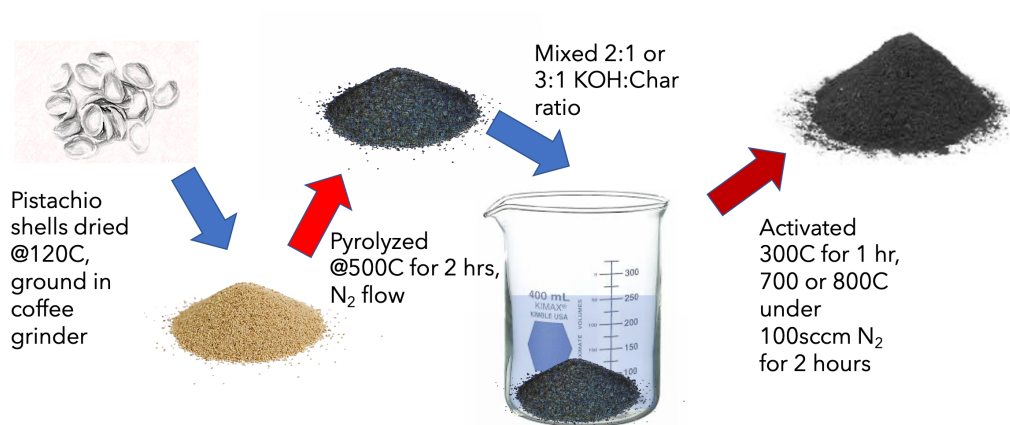
Figure 5.1: Synthesis approach to pistachio shell-derived activated carbon production.
