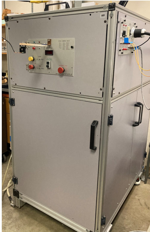
Figure 2.7: The pulse-forming network designed to extend the duration of the plasma jet.
