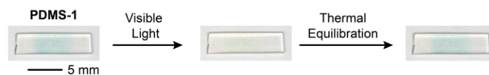
Figure 3.11 Photographs of a film of mechanochemically active PDMS-1 containing 2.5 wt% of mechanophore crosslinker ( \pm )- 5a after manual tensile activation and subsequent immersion for 90 s in a solution of 4-methoxy- N -methylaniline (7 mM in 9:1 DCM/HFIP). The blue–green colored DASA is generated in the gauge region of the sample. Subsequent exposure to visible light irradiation for 30 s induces photoswitching to the colorless closed form of the DASA. Cessation of irradiation leads to rapid regeneration of the colored form under ambient conditions.
