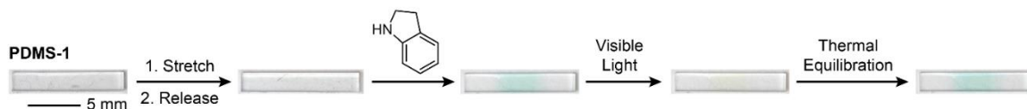
Figure 3.12 Photographs of a film of mechanochemically active PDMS-1 containing 2.5 wt% of mechanophore crosslinker ( \pm )- 5a after manual tensile activation and subsequent immersion for 90 s in a solution of indoline (0.5 vol% in 9:1 DCM/HFIP). The blue–green colored DASA is generated in the gauge region of the sample. Exposure to visible light irradiation for 30 s induces photoswitching to the colorless closed form of the DASA. Cessation of irradiation results in the rapid regeneration of the colored triene form under ambient conditions.
