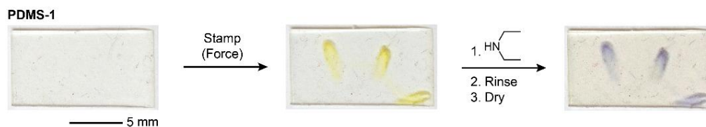
Figure 3.15 Photographs of a film of mechanochemically active PDMS-1 containing 2.5 wt% of mechanophore crosslinker ( \pm )- 5a after localized compression via stamping and subsequent exposure to diethylamine vapor for 7 min. The purple-colored DASA is generated in the force-activated region of the sample.
