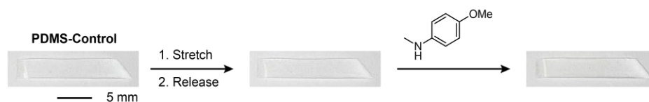
Figure 3.16 Photographs of control film PDMS-Control containing 2.5 wt% of monofunctional mechanophore ( \pm )- 5b after manual tensile activation and subsequent immersion for 90 s in a solution of 4-methoxy- N -methylaniline (7 mM in 9:1 DCM/HFIP). No change in color is observed, indicating that force must be applied across the mechanophore to achieve activation and DASA formation.
