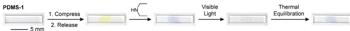
Figure 3.13 Photographs of a film of mechanochemically active PDMS-1 containing 2.5 wt% of mechanophore crosslinker ( \pm )- 5a after manual compression and subsequent immersion for 90 s in a solution of diethylamine (0.5 vol% in DCM). The purple colored DASA is generated in the compressed region of the sample. Exposure to visible light irradiation for 30 s induces photoswitching to the colorless closed form of the DASA. Cessation of irradiation results in the regeneration of the colored triene form after several minutes under ambient conditions.
