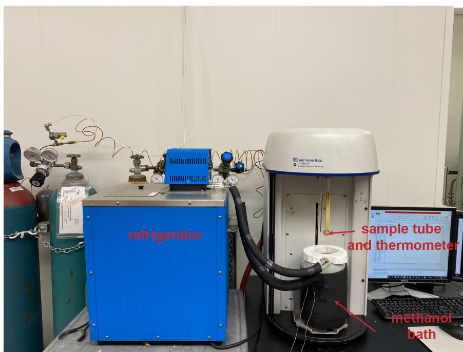
Figure 3.2: The setup of the krypton adsorption measurement at different temperatures. The refrigerator cycles methanol at different temperatures. The methanol in the refrigerator goes through the condensing coil in the bath bottle and delivers heat to the methanol in the bath. After waiting for enough time and when the two types of methanol reach equilibrium, the methanol bath bottle is raised up and the sample tube is sunk inside the bath. One thermometer sensor is attached to the sample tube, and another sensor is sunk inside the bath. Temperature is measured every second during the experiment.
