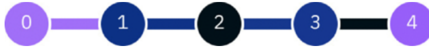
Figure 3.4: Layout of IBM Q device Bogota. It consists of 5 transmon qubits arranged in a linear chain. The figure is reproduced from [85].
