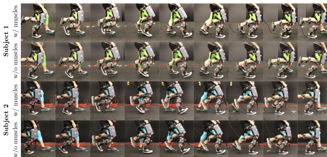
Figure 5.12: Gait tiles of experimental demonstration on AMPRO3 for gaits generated without or with muscle model constraints for two subjects.
