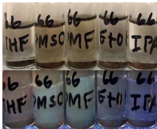
Figure 5.14 Images of Si NCs reacted with 10 mM aldehyde in methanol solution under visible light (top) and under UV light (bottom). The NCs are dispersed in solvents of varying polarity, i.e., THF, DMSO, DMF, ethanol, and IPA (left to right). Weak photoluminescence observed for dispersion in DMSO and DMF, but its origin is still unclear.
