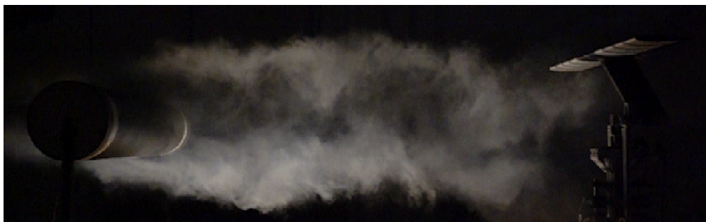
Figure 3.4: Smoke visualizations showing the turbulent wake of a standard cylinder at Reynolds number Re_D = 50000 . This was taken in the Caltech Center for Autonomous Systems and Technologies fan-array wind-tunnel at lower Reynolds number for purposes of visualization. The actual flow conditions used for testing and training were too turbulent for effective smoke visualization.
