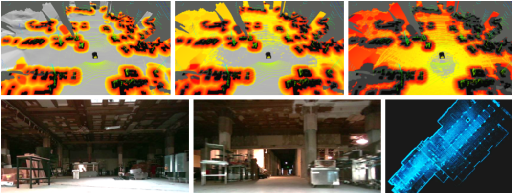
Figure 3.16: Traversability analysis results for Husky in an abandoned subway experiment. Top left to right: Risk maps at three varying risk levels: \alpha = 0.1, 0.5, 0.9 , respectively. Colors correspond to CVaR value (white: safe ( r \leq 0.05 ), yellow to red: moderate ( 0.05 < r \leq 0.5 ), black: risky ( r > 0.5 )). Also shown are the most recent LiDAR measurements (green points). Bottom left and middle: Front and right on-board cameras observing the same location. Bottom right: Completed top-down map of the environment after autonomous exploration. Bright dots are pillars, which are visible in the camera images. The effect of these risk analyses results in intuitive outcomes - for example, a low pile of metal, while probably traversable, should be avoided if possible. When the region has inadequate sensor coverage, the risk will be high. When the robot is closer and the sensor coverage is good, then the CVaR cost will decrease, yielding a more accurate risk assessment. This results in more efficient and safer planning when compared to deterministic methods.
