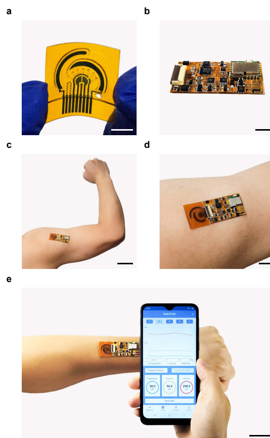
Figure D-1. Integrated flexible NutriTrek prototype for personalized nutritional monitoring. a,b , Optical photos of a wearable NutriTrek prototype consisting of a flexible, disposable microfluidic sensor patch ( a ) for autonomous sweat stimulation and sweat analysis and a flexible printed circuit board (FPCB) ( b ) for in situ electrochemical control, signal processing, and wireless communication. Scale bars, 5 mm ( a ) and 1 cm ( b ). c,d , Optical photos of the integrated system on the body. Scale bars, 5 cm ( c ) and 1 cm ( d ). e , Optical photo of a flexible NutriTrek patch interfacing with the custom cell phone app for real-time data collection. Scale bar, 3 cm.
