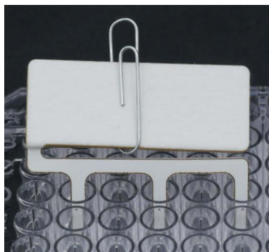
Figure 3.6: Photograph of the lateral flow device for viral RNA detection. The lateral flow device with three channels resting within their respective wells on a 96-well plate.
