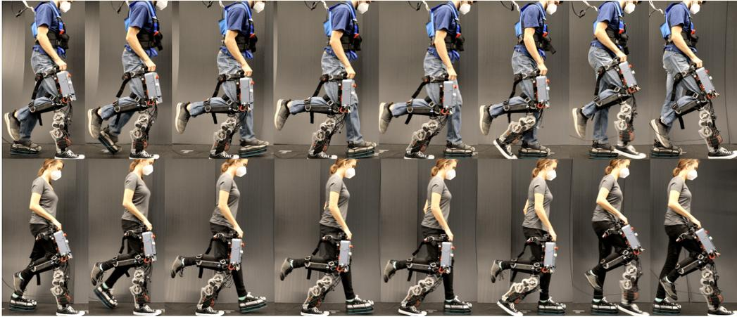
Figure 8.4: Gait tiles of 2 subjects walking on a rubber floor with the force sensing ID-CLF-QP prosthesis controller.
