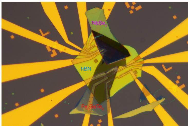
Figure 1.6: A device consisting of pre-fabricated Au electrodes, with a flake of  $\text{Fe}_3\text{GeTe}_2$  and a flake of  $\text{NbSe}_2$  stacked so that the resistance of the junction between them could be measured.
