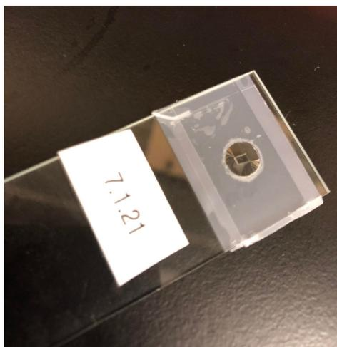
Figure 2.2: An example polymer stamp, showing a pre-cut PDMS square that supports the thin PC film, which is attached to the slide using scotch tape with a window cut out.
