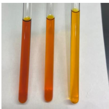
Figure 3.18. W(CNDipp) 6 (5 mol%), TMP (2 equiv), and 1-(2-iodobenzyl)-pyrrole substrate (50 mM) reactions in benzene (left), DFB (center), and DFB with 0.2M TBAPF 6 (right) after 1 hour of irradiation.
