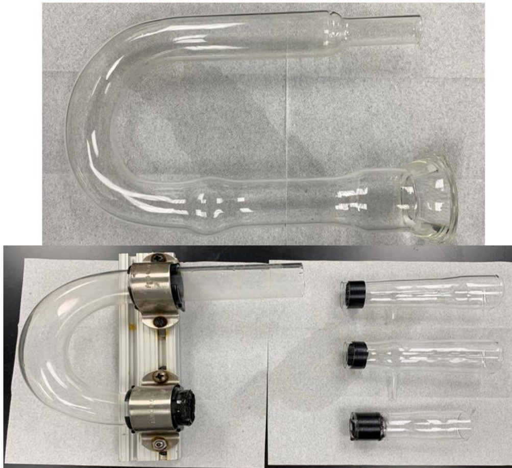
Figure 2.3: Images of the two curved glass pipes that simulated the aortic arch. Top: Curved aorta with a 34 mm sinus bulge. Bottom: Curved glass aorta with interchangeable sinus bulge sizes (bottom right) Note that some sinuses had dye ports installed.
