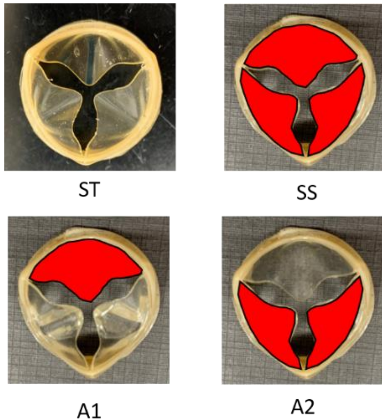
Figure 2.2: 27mm Polymer Prosthetic Heart Valves developed by Foldax. Four different experimental configurations are shown where red overlays on the leaflets indicate that they have been stiffened from 0.05 mm to 0.5 mm
