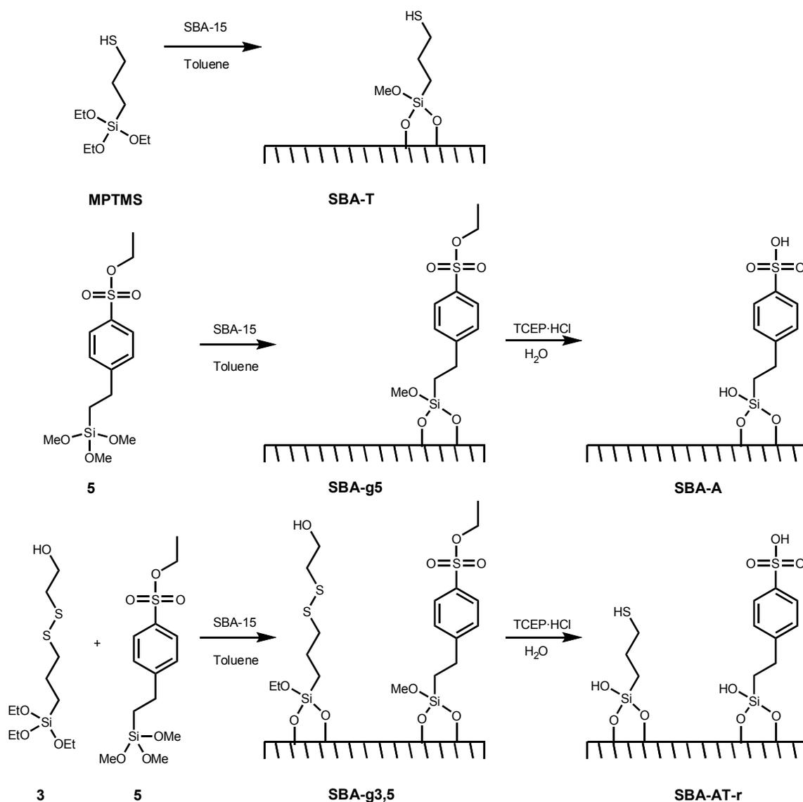
**Scheme 3.3.** (Top) Grafting 3-mercaptopropyltrimethoxysilane (MPTMS) onto SBA-15 generates **SBA-T**, containing only thiol sites. (Middle) Grafting sulfonate ester precursor **5** generates intermediate **SBA-g5**, which is hydrolyzed to **SBA-A**, containing only acid sites. (Bottom) Grafting both disulfide **3** and sulfonate ester **5** generates intermediate **SBA-g3,5** which is deprotected to form **SBA-AT-r**, containing randomly-distributed acid and thiol sites.
