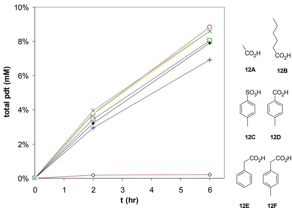
**Figure 5.10.** Total yield of aldol product formation (alcohol + olefin) catalyzed by **SBA-PA-TMS** + homogeneous acid: no acid (◆), **12A** (+), **12B** (×), **12C** (◇), **12D** (○), **12E** (●), **12F** (□). Reaction conditions: 6 mL of 50 mM *p*-nitrobenzaldehyde solution in acetone, 10 mol% heterogeneous amine, 10 mol% acid, 25°C
