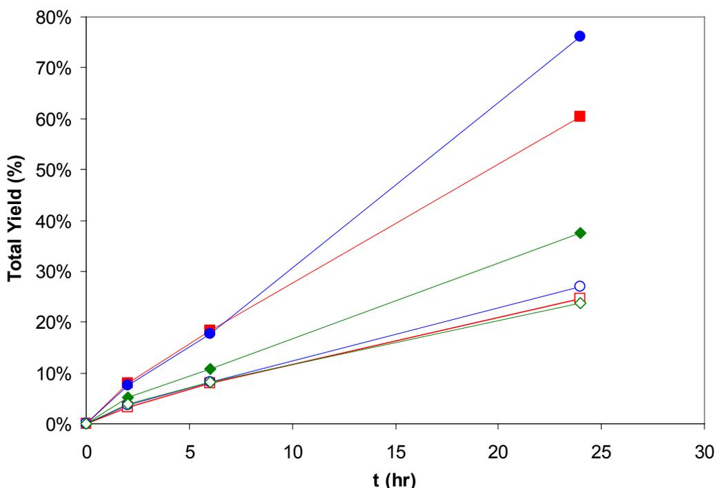
**Figure 5.9.** Comparison of kinetic profiles for aldol reaction with unsilylated (filled symbols) and silylated (open symbols) heterogeneous catalysts: **SBA-PA(-TMS)** (■, □), **SBA-PA-CA-r(-TMS)** (●, ○), and **SBA-PA-CA-p(-TMS)** (◆, ◇). Reaction conditions: 50 mM *p*-nitrobenzaldehyde solution in acetone, 10 mol% amine, 25°C
