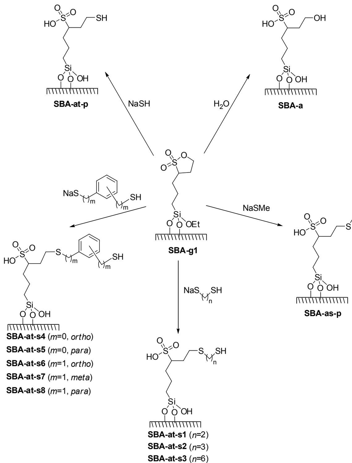
**Scheme 2.3.** Ring-opening of surface-bound sultone to form sulfonic acid-containing materials
