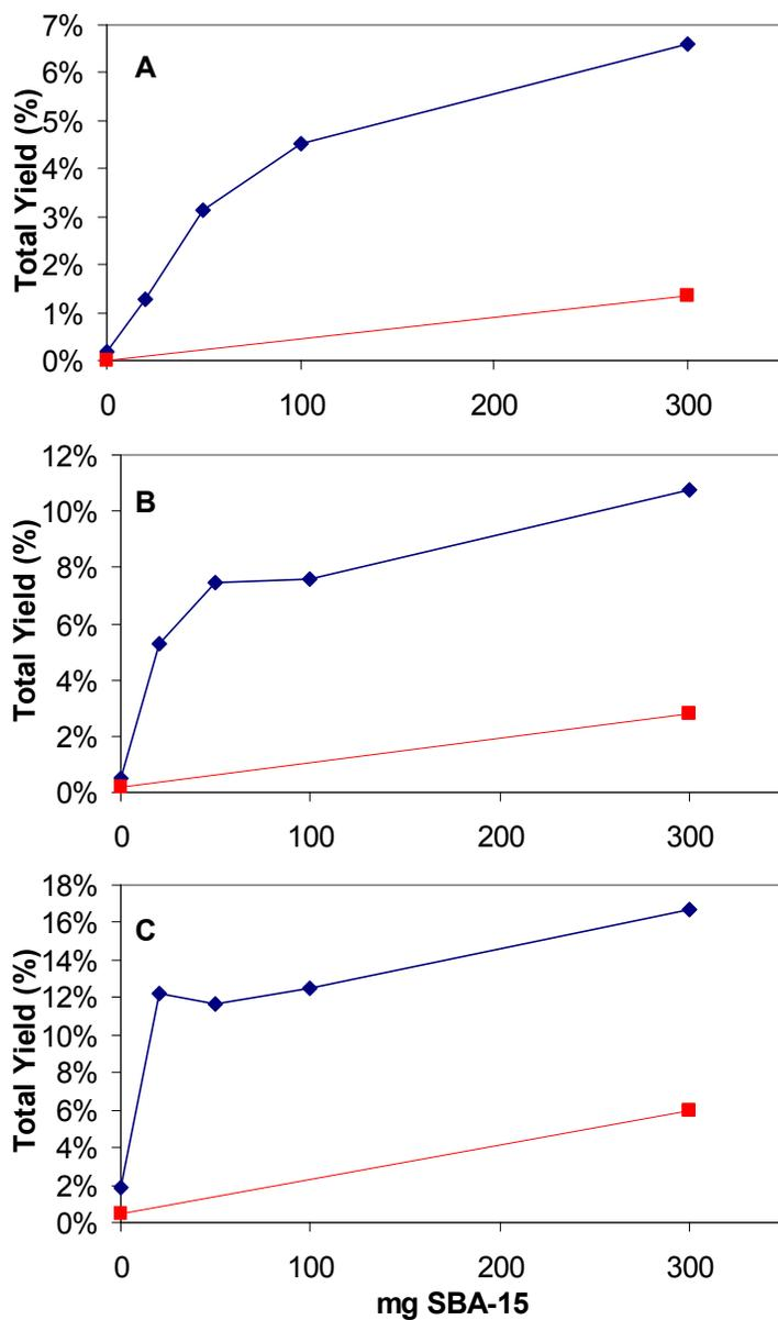
**Figure 5.11.** Total yield of aldol product formation (alcohol + olefin) catalyzed by homogeneous amine + unsilylated SBA-15 (◆) or silylated SBA-15 (■) after reaction times of: (A) 2 hrs, (B) 6 hrs, and (C) 24 hrs. Reaction conditions: 6 mL of 50 mM *p*-nitrobenzaldehyde solution in acetone, 10 mol% propylamine, 25°C
