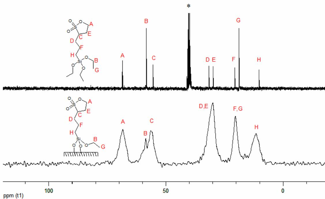
**Figure 2.3.** <sup>13</sup>C NMR (DMSO-*d*<sub>6</sub>) of silane **1** (top) and <sup>13</sup>C{<sup>1</sup>H} CP/MAS NMR of **SBA-g1** (bottom). \* denotes solvent peak.
