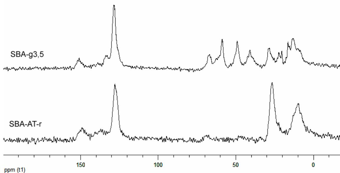
**Figure 3.5.**  $^{13}\text{C}\{^1\text{H}\}$  CP/MAS NMR spectra of **SBA-g3,5** (top) and **SBA-AT-r** (bottom). The ethyl ester peak (67 ppm) and mercaptoethanol peaks (41 ppm, 60 ppm) are absent in **SBA-AT-r** following deprotection. The residual ethoxy (16 ppm, 58 ppm) and methoxy peaks (49 ppm) are also hydrolyzed in the deprotection process. The small peak in the **SBA-g3,5** spectrum at 21 ppm is due to residual adsorbed toluene.
