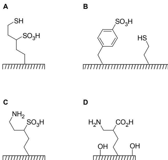
**Figure 1.2.** Summary of the four polyfunctional SBA-15 catalysts described in this work.
