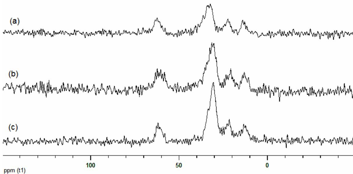
**Figure 2.11.**  $^{13}\text{C}\{^1\text{H}\}$  CP/MAS NMR spectra of alkyl spacer materials. (a) **SBA-at-s1**
