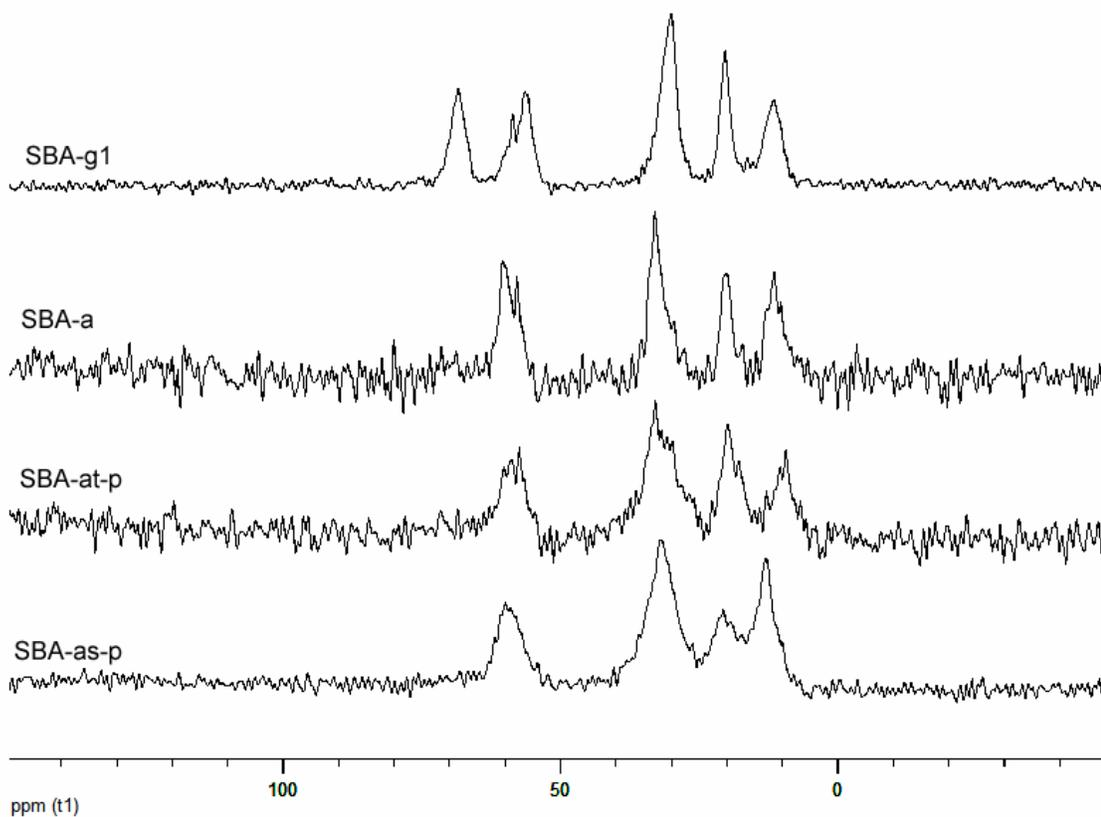
**Figure 2.6.** Comparison of  $^{13}\text{C}\{^1\text{H}\}$  CP/MAS NMR spectra of **SBA-g1** (top) and sulfonic-acid-containing SBA-15 materials. The complete disappearance of the sultone peak at 68 ppm indicates complete ring-opening of the sultone.
