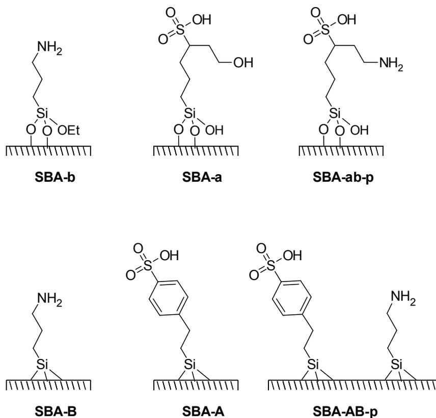
**Figure 4.3.** Summary of the grafted amine/alkylsulfonic acid SBA-15 catalysts whose synthesis is reported here (top) and the one-pot-synthesized amine/arylsulfonic acid SBA-15 catalysts of Zeidan et al.<sup>7</sup> (bottom)
