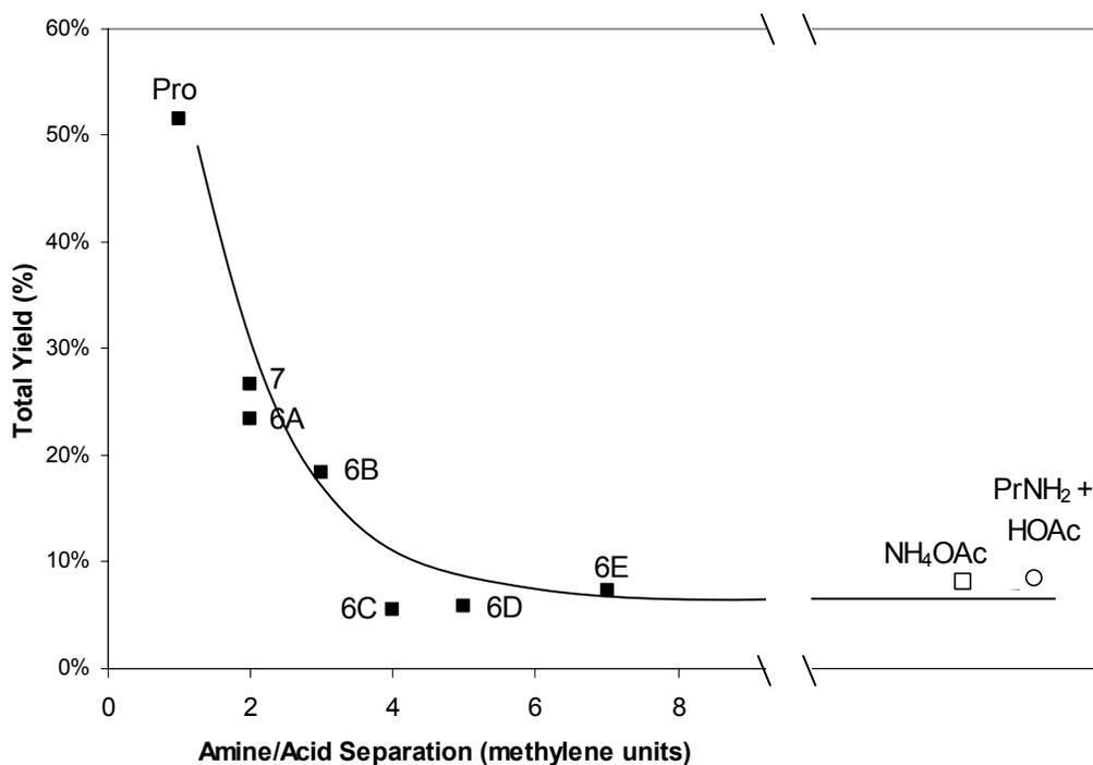
**Figure 5.4.** Total yield of aldol product formation (alcohol + olefin) for various homogeneous amino acid catalysts as a function of amine/acid separation. Reaction conditions: 50 mM *p*-nitrobenzaldehyde in 1:1 acetone/methanol, 10 mol% catalyst, 24 hrs, 25°C. The data points for ammonium acetate (□) and propylamine + acetic acid (○) are also shown, arbitrarily placed at a large amine/acid separation.
