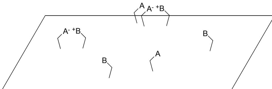
**Figure 4.1.** Schematic representation of a catalyst surface functionalized with covalently tethered, randomly-distributed acid (A) and base (B) groups. Some of these groups will be spatially isolated and unable to exchange protons, while others will be close enough to interact directly with another nearby group, allowing proton exchange and equilibration with the ion-pair form (represented by  $A^-/B^+$  pairs).
