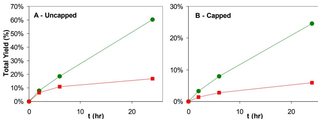
**Figure 5.12.** Kinetic profiles for aldol reaction catalyzed by SBA-15 + untethered propylamine (■) and propylamine groups tethered to silica, **SBA-PA(-TMS)** (●). In (A) the silanols of SBA-15 and **SBA-PA** are uncapped, and in (B) silanols are capped with TMS groups. Reaction conditions: 6 mL of 50 mM *p*-nitrobenzaldehyde solution in acetone, 10 mol% amine, 300 mg silica, 25°C
