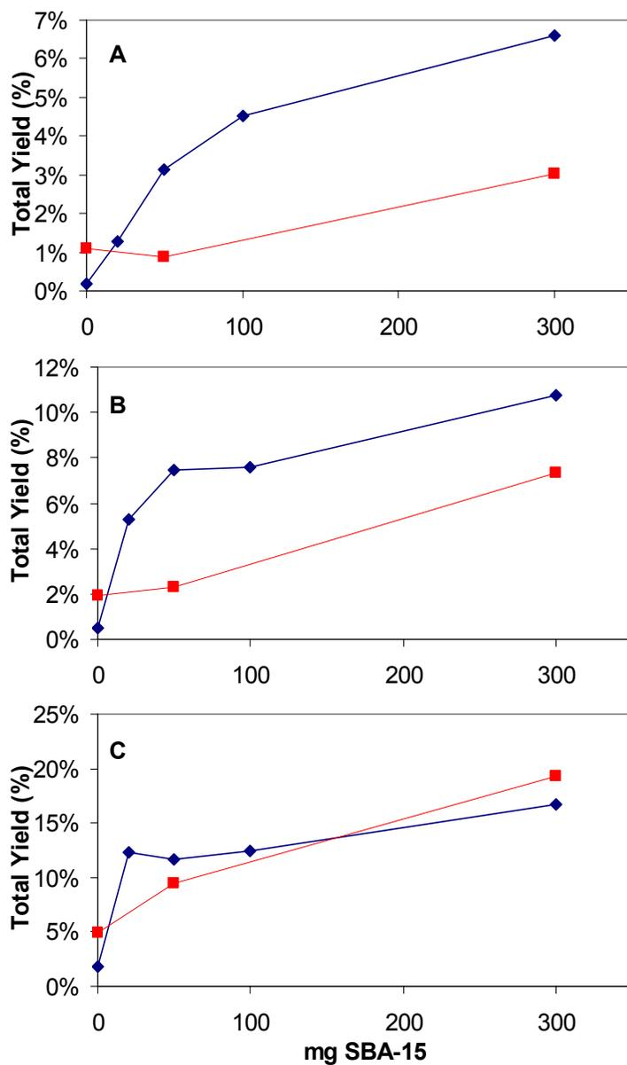
**Figure 5.14.** Total yield of aldol product formation (alcohol + olefin) catalyzed by homogeneous amine + SBA-15 after reaction times of: (A) 2 hrs, (B) 6 hrs, and (C) 24 hrs. Reaction conditions: 6 mL of 50 mM *p*-nitrobenzaldehyde solution in acetone (◆) or 1:1 acetone/methanol (■), 10 mol% propylamine, 25°C
