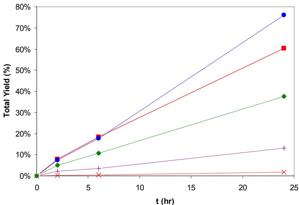
**Figure 5.7.** Kinetic profiles for aldol reaction with heterogeneous amine/acid catalysts. Reaction conditions: 50 mM *p*-nitrobenzaldehyde in acetone, 10 mol% heterogeneous amine and/or 10 mol% carboxylic acid, 25°C. Catalysts: **SBA-PA-CA-r** (●), **SBA-PA** (■), **SBA-PA-CA-p** (◆). For comparison purposes, data for homogeneous catalysts is also shown: propylamine + acetic acid (+), propylamine (×).
