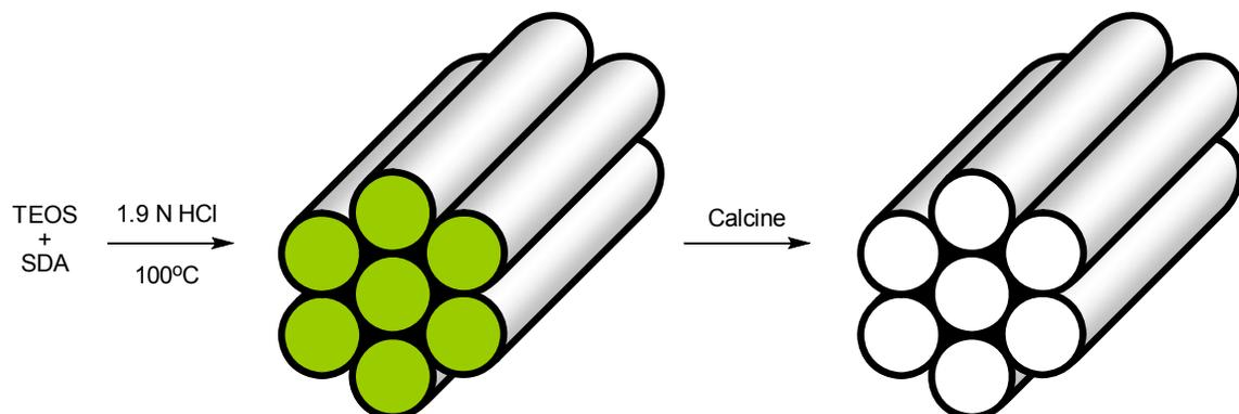
**Figure 1.1.** Synthesis of SBA-15. The structure-directing agent (SDA) is a triblock copolymer of ethylene oxide (EO) and propylene oxide (PO) with formula  $(EO)_{20}(PO)_{70}(EO)_{20}$ . The calcination process (at  $550^{\circ}\text{C}$ ) burns out the SDA, leaving the pores empty. The silica source is tetraethyl orthosilicate (TEOS).
