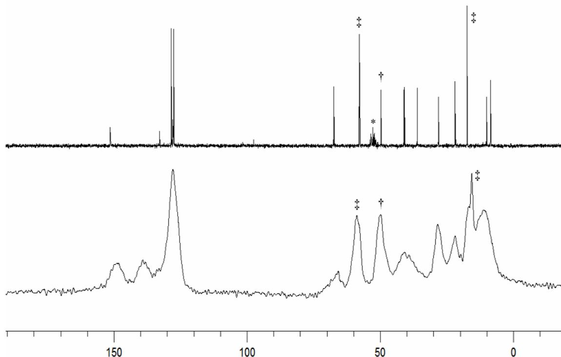
**Figure 3.2.** The  $^{13}\text{C}$  NMR spectrum of bissilane **4** (top) and  $^{13}\text{C}\{^1\text{H}\}$  CP/MAS spectrum of **SBA-g4** (bottom) confirm that the disulfide/sulfonate ester structure remains intact following the grafting reaction.
