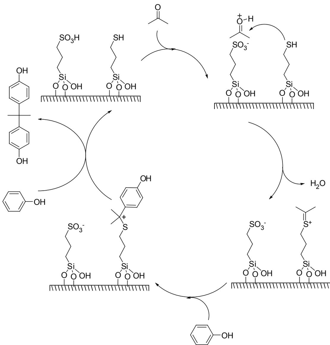
**Figure 2.1.** Proposed catalytic cycle for the synthesis of bisphenol A over a bifunctional acid/thiol catalyst. The propylidene sulfonium (bottom right) and carbocation (bottom left) intermediates are in close proximity to the pore wall, which provides the steric driving force that favors the formation of the *p,p'* isomer of bisphenol A.
