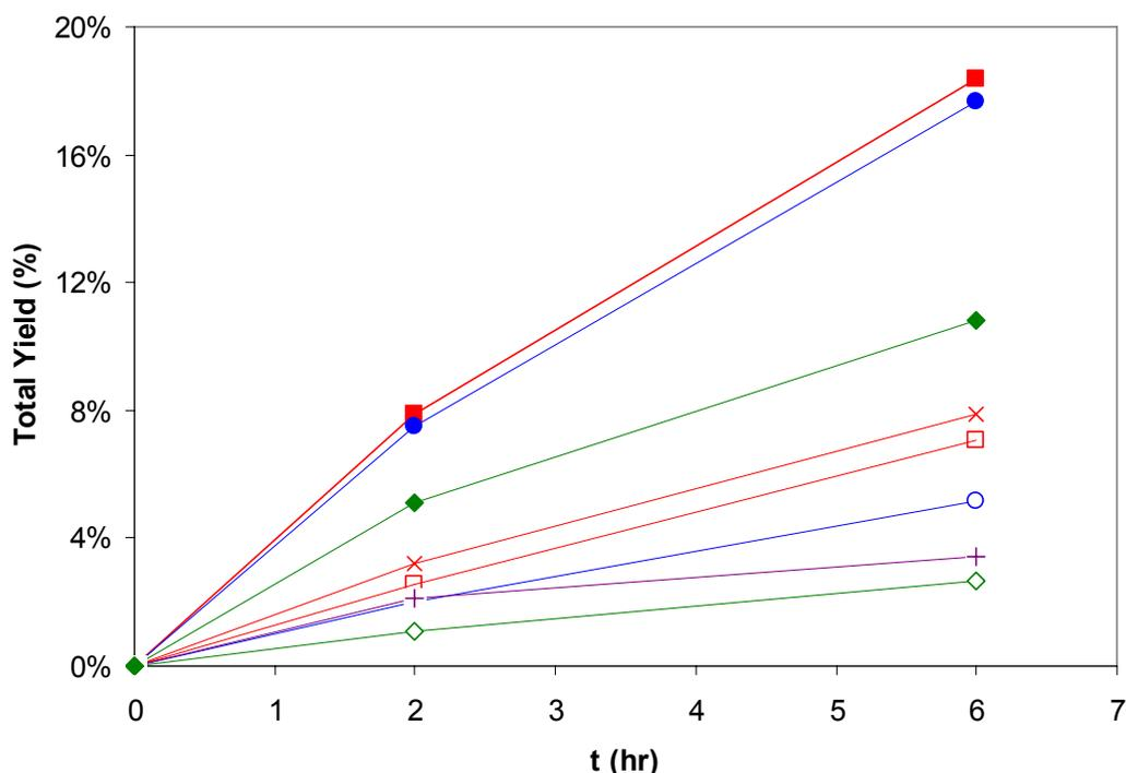
**Figure 5.13.** Comparison of kinetic profiles for aldol reaction with heterogeneous catalysts **SBA-PA** (■,□), **SBA-PA-CA-r** (●,○), and **SBA-PA-CA-p** (◆,◇). Reaction solvent: acetone (filled points) or 1:1 acetone/methanol (open points). For comparison purposes, the data for **SBA-PA-TMS** in acetone (×) and propylamine/acetic acid in 1:1 acetone/methanol (+) are also shown.
