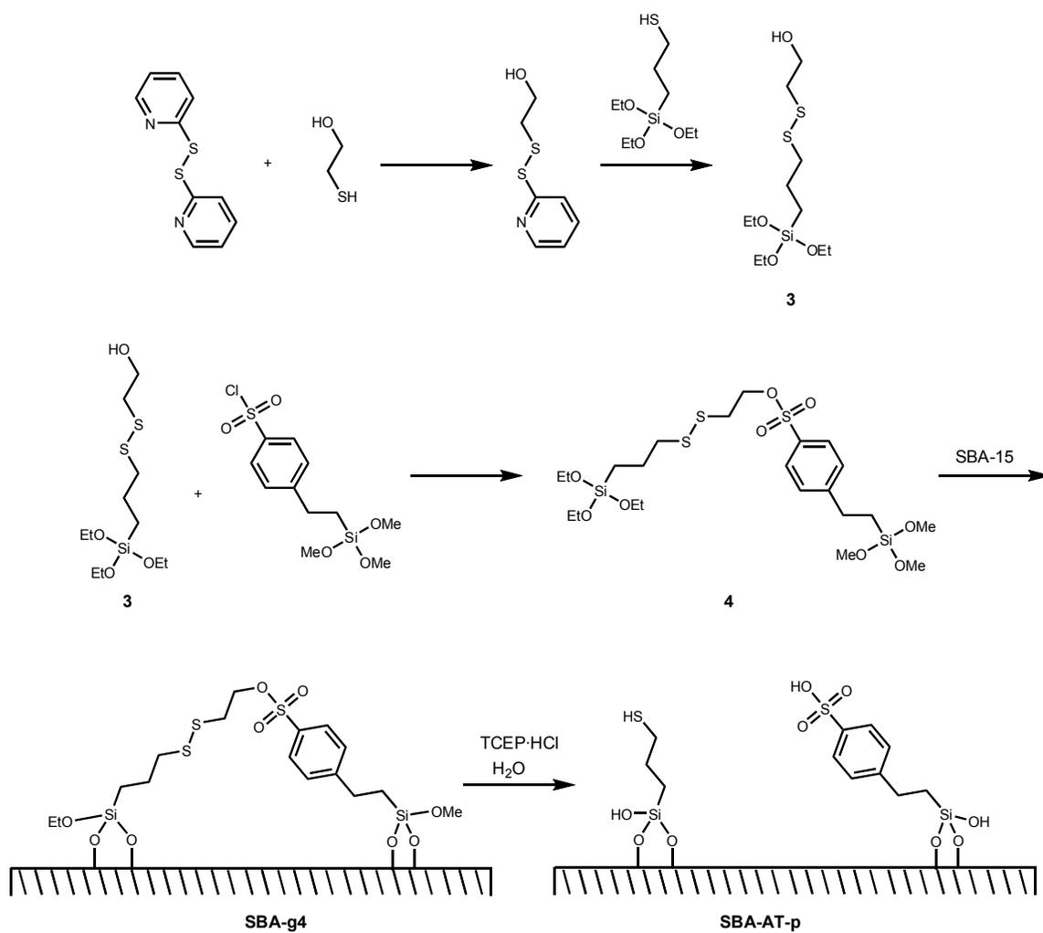
**Scheme 3.2.** Synthesis of disulfide silane **3** (top) and bissilane **4** (middle) and the grafting of **4** onto SBA-15 to generate disulfide/sulfonate ester-functionalized silica **SBA-g4** (bottom), the mercaptoethanol linker of which is cleaved to generate the acid/thiol-paired material **SBA-AT-p**
