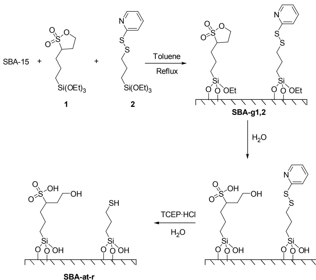
**Scheme 2.4.** Simultaneous grafting of silanes **1** and **2** to form randomly-bifunctionalized sultone/disulfide material **SBA-g1,2** and subsequent deprotection to form random acid/thiol material **SBA-at-r**
