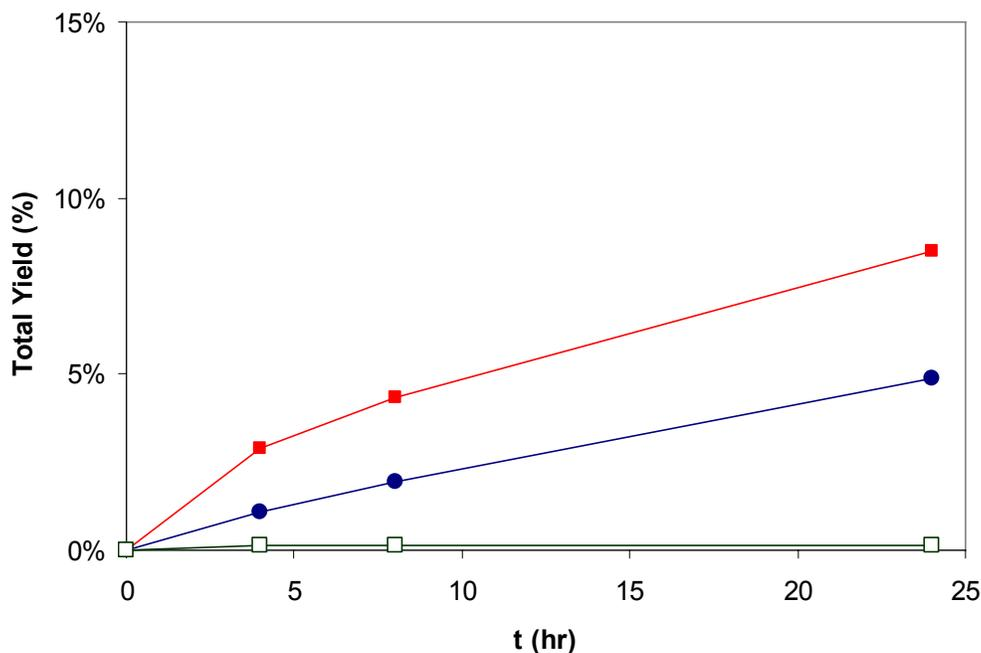
**Figure 5.2.** Aldol reaction yield (alcohol + olefin) with homogeneous catalysts: acetic acid (□), propylamine (●), and propylamine + acetic acid (■). Reaction conditions: 50 mM *p*-nitrobenzaldehyde in 1:1 acetone/methanol, 10 mol% each catalyst, 25°C
