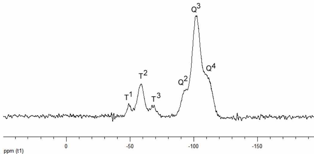
**Figure 2.2.** <sup>29</sup>Si{<sup>1</sup>H} CP/MAS NMR spectrum of **SBA-g1** (loading = 0.7 mmol/g)
