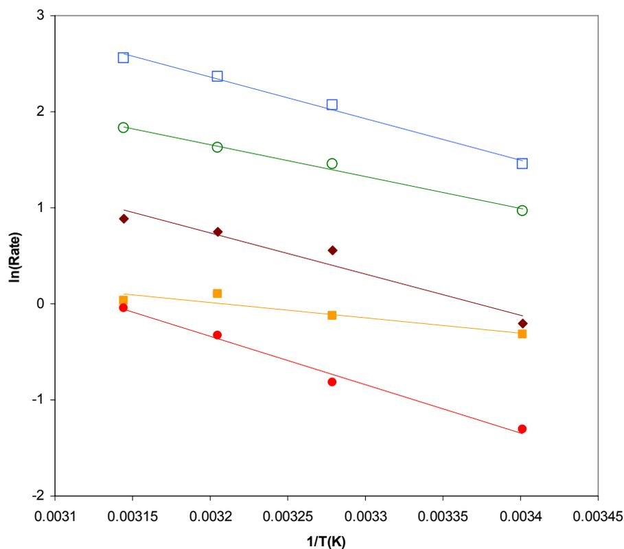
**Figure 5.6.** Arrhenius plots for homogeneous amino acid aldol catalysts. Proline (□), **7** (○), **6C** (◆), propylamine + acetic acid (■), propylamine (●). Rate data refer to the initial rate of product formation (alcohol + olefin) over the first 1–2 hours of reaction (conversion < 12%).
