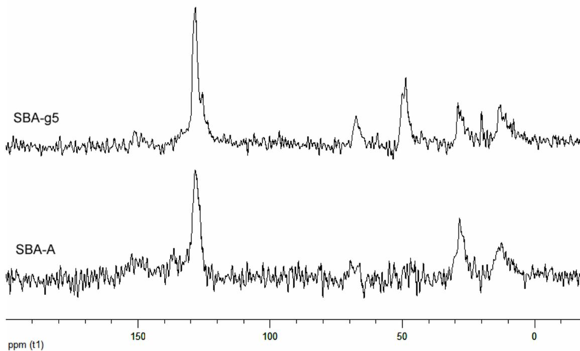
**Figure 3.4.**  $^{13}\text{C}\{^1\text{H}\}$  CP/MAS NMR spectra of **SBA-g5** (top) and **SBA-A** (bottom). The peak at 67 ppm is due to the ethyl ester and is nearly absent in **SBA-A**. The small peak in the **SBA-g5** spectrum at 21 ppm is due to residual adsorbed toluene.
