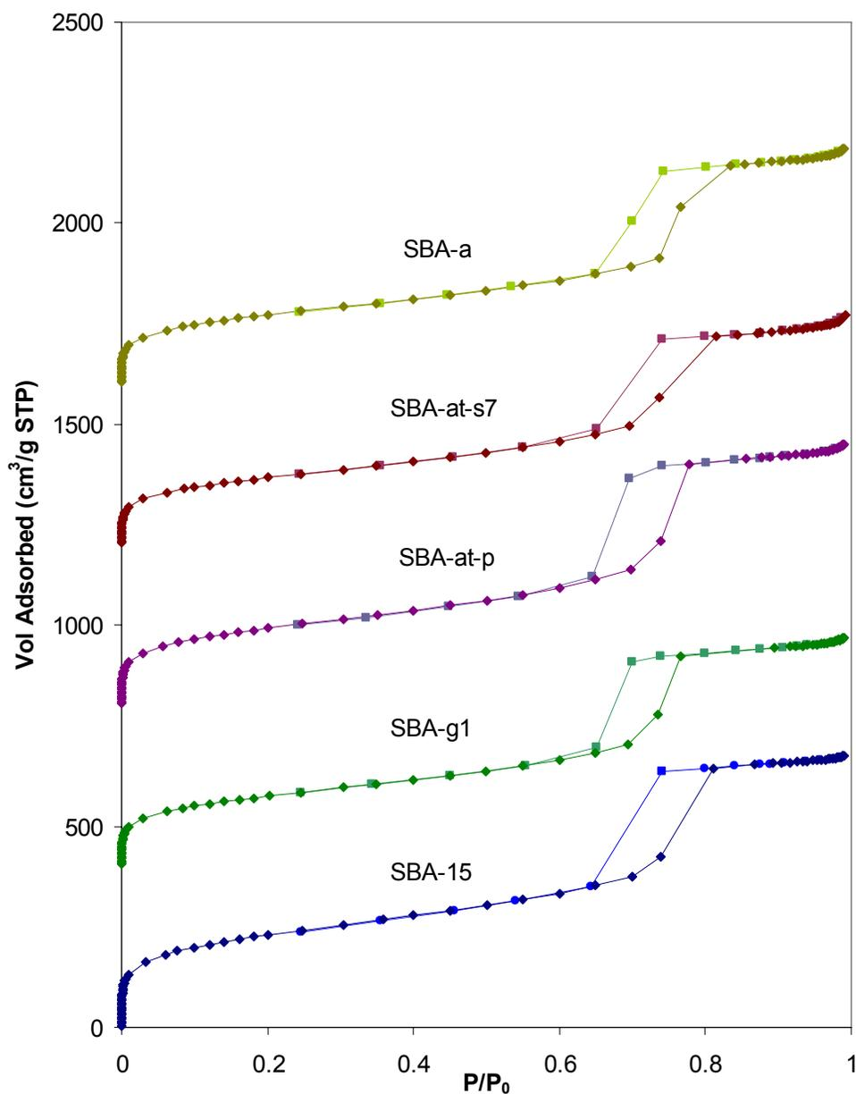
**Figure 2.5.** Nitrogen adsorption/desorption isotherms for various SBA-15 materials. Diamonds correspond to adsorption, squares to desorption. Data have been offset vertically by 400 units for clarity. The organic loading of each functionalized material is  $\sim 0.2$  mmol/g.
