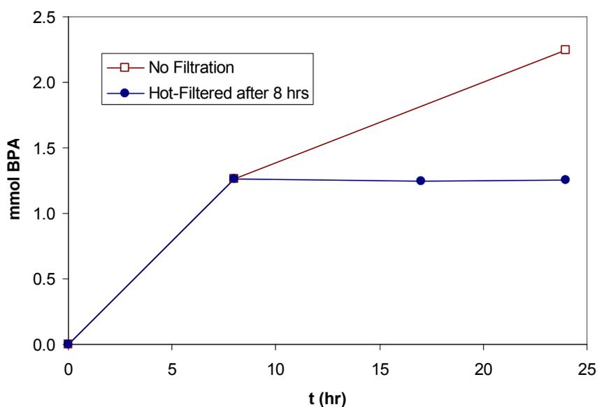
**Figure 2.8.** Hot-filtration test results with **SBA-at-p**. Reaction conditions: 0.02 mmol  $H^+$ , 6 mmol acetone, 24 mmol phenol, 90°C. Catalyst was removed after 8 hours and filtrate was heated at 90°C for another 16 hours.
