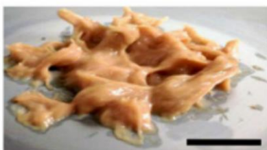
Figure 1.4. Psl overproducing P. aeruginosa ; 10-15 plates of biofilm required (pooled) to perform rheology. Scale bar estimated 3 mm based on other publications by authors specifying tool geometry. Image adapted from [34], open access.
