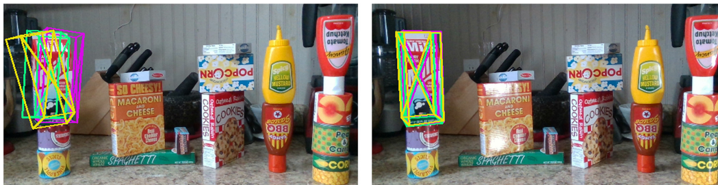
Figure 7.1: Detection results of the milk object of three deep learning models in two images. In the left image, these three models disagree much more than the right image.
