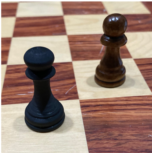
Figure 1.1: Additively manufactured pawn. I designed a pawn (left) to match the style of my chess set (right), and printed it using PR57 black resin.
