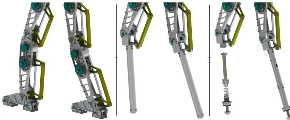
Figure 2.4: The three leg configurations of AMBER-3M: Flat Foot (left), Point Foot (center), and Compliant Point Foot (Right).
