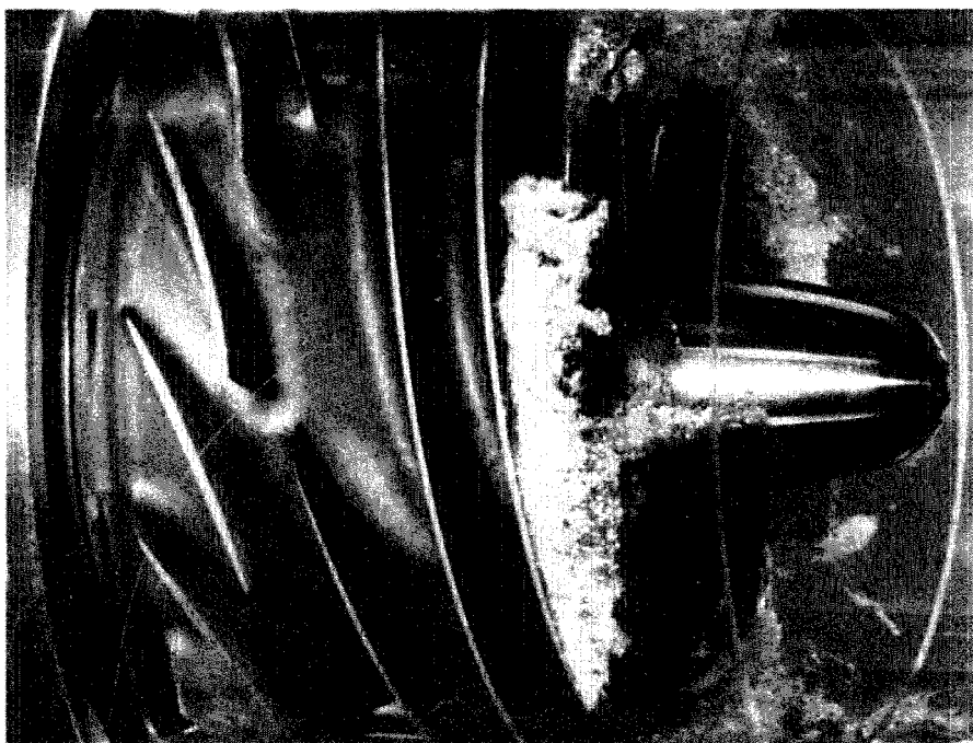
Fig. 3.9 Photographs of Impeller 6 operating at a flow coefficient of 0.070 and at cavitation numbers of 0.087 and 0.061.
