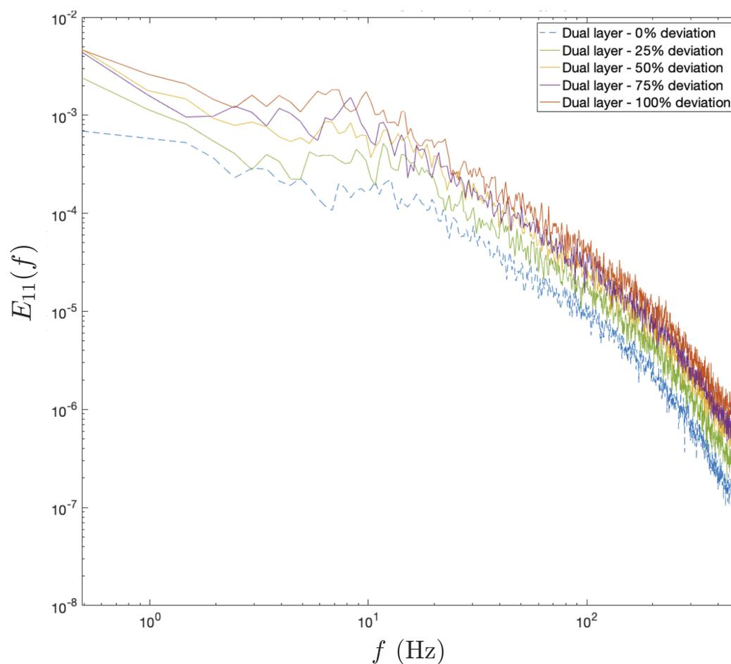
Figure C.4: The energy spectra for the TOD algorithm applied to the backmost layer of a decoupled dual-layer fan array showcases that the increase of the total fluctuation energy is broadly distributed across all relevant scales as the maximum allowed percentage deviation range in the TOD algorithm is consistently increased.
