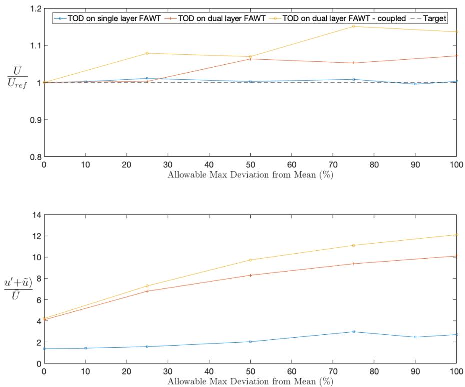
Figure C.2: Comparisons of the TOD algorithm on a single- and dual-layer FAWT.
