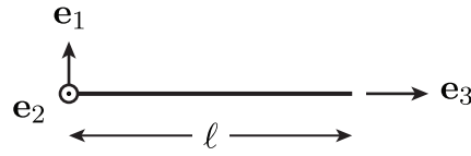
Figure 6.11: Initial (undeformed) configuration of swinging flexible pendulum. The local (material) frame in the initial configuration coincides with the global \{\mathbf{e}_1, \mathbf{e}_2, \mathbf{e}_3\} frame. The gravitational field applied at t = 0 acts in the -\mathbf{e}_1 direction.
