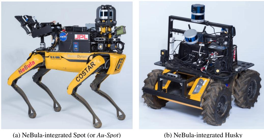
Figure 2.2: Both robots are equipped with custom sensing and computing systems, enabling high levels of autonomy and communication capabilities. The sensing system consists of 3D LiDARs, Intel RealSense cameras, high-intensity LEDs, an IMU, and a thermal camera. The entire autonomy stack runs in real-time on an Intel Core i7 processor with 32 GB of RAM.
