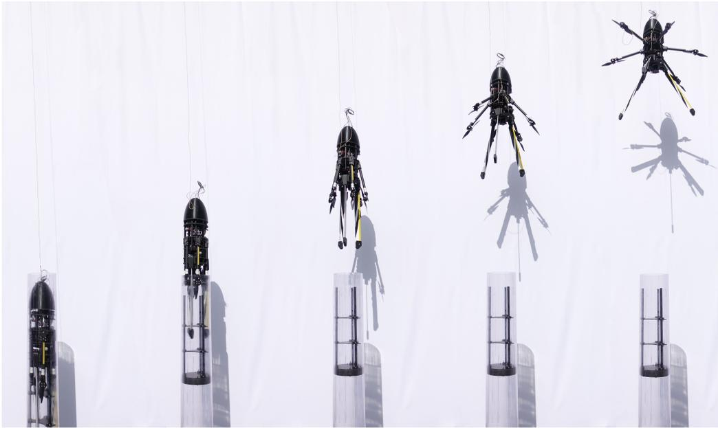
Figure 6.1: Launching *SQUID*: starting from inside the launcher tube, then deploying its arms and fins, before reaching its fully-deployed configuration. Note the slack in the development safety tether and how the carriage assembly remains in the tube throughout launch. Each snapshot is 41 ms apart
