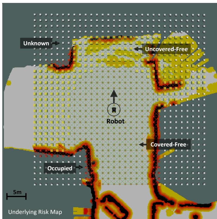
Figure 4.2: Local Information Roadmap (IRM) shown overlaid on the Risk Map. The IRM contains world coverage and traversability risk information. The goal of the coverage planner is to construct paths on the IRM that convert nodes from uncovered traversable (yellow) to covered traversable (brown). By constructing coverage paths in a receding-horizon fashion, the robot extends the boundaries of explored space.
