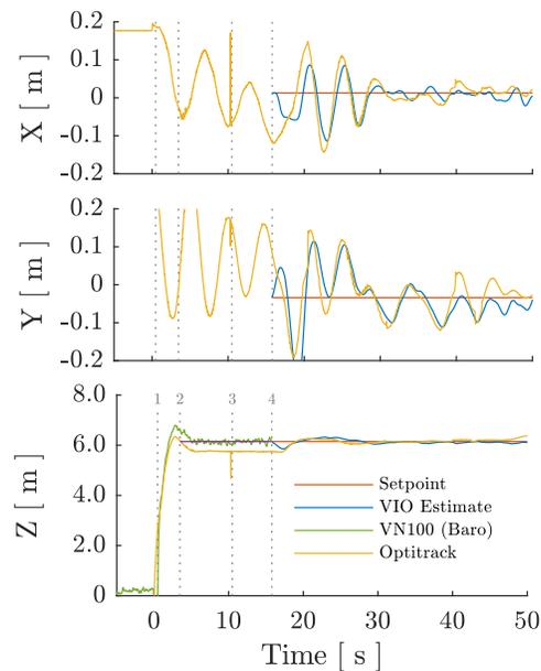
Figure 6.8: Onboard state estimates and ground truth during launch. 1: Motors on, 2: Closed-Loop altitude control, 3: VIO initialization, 4: Position control.
