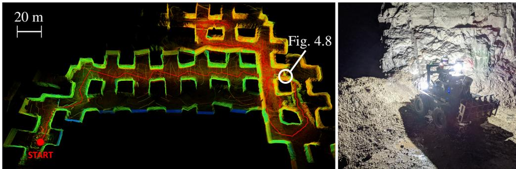
Figure 4.9: Husky’s exploration of a limestone mine during a 60 min. mission using the proposed coverage planner. The coverage paths down the main corridor exhibit a wave-like shape. When the robot encounters a junction, it moves toward the corner in order to maximize coverage of both branches, and then re-aligns with the centerline of the main corridor. The starting location of snapshot Fig. 4.8 (a) is indicated on the map. Fig. 5.8 (b) provides the associated coverage plot.
