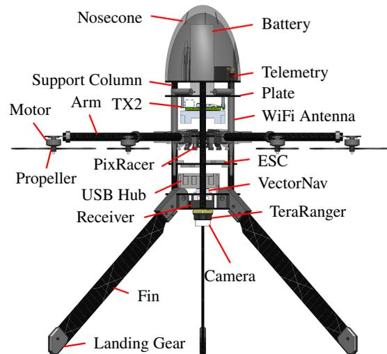
Figure 6.2: An annotated schematic of *SQUID*.
