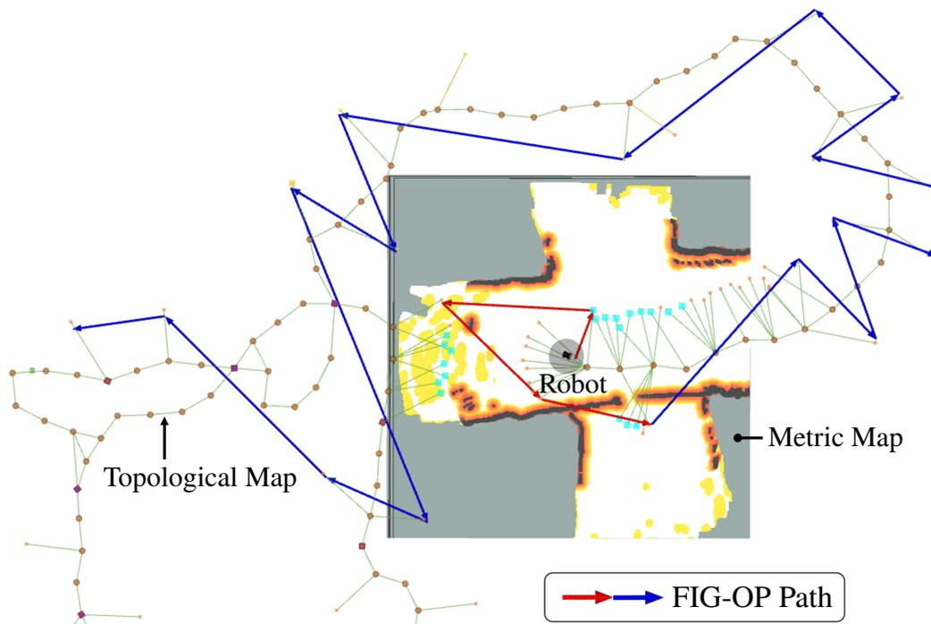
Figure 5.1: FIG-OP path generated during the autonomous exploration of the limestone mine of the Kentucky Underground, Nicholasville, KY, with a Husky robot platform. The environment representation is broken down into two levels: a dense robot-centered local metric map, and a sparse globally-spanning topological map. Arrows show the FIG-OP solution. Path costs are computed on either the metric (red arrow) or topological map (blue arrow).
