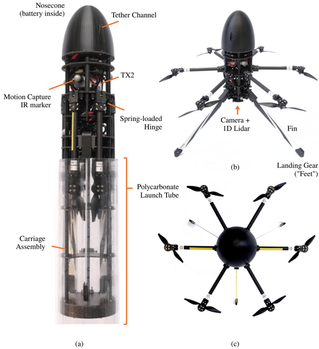
Figure 6.3: *SQUID* partially inside the launcher tube and interfacing with the carriage (a), and with its arms and fins fully deployed from a side (b) and top perspective (c).
