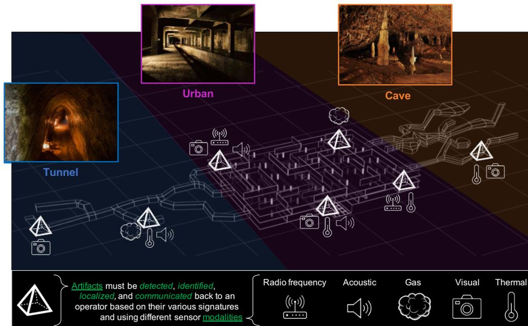
Figure 2.1: The Final Circuit of the DARPA SubT Challenge consists of elements from all subdomains (i.e., tunnel, urban, cave). To demonstrate efficient exploration of the environment, competitors score points by accurately reporting the type and location of artifacts distributed along the course. [4]
