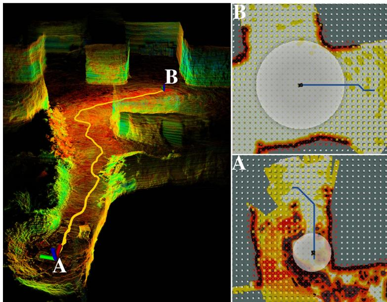
Figure 4.1: Adaptive coverage range (translucent circle) and coverage path from single planning episode (blue) in a locally confined (A) and spacious area (B) during Husky’s autonomous exploration of a limestone mine in Nicholasville, KY. The robot’s trajectory (yellow) is overlaid on pointcloud (left figure).
