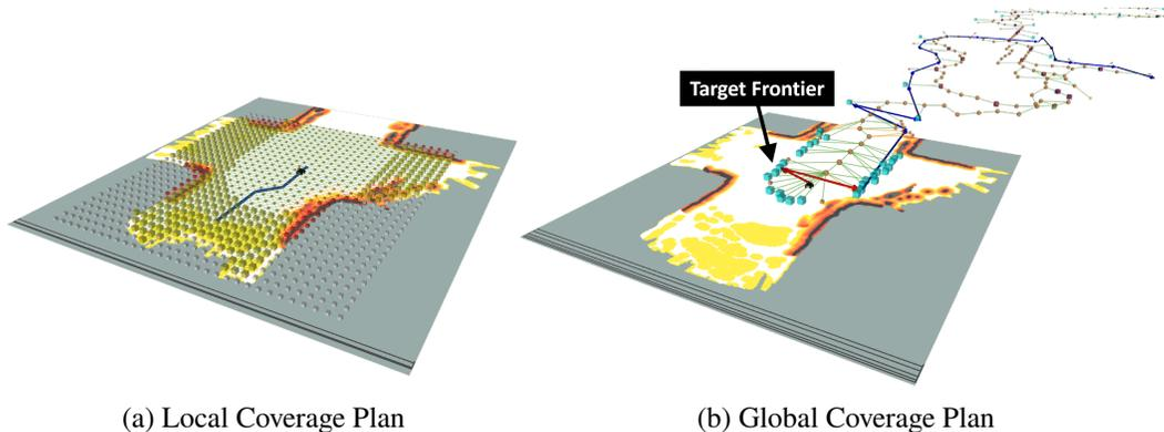
Figure 3.5: Illustration of local-global coverage planner coordination. Simultaneously constructed local (a) and global (b) coverage plans during Husky’s exploration of a limestone mine are shown. Since the target frontier associated with the GCP policy is inside the bounds of the Local IRM, LCP maintains control guides the robot. The local and global policies shown are developed in Chaps. 4 and 5, respectively.
