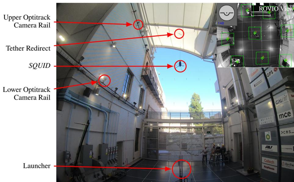
Figure 6.6: Launching *SQUID* in 42 foot-tall flying arena. The arena has two tiers of motion capture cameras.
