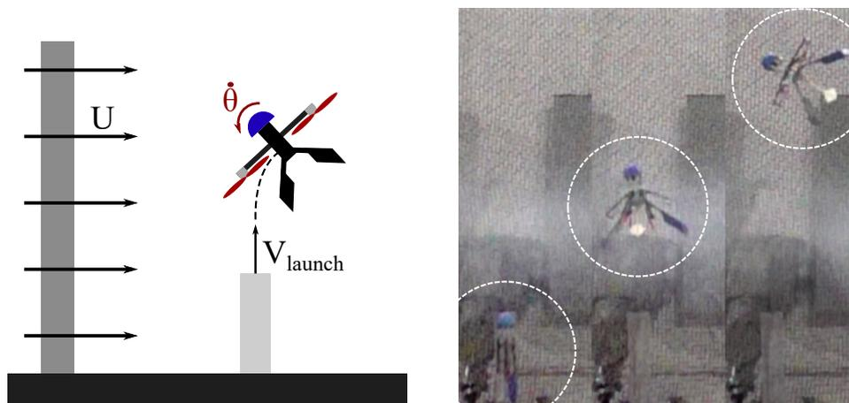
Figure 6.5: Wind Tunnel Testing. Left: definition of experiment parameters. Right: snapshot sequence showing stable upwind pitching of the 1/3 *SQUID* model.
