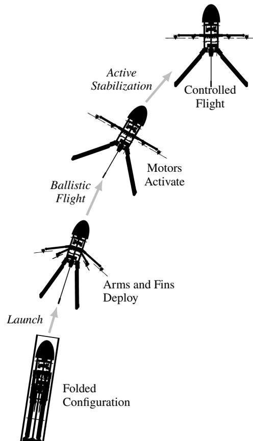
Figure 6.4: *SQUID* deployment sequence.
