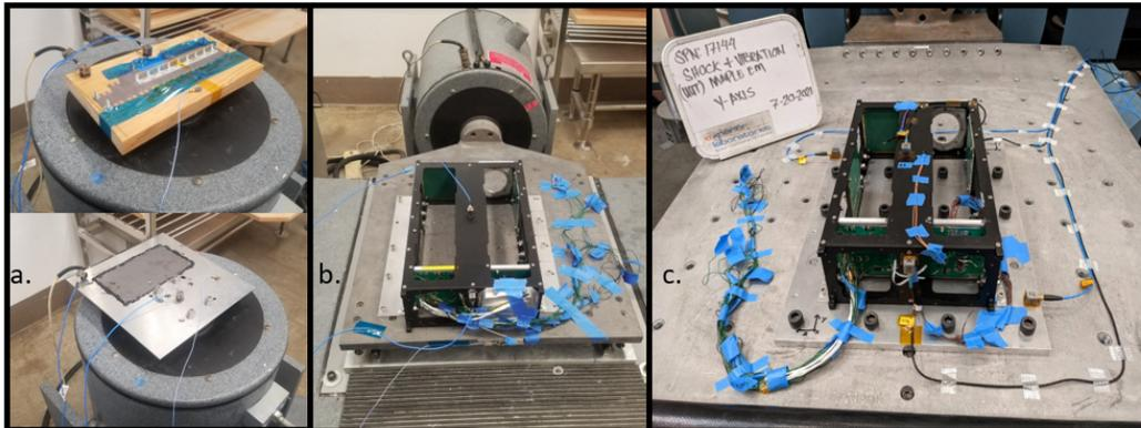
Figure A.9: (a) Component level mechanical testing at Caltech. (b) Preliminary EM mechanical testing at Caltech. (c) EM mechanical testing at Experior Labs.
