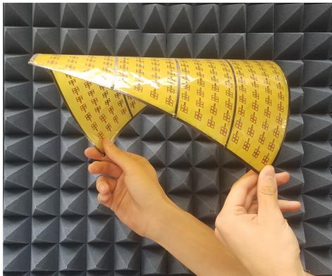
Figure 4.23: A 2D flexible phased array antenna sheet with 256 10 GHz patch antennas.
