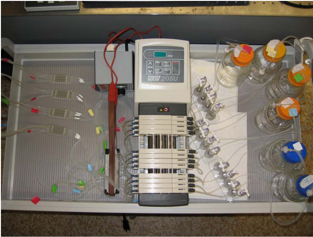
Figure A3 Photograph of the flow apparatus. The entire interior was kept sterile, and flow chambers were maintained at 30°C in an incubator (not shown).
