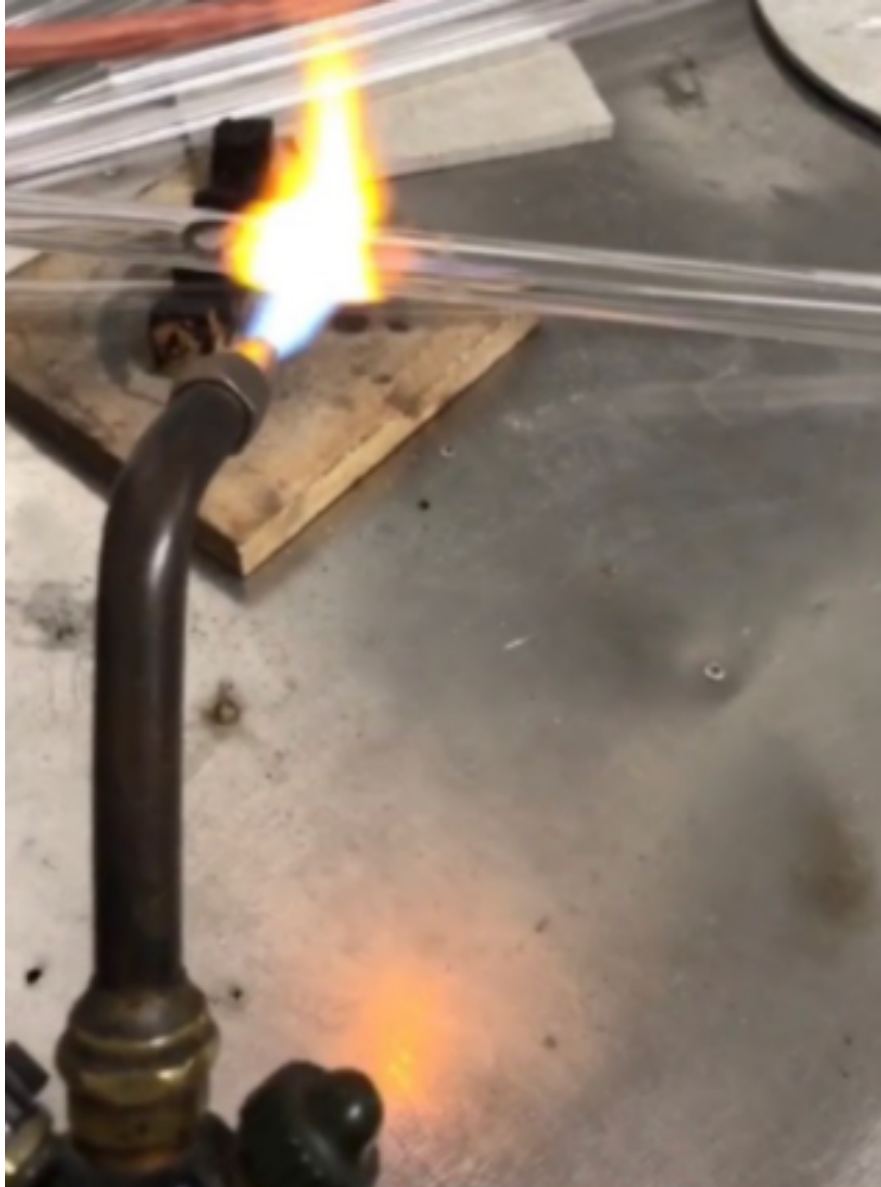
Figure 4.1: An image of the glassblowing torch used to seal the quartz ampules.
