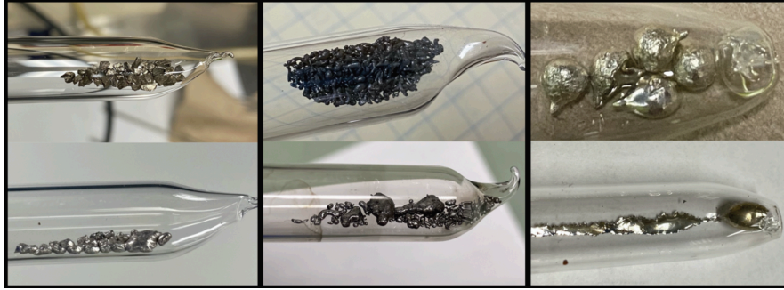
Figure 1.2: Bi, Pb, and Sn sealed in evacuated quartz ampules before (top) and after (bottom) melting in preparation for neutron scattering at ARCS. In this thesis we will primarily be analyzing neutron scattering done on Ge in a similar ampule.
