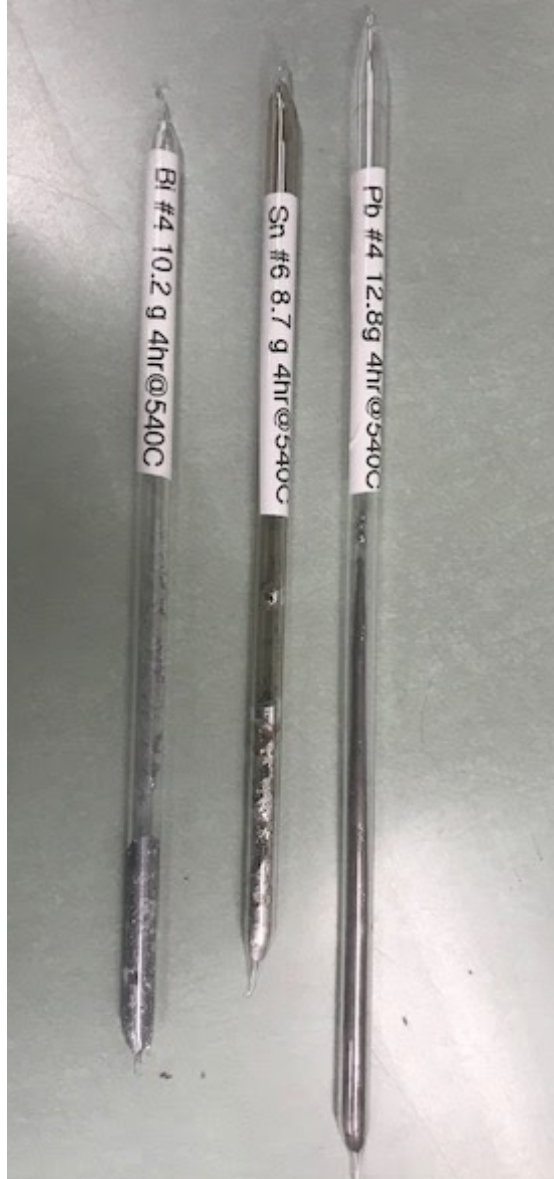
Figure 4.2: An image of some of the melted samples demonstrating containment.
