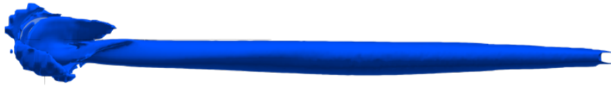
Figure 5.9: Streamwise vorticity isosurface ( \omega_x = 1 ) for the mean flow at Re = 500 and \alpha = 25^\circ for \lambda = 2 .
