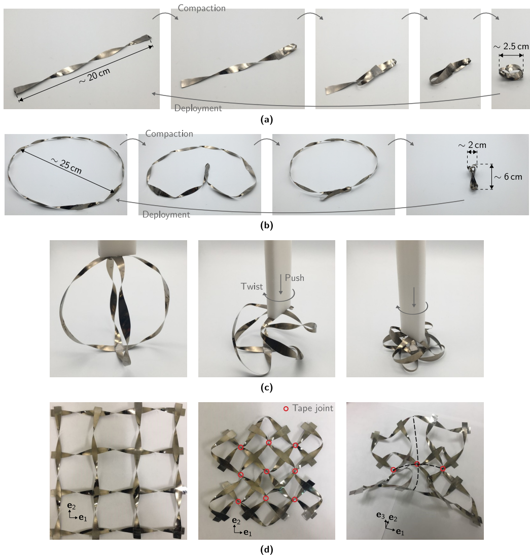
Figure 2.10: Elastic stowage and deployment of twisted ribbons. In all cases, deformations are reversible and do not induce any plastic deformation. Note that we use tape to keep together the stowed configurations for illustration purposes. (a) A twisted ribbon can be compacted by folding it about the necks/hinges, and by finally bending the wide faces. (b) Assembling four ribbons in a circle leads to a ring structure that can be compacted following the same procedure shown in (a). (c) The chirality of the ribbons can be leveraged to create a sphere that can be compacted by applying a twisting load, similarly to Hoberman’s Twist-O. (d) Planar auxetic lattice made of twisted ribbons. The dashed lines highlight the global curvature achievable by taping together selected pairs of necks.
