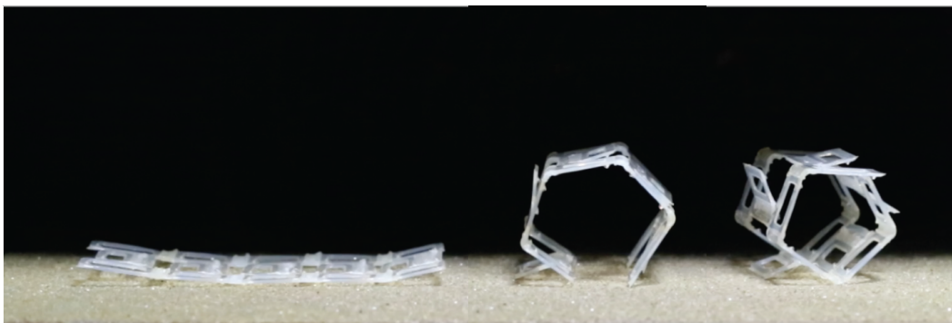
Figure 1.2: A time-lapse overlay showing untethered shape-reconfiguration and locomotion by a programmed structured medium. The mesogen orientation in the liquid crystal elastomer bilayers cause the hinges to fold in response to a thermal stimulus [15].
