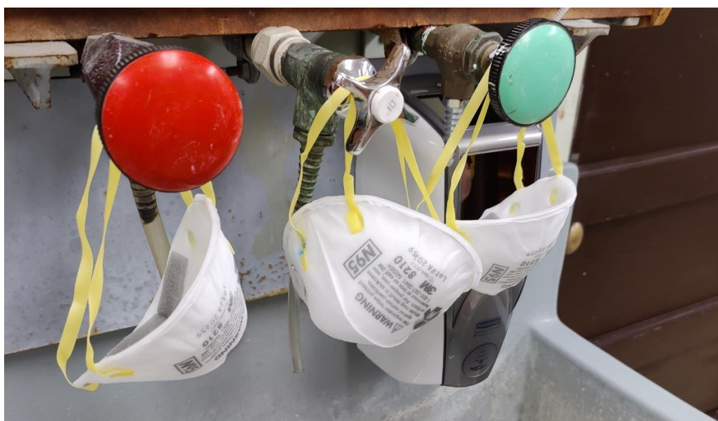
Figure 5.1. Three 3M 8210 N95 respirators air drying after liquid treatment.
