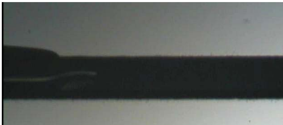
C: top view on 200 \mu m wide nanowick
