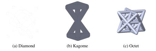
Figure 1.1: Computer aided drawings (CAD) of the unit cells used throughout this dissertation shown in various renderings.
