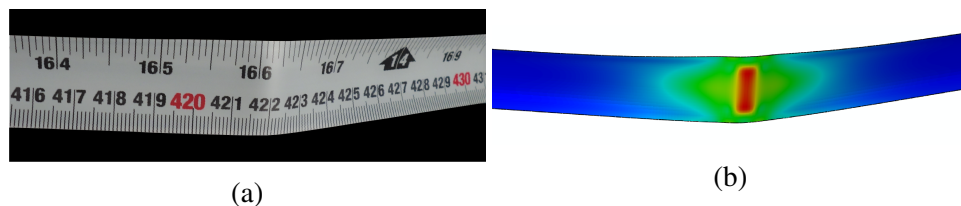
Figure 3.13: Tape spring deformed shape obtained for the opposite sense bending test. (a) Experimental deformed shape and (b) finite element deformed shape. The color map corresponds to the distribution of the Von Mises stress, but it is used here solely for visualization purposes.
