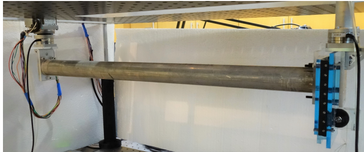
Figure 3.5: Stiff tube mounted on the bending machine. This test sample is used to determine the torsional stiffness of both sliders.
