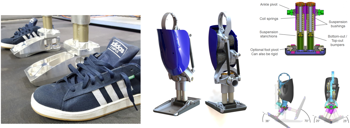
Figure 4.3: Final ankle design which was used on DURUS. In particular, two passive springs in the ankle were utilized below a two degree of actuation ankle. The result is compliant interaction between the robot and the ground with rigidly controlled linkages above.
