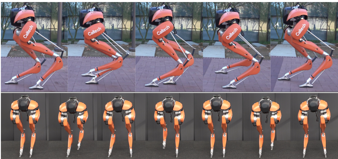
Figure 8.19: Gait tiles for Cassie walking with an ID-CLF-QP controller on a sidewalk at Caltech, and for lateral strafing indoors.
