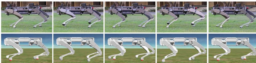
Figure 4.19: Top: Snapshots showing a two full steps of the walking gait on an outdoor lawn. Bottom: Running gait in the RaiSim simulation environment.
