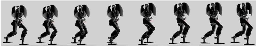
Figure 3.4: Snapshots of the DURUS running at 2.0 m/s.
