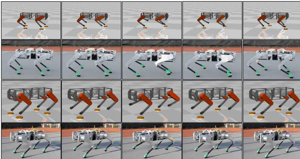
Figure 4.11: Comparison between MuJoCo simulation (animated) and experiments. The upper two are for stepping in place, gait4; the lower two are logged for a full step of the ambling gait.
