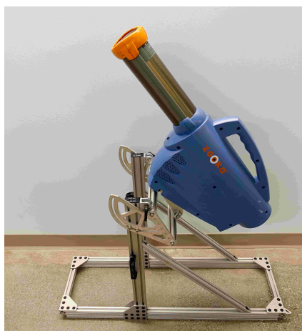
Figure 3.3: The pneumatic baseball pitching machine used to launch the SQUID 3" prototype.
