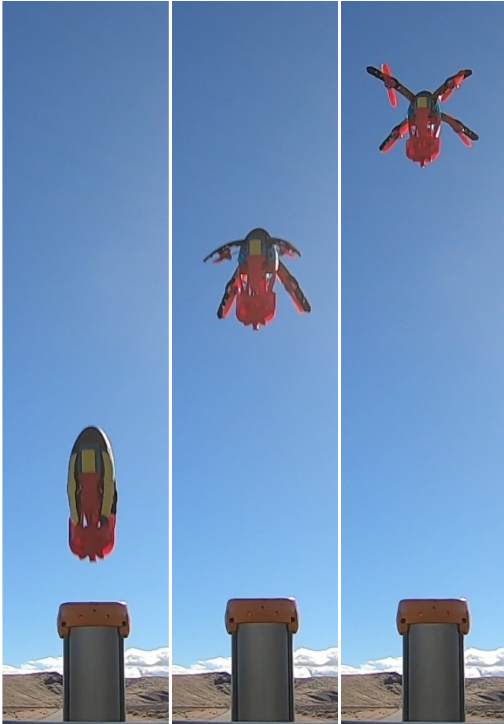
Figure 3.1: The SQUID 3'' prototype in both ballistic (left), deploying its arms (center) and multirotor (right) configurations during flight. Selected frames during a launch from a moving vehicle at 50mph (22 m/s). After deployment the drone hovered around the area.
