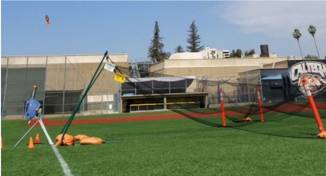
Figure 3.8: Picture of the field testing setup deployed on a Caltech sports field, with a net to protect the SQUID 3 '' prototype from crashes
