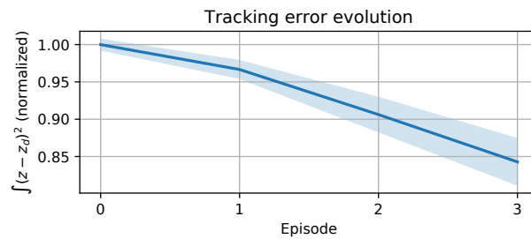
Figure 5.4: Mean \pm 1 standard deviation of tracking performance after each episode over 5 independent campaigns.
