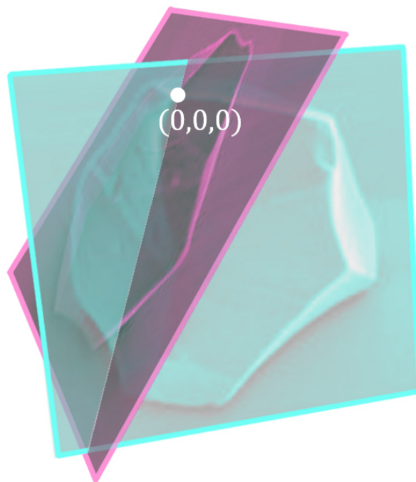
Figure B.1: Defining a reference point based on 2D images of the same particle.
