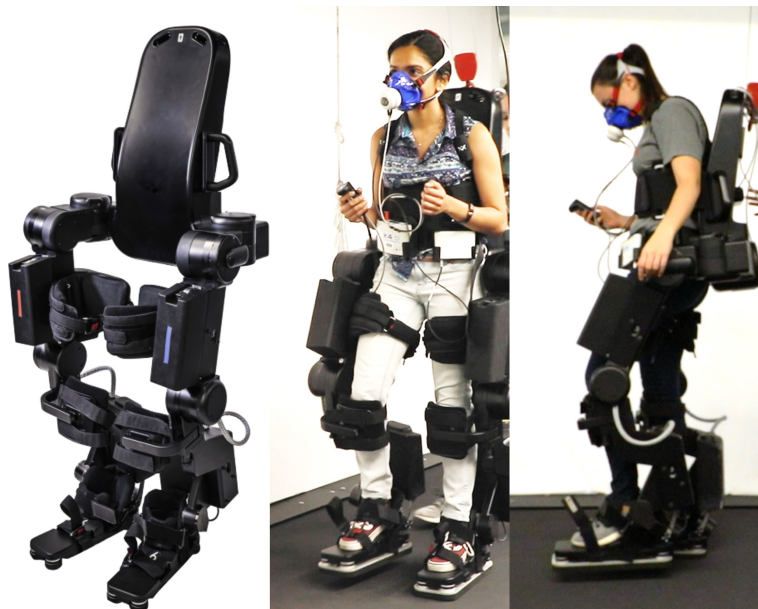
Figure 5.1: Atalante Exoskeleton with and without a user. The user is wearing a mask to measure metabolic expenditure.
