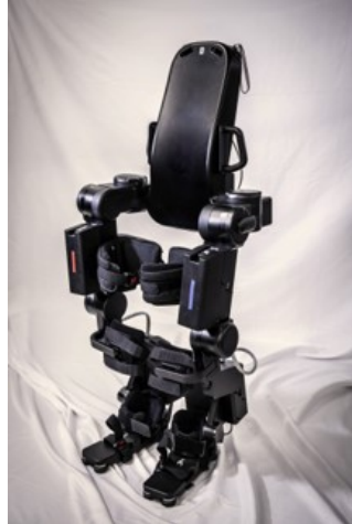
Figure 1.1: The Atalante exoskeleton, designed by Wandercraft (Wandercraft, n.d.).
