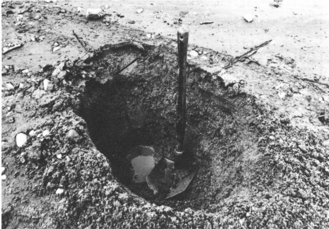
(b) Recovered scour-cord (arrow), straightened to vertical position.
