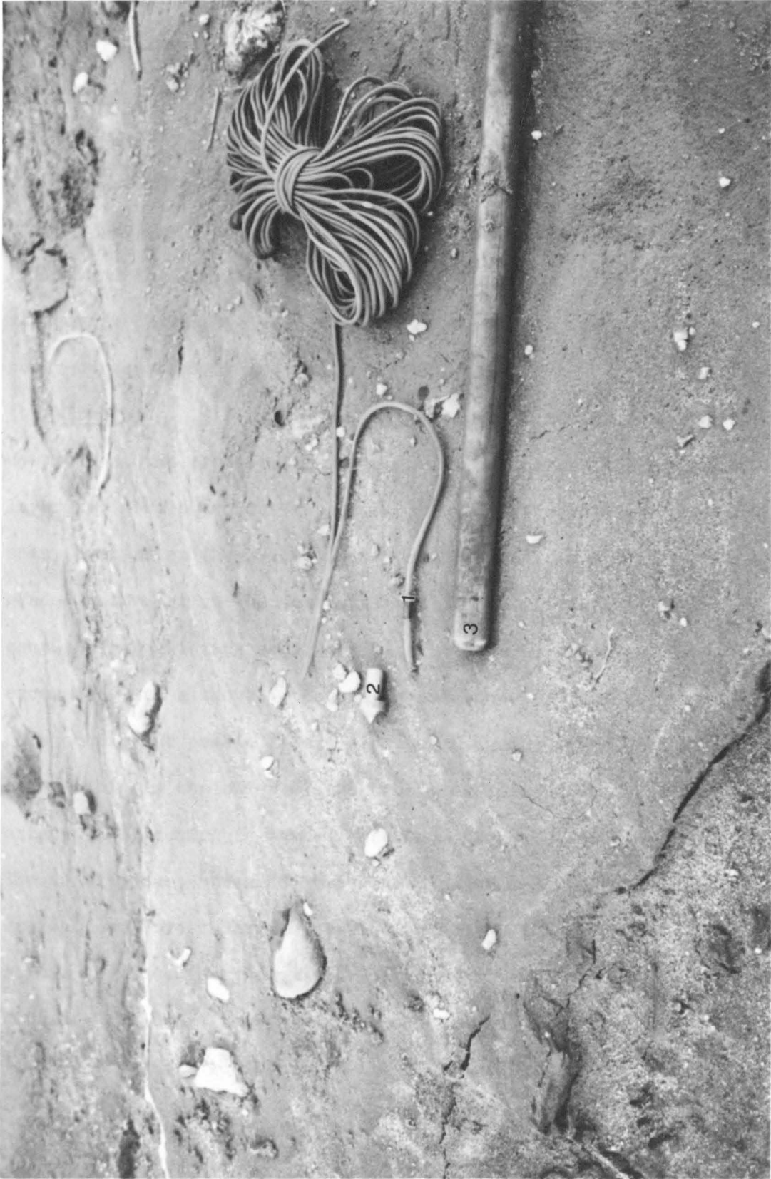
Figure 2-5. Scour-cord with lock-screw (1), penetrator-anchor (2), and driving tube (3).
