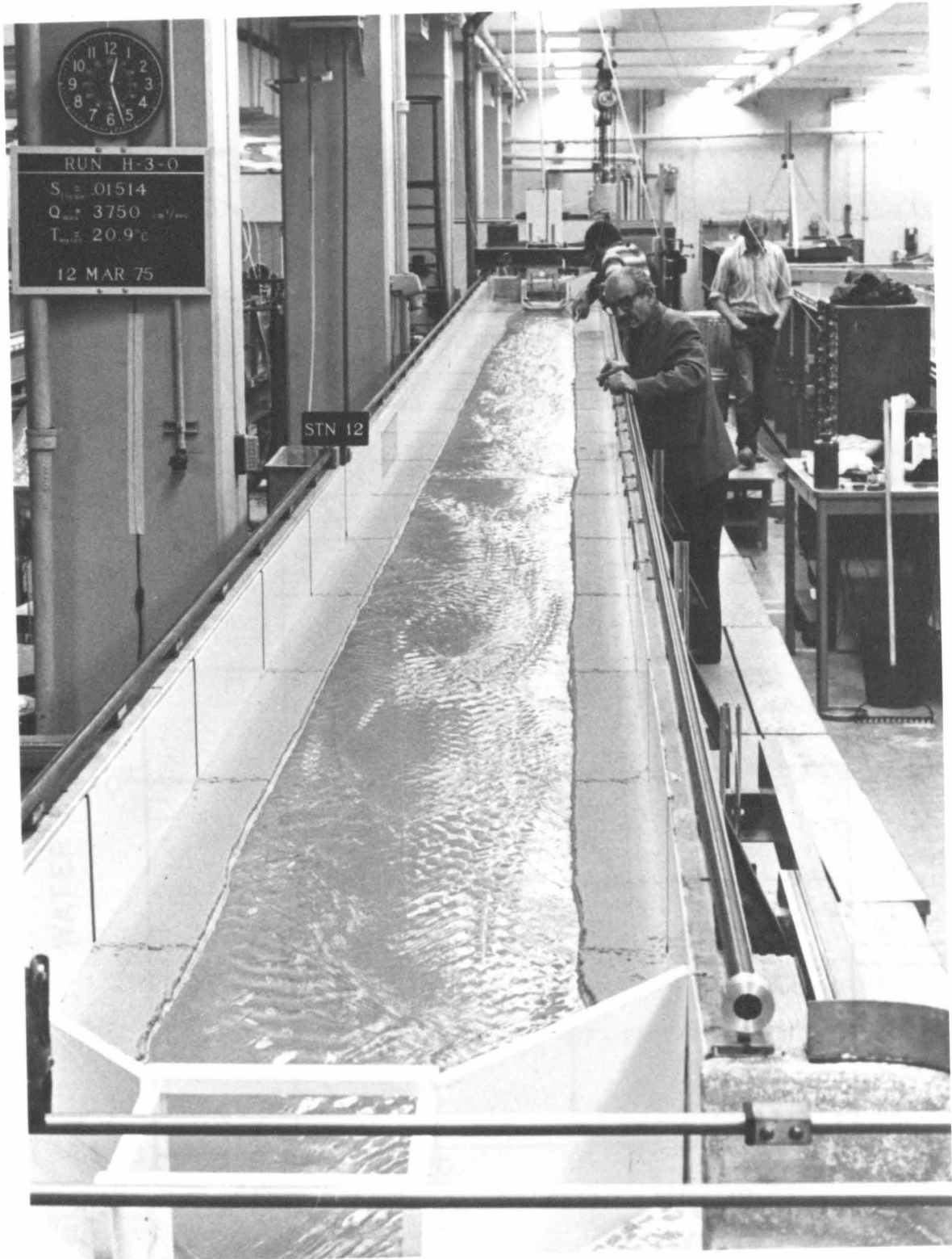
Figure 6-9. Typical channel bore in alluvial-bank experiment.
