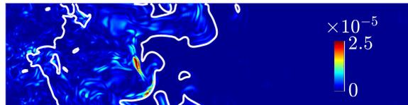
Figure 3.13: Two-dimensional slice showing isocontours of  $\epsilon$  for the turbulent case ( $\Delta t = 10^{-8}$  s). Two temperature isolines are superimposed in white ( $T = 1000$  K and  $T = 1900$  K).
