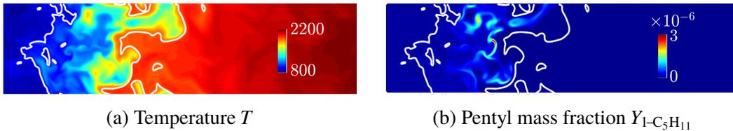
(a) Temperature  $T$ (b) Pentyl mass fraction  $Y_{1-C_5H_{11}}$ Figure 3.11: Two-dimensional slices showing isocontours for the turbulent case ( $\Delta t = 10^{-8}$  s). Two temperature isolines are superimposed in white ( $T = 1000$  K and  $T = 1900$  K).
