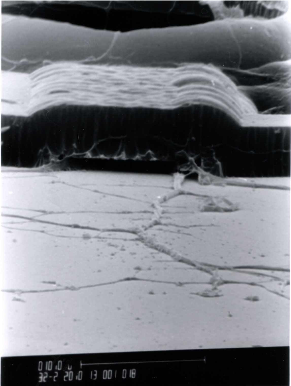
Figure 4.2: A neural process emerging from a neurocage tunnel. The origin of the neurite is the trapped neuron on the interior of the cage. Note that there are many thin processes branching off from the main process. Under Nomarski optics, only the thickest processes are visible; numerous thin processes are not. Scale bar: 10 \mu\text{m}
