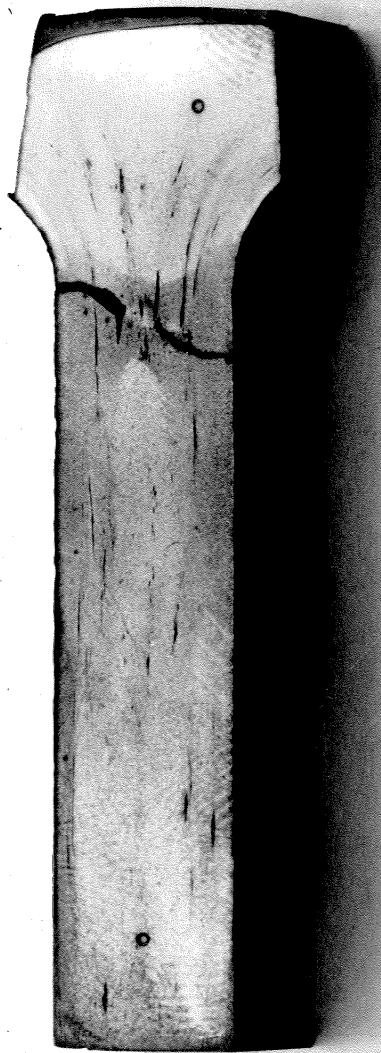
FIG. 5.7 ETCHED END SECTION SHOWING AREAS OF MASSIVE YIELDING
