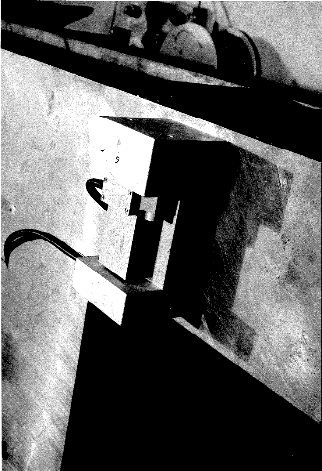
FIG. 4.1 ACCELEROMETER MOUNTED IN A MILLED STEEL BLOCK
