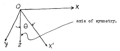
Consider when state of stress in body is due to a stress  $x^{\dagger}x^{\dagger}$  in the direction ox!. Take oy! and oz! to form an orthogonal set of axes with ox!.
