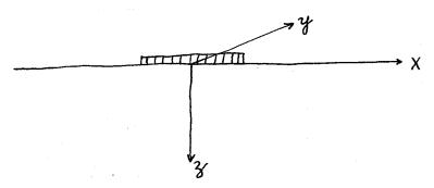
For simplicity, consider a loading symmetrical about o y, and extend in either direction from 0 a considerable distance along the y axis, say from  $y = \ell$  to  $y = -\ell$ . At regions, not close to  $y = \ell$  the state of strain is approximately plane: i.e.
