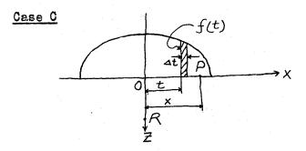
The deflection at any point P due to the elemental loading  $f(t) \triangle t$  at the point t is, on using (2.50), given by
