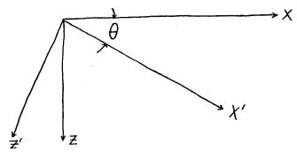
Consider a two dimensional medium, with the orthogonal pair of axes ox', oz' making an angle  $\theta$  with ox and oz respectively.
