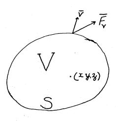
Consider the motion of the material within a closed surface S enclosing a volume V surrounding a point (x, y, z) in the strained medium.
