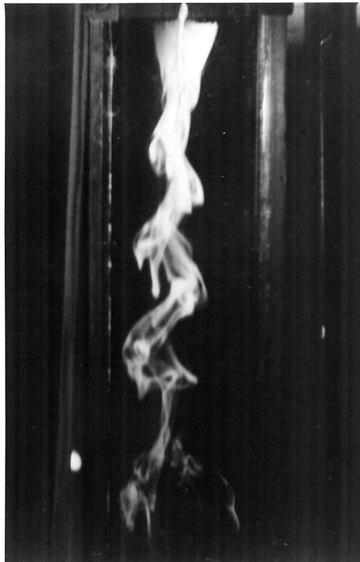
Photo No. D, 8. -Elliptic plate (major axis=32 mm; minor axis=4 mm; ratio of the axes = 1/8 ), looking at it in the direction of the minor axis. Velocity: 20.6 cms/sec. R.N.=496
