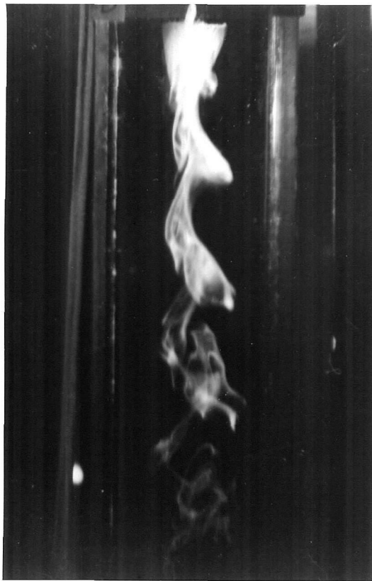
Photo No. D,8. - Elliptic plate (major axis=32 mms; minor axis=4 mms; ratio of the axes=1/8), looking at it in the direction of the minor axis. Velocity: 20.6 cms/sec. R.N.=496
