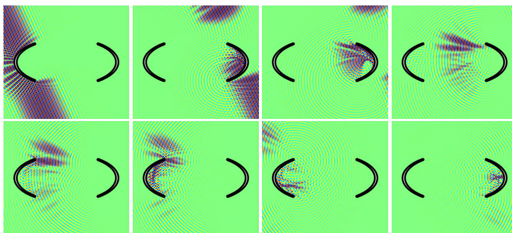
Figure 2.6: Total fields in the “Whispering Gallery” experiment mentioned in the text. Note the multiple reflections that take place at the elliptical surfaces which, over long propagation times, give rise to a significant number of scattering events. The time sequence starts left-to-right on the first row, and then continues left-to-right on the second row.
