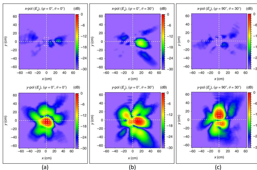
Figure 3.76: Broadside array fields recorded in 2-D [84].
