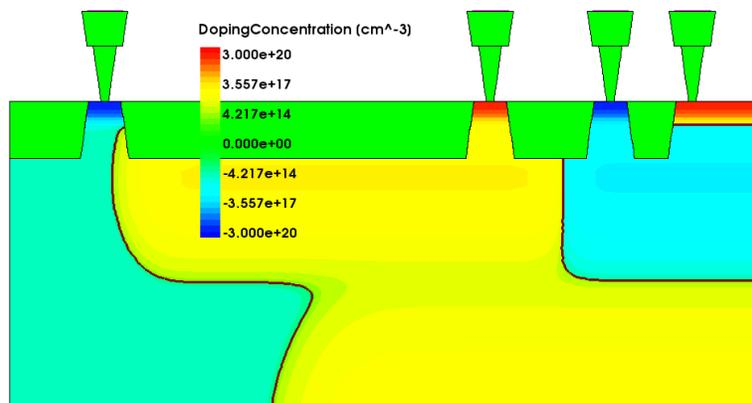
Figure 4.7: A cross section of doping concentrations for PD design (Fig. courtesy of C. Ives).
