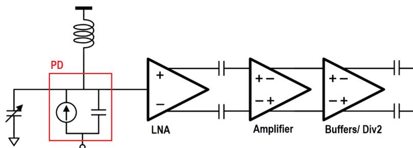
Figure 4.10: Input chain schematics (Fig. courtesy of C. Ives)
