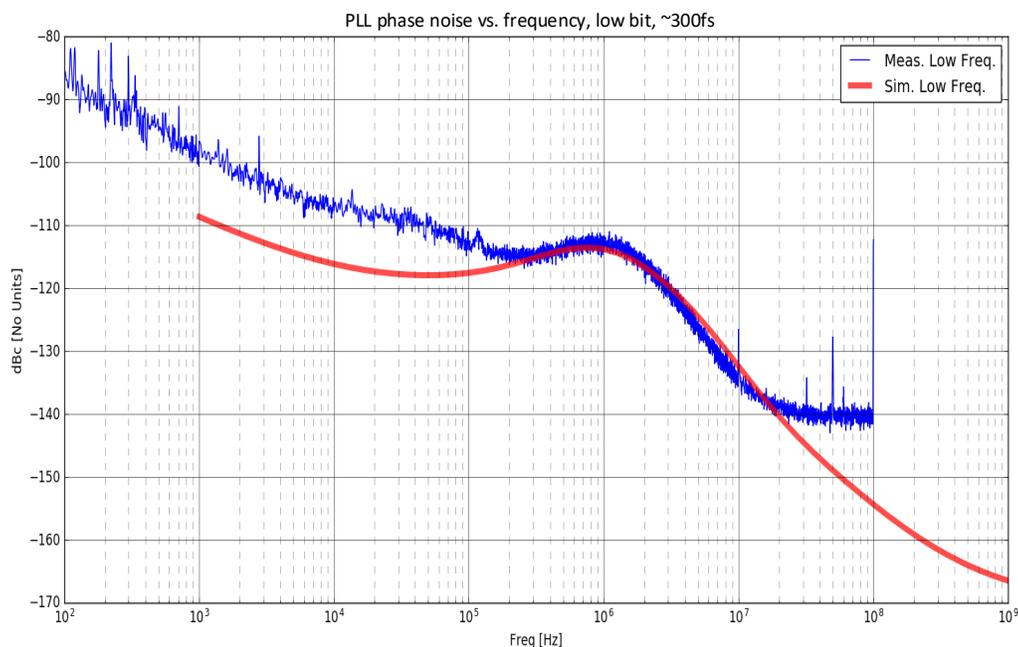
Figure 3.48: PLL phase noise PSD measurement vs. simulation
