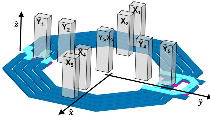
Figure 2.22: Probe locations for gain profile characterization.
