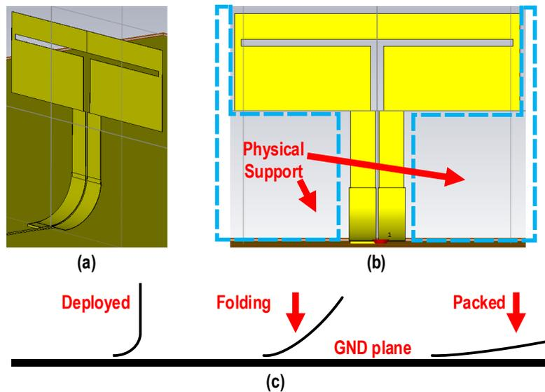
Figure 3.68: Vertical sheet antenna concept.
