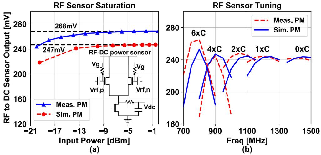
Figure 2.20: Measurement vs. simulation of (a) input power saturation, and of (b) input matching.
