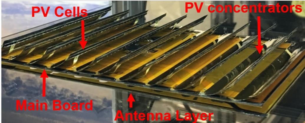
Figure 3.14: A photo of an SSP tile prototype.
