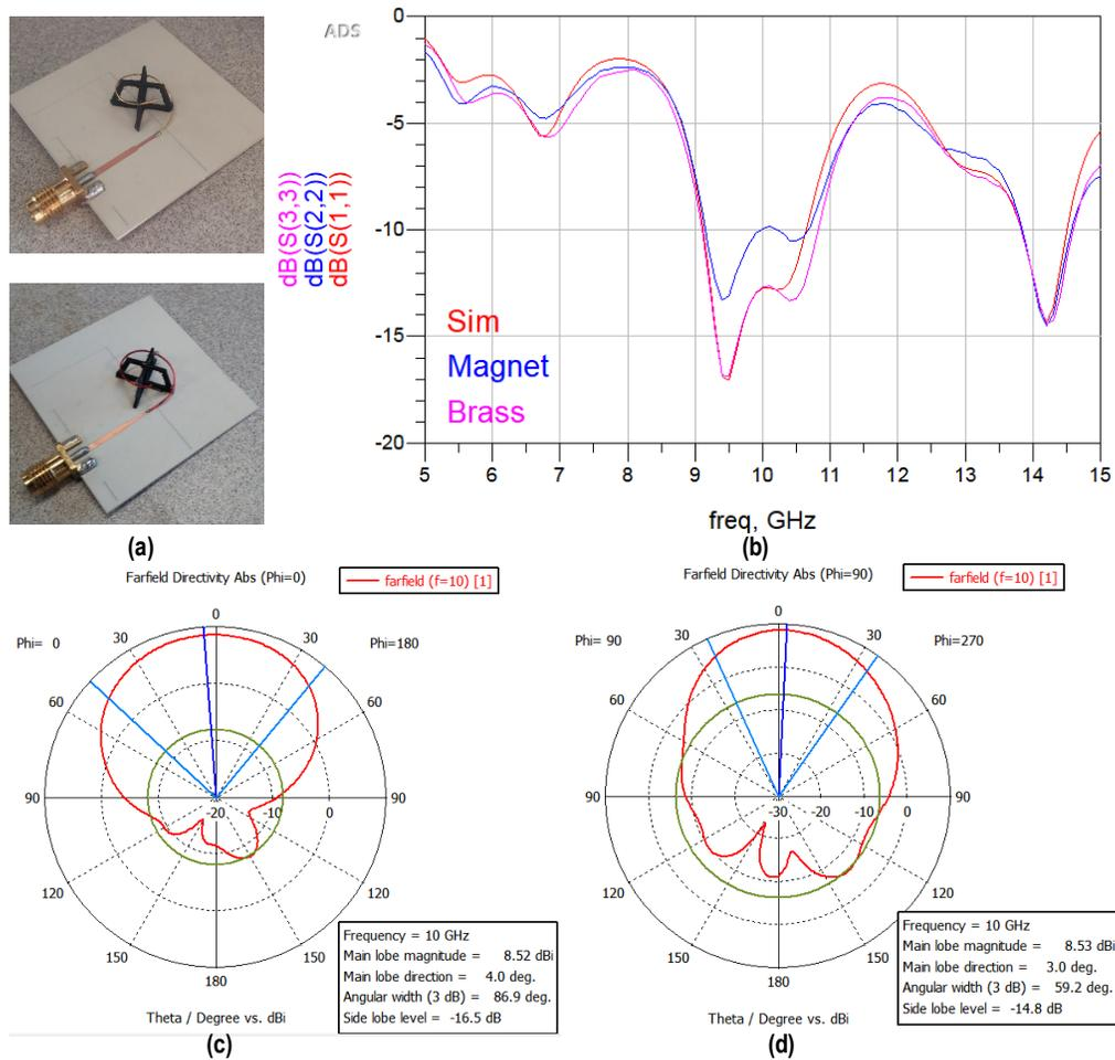
Figure 3.71: Collapsible spring antenna (a) test structure (the plastic support should be removed or changed in the final design), (b) input matching, (c) antenna pattern 0°, (d) antenna pattern 90°.
