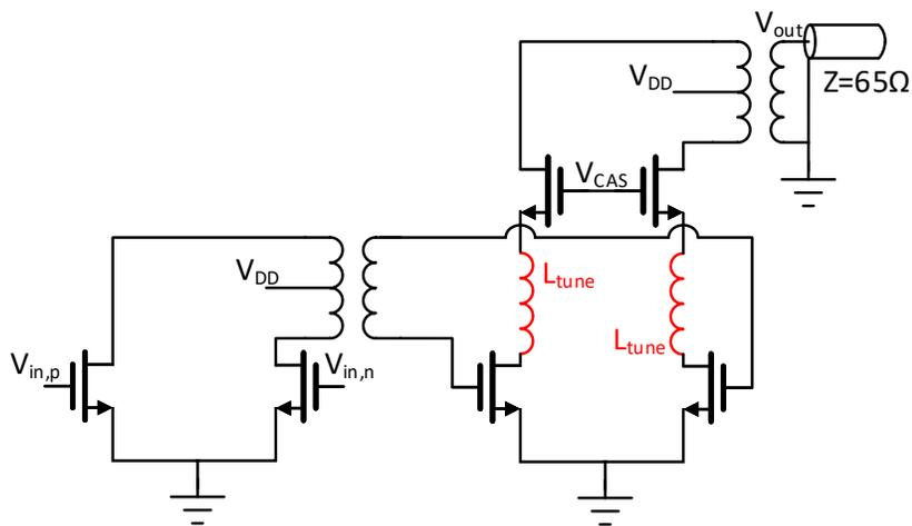
Figure 4.21: Power amplifier output schematic.
