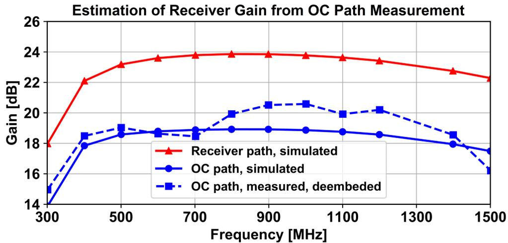
Figure 2.21: Comparison between the simulated and measured OC path gain to the simulated receiver gain.
