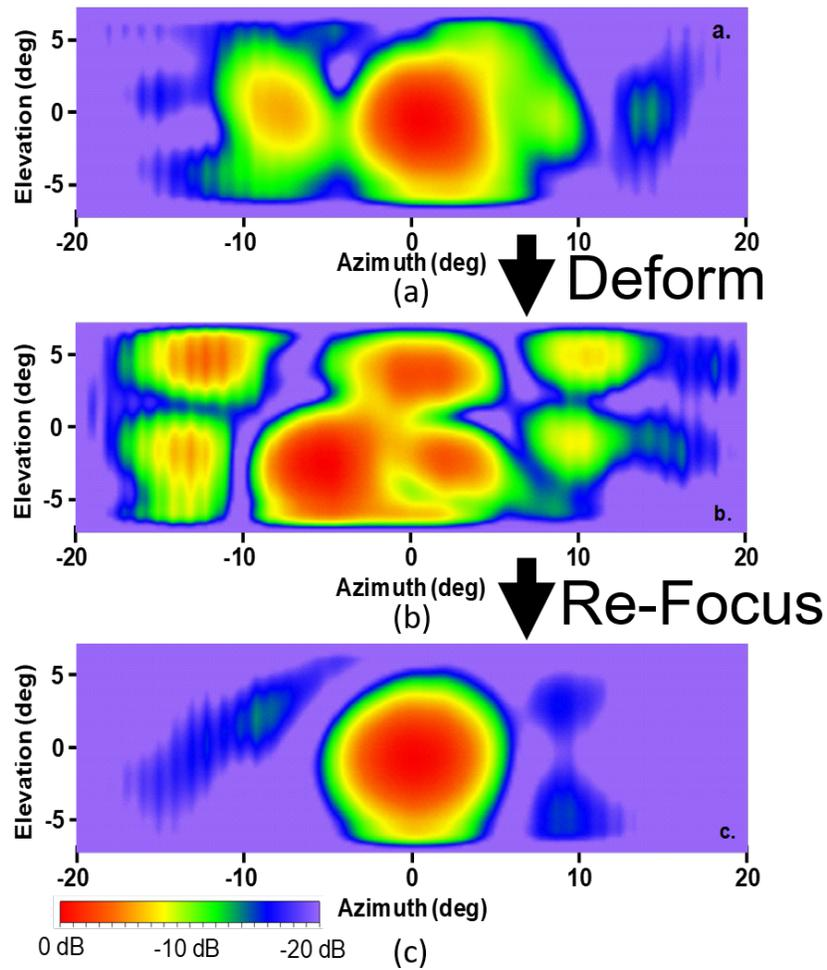
Figure 3.92: Deformation correction. (a) Focusing, (b) deformation, and (c) re-focusing of a deformed flexible phased array transmitter.
