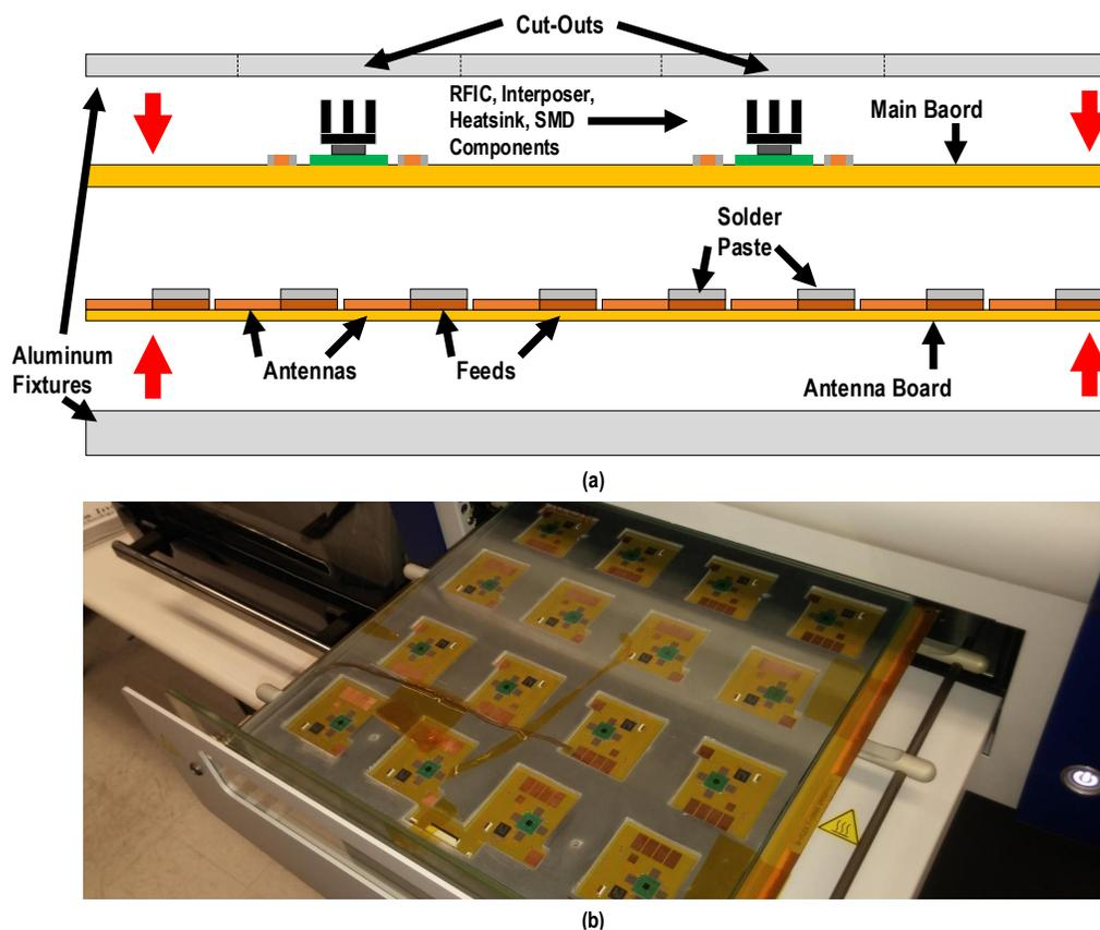
Figure 3.86: Antenna sheet assembly. (a) Schematic description and (b) a demonstration of the assembly process.
