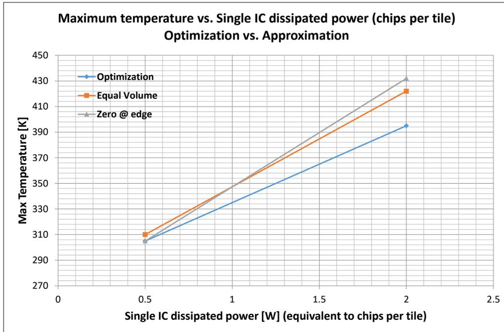
Figure 3.19: Expected temperature as a function of power per chip, all ground leveling schemes.
