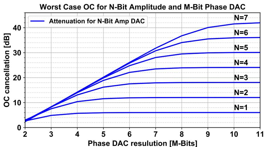
Figure 2.18: Attainable offset cancellation as a function of amplitude and phase control number of DAC bits.
