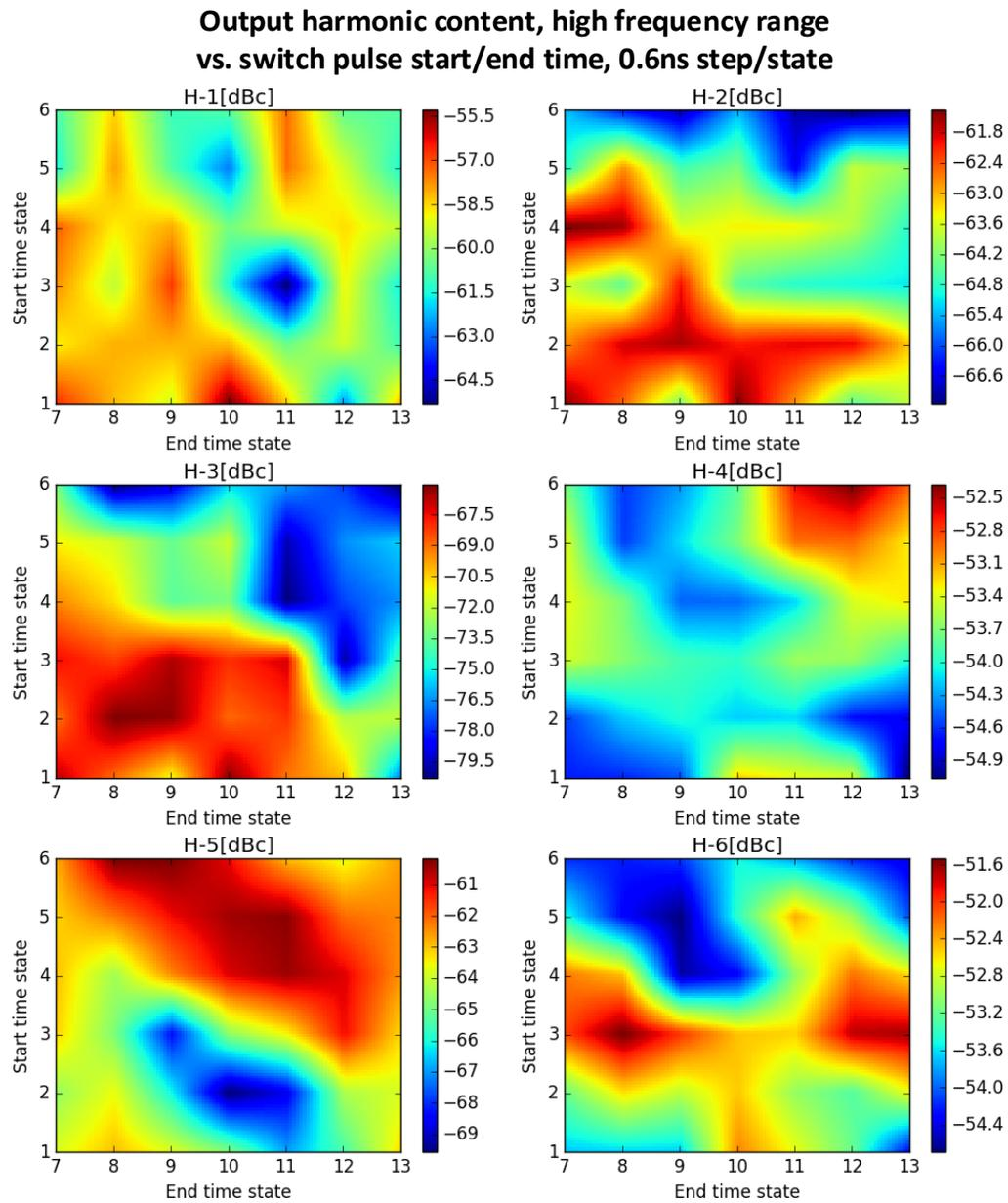
Figure 3.47: PLL reference spur levels for different digital settings of start/stop times of the pulse.
