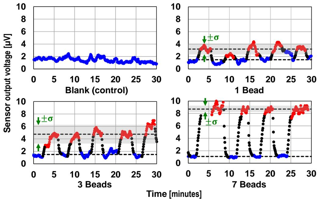
Figure 2.25: Exemplary system response to different amounts of  $4.5\mu\text{m}$  iron-oxide beads.
