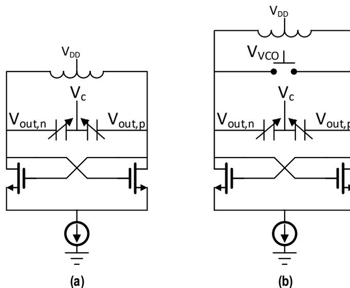
Figure 4.15: VCO and ILFD schematics.
