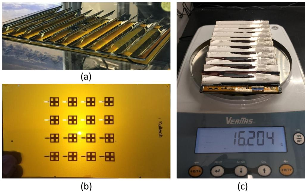
Figure 3.81: Integrated RF-PV tile. (a) Completed demonstration board, (b) antenna sheet, and (c) weight of the assembled board.
