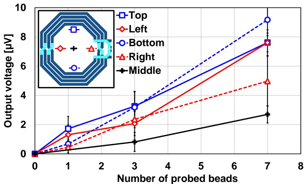
Figure 2.26: Sensor cell response for  $4.5\mu\text{m}$  beads at various locations on the core surface.
