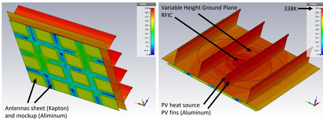
Figure 3.21: Estimated temperature of tile with PV and RFIC heat sources in space.
