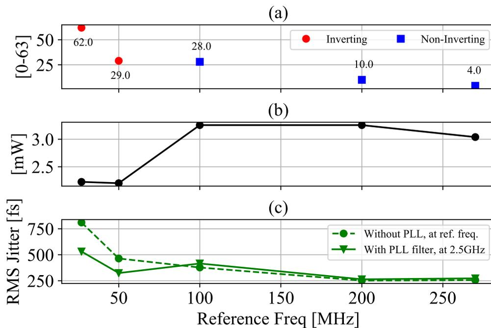
Figure 3.53: Performance vs. frequency. (a) Participating DCDL cell count, (b) power consumption of participating DLL blocks, and (c) rms jitter within the 1kHz - 10MHz band.
