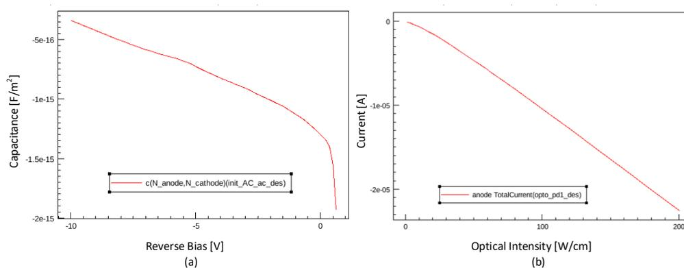
Figure 4.8: Photodiode (a) capacitance density and (a) responsivity simulations (Figs. courtesy of C. Ives).
