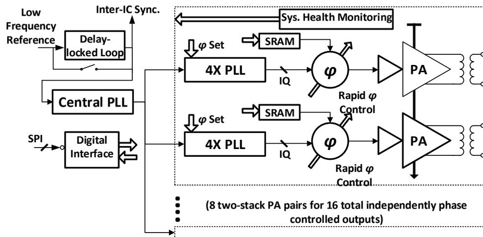
Figure 3.31: Block diagram of an RFIC with two output PAs stacked from a DC perspective [74].
