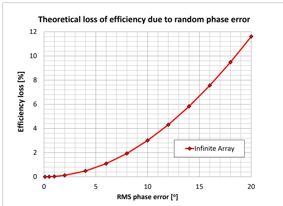
Figure 3.37: Phased array loss of efficiency due to the array's phase noise (infinite array approximation) (Fig. courtesy of Dr. F. Bohn).
