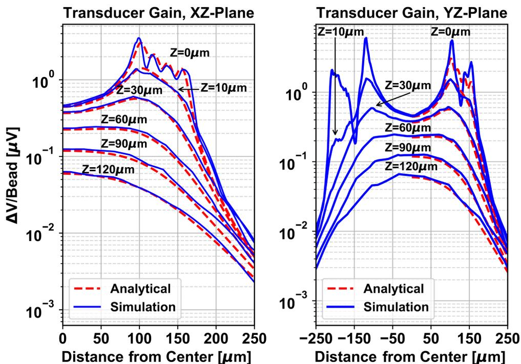
Figure 2.13: Comparison between the calculated and simulated transducer gain as a function of location above the sensor, (left) on  $xz$ -plane, (right) on  $yz$ -plane.
