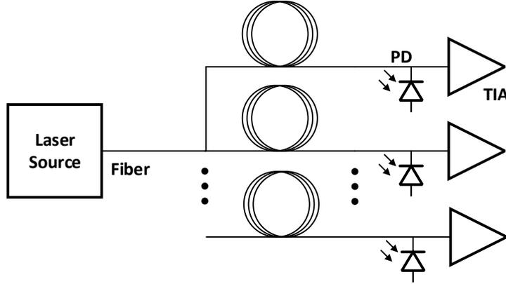
Figure 4.2: Laser clock distribution block diagram.
