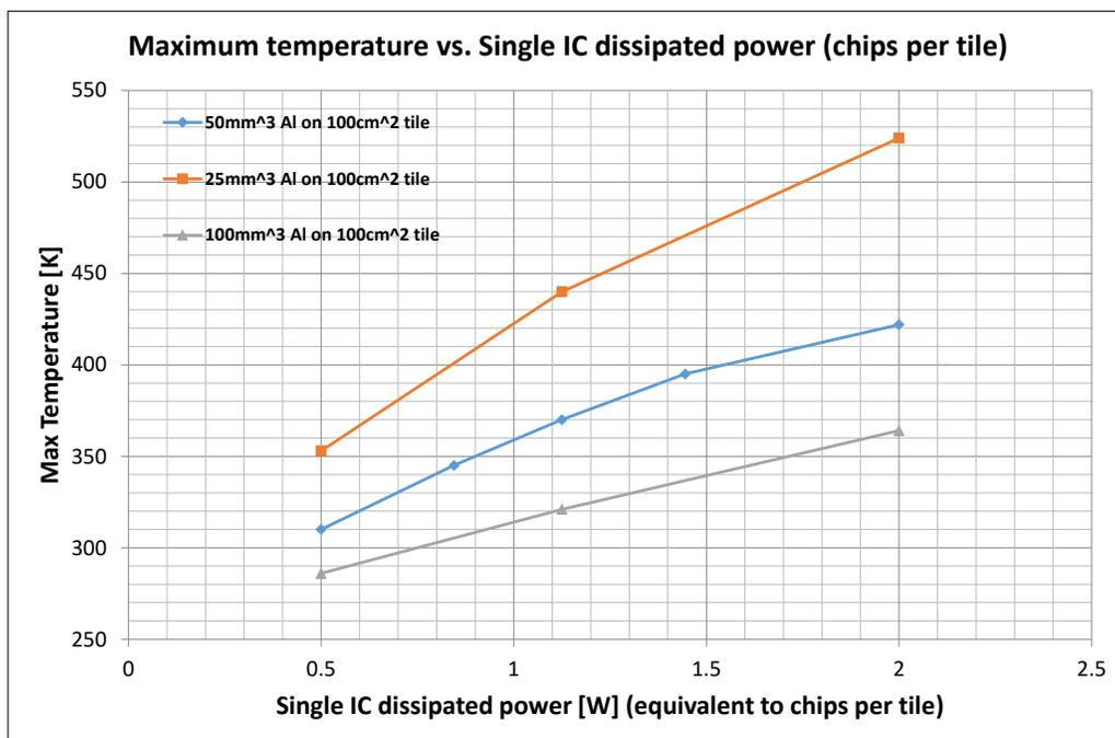
Figure 3.20: IC temperature as a function of power per chip for different ground metal volume, "equal volume" approximation.
