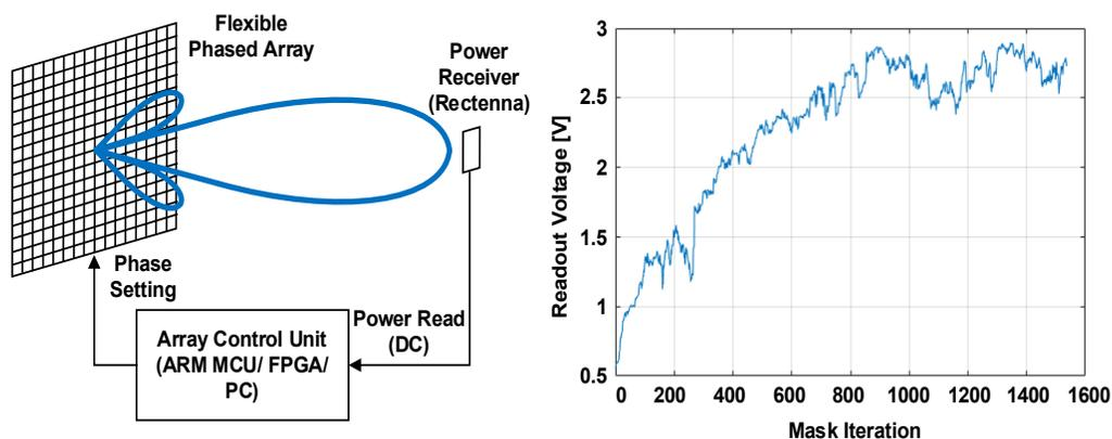
Figure 3.89: Phased array focusing setup (left) and results (right).
