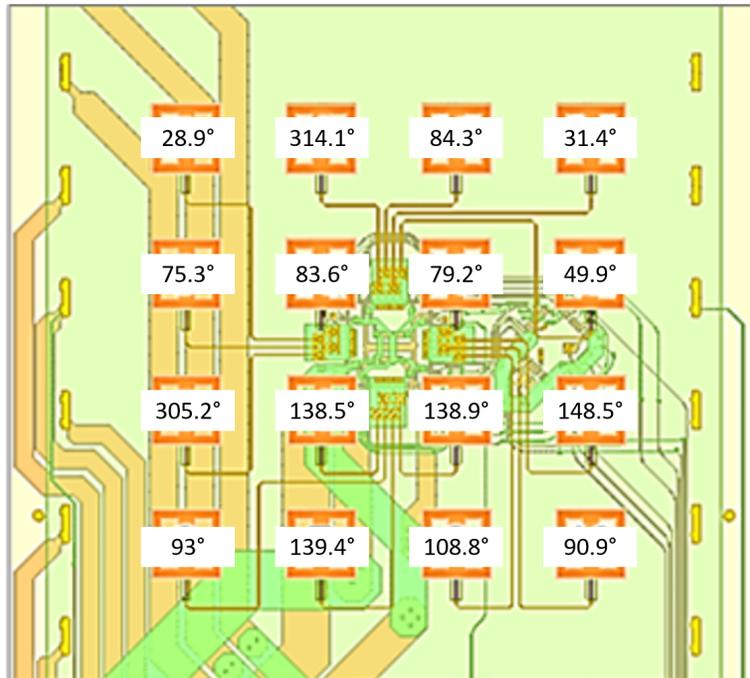
Figure 3.74: Simulated phase of each antenna output for broadside radiation [84].
