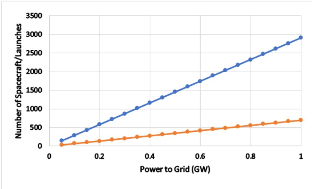
Figure 3.3:  $N_{SV}$  and  $N_L$  are linearly dependent on  $P_g$ . The slopes of the curves depend on the specifics of the space vehicle [41].
