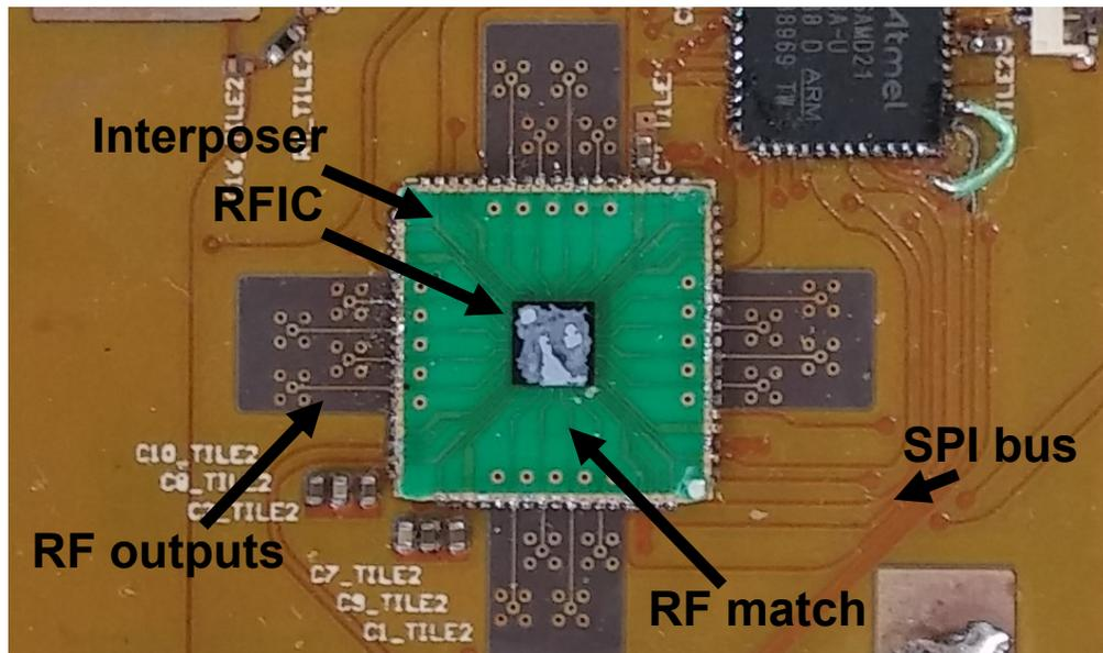
Figure 3.60: Chip-board interface with a small rigid interposer.
