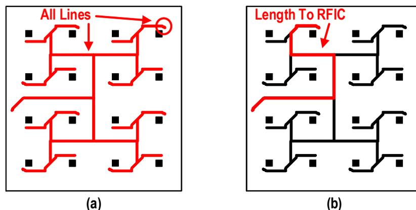
Figure 4.4: Counting the (a) total length of reference distribution lines and (b) distance from centralized source to a single IC.
