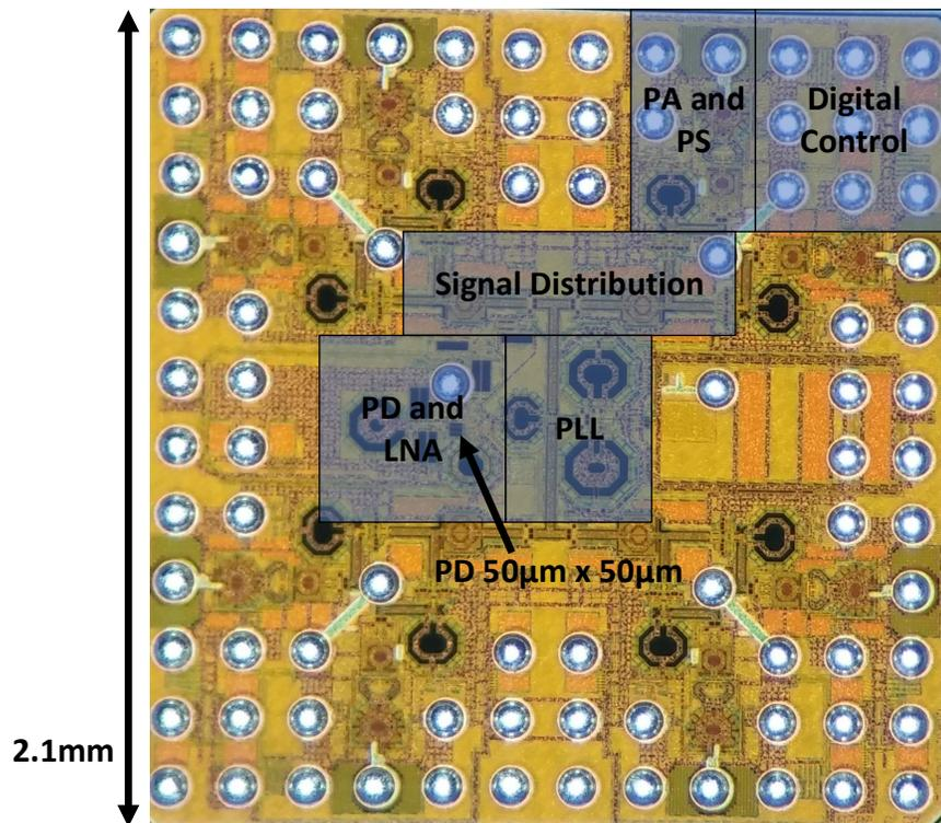
Figure 4.23: Optical reference distribution chip die photo.
