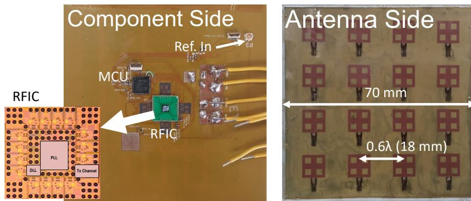
Figure 3.58: A flexible phased-array transmitter unit-cell (tile).
