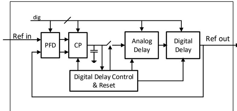
Figure 3.25: An RFIC delay-locked loop (DLL).
