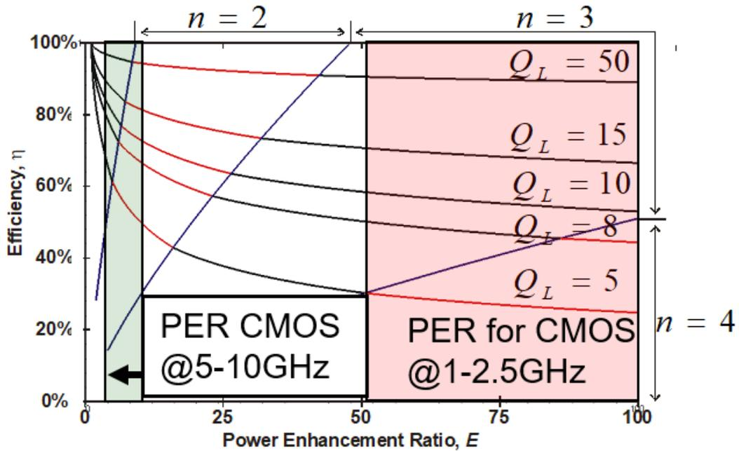
Figure 3.6: Achievable efficiency for given PER, quality factor, and number of output matching stages [55].
