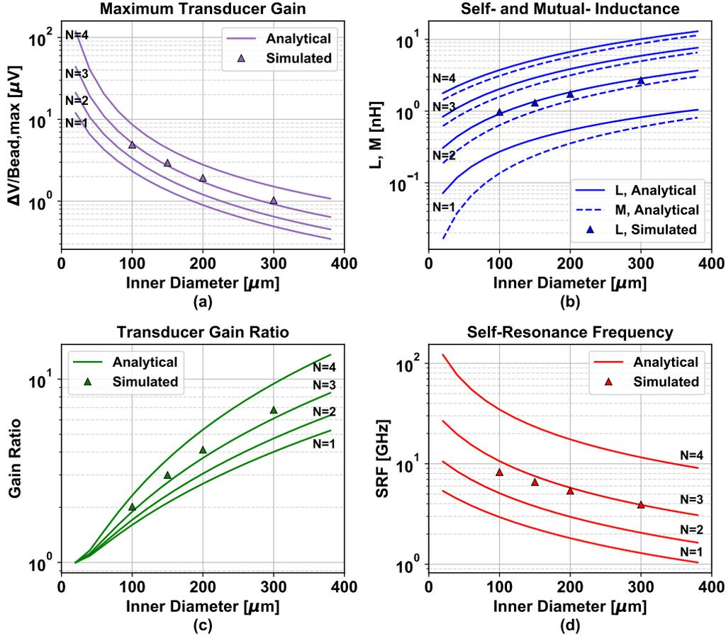
Figure 2.12: Coupled bridge design parameters as a function of the inner core diameter and the number of the single-inductor turns. (a) maximum transducer gain, (b) self and mutual inductance, (c) gain ratio, (d) SRF.
