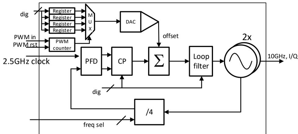
Figure 3.26: Second  $\times 4$ , 2.5 GHz to 10 GHz clock-multiplier unit (CMU).
