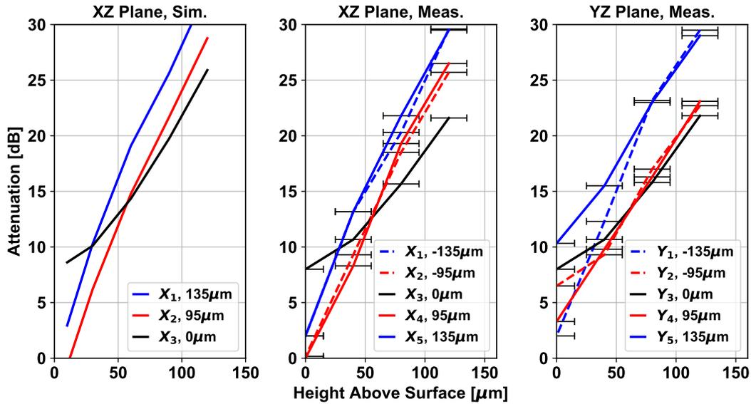
Figure 2.23: Gain profile degradation vs. height on  $yz$ -plane (right) and  $xz$ -plane (middle) compared to simulation prediction (left).
