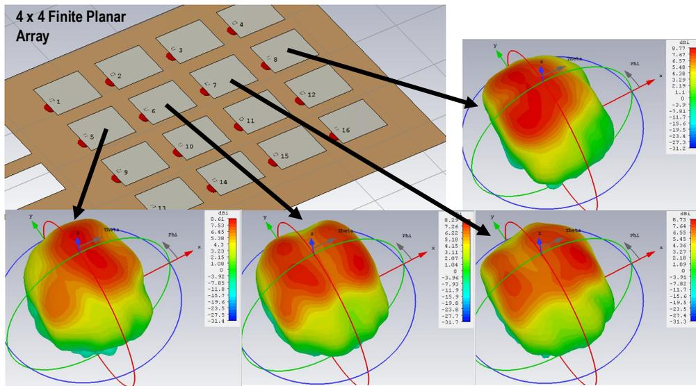
Figure 3.67: Simulated change in element pattern when placed in a finite-size array with a finite ground plane.
