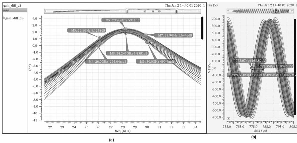
Figure 4.20: Vector modulator phase shifter. (a) Small signal gain and (b) transient phase shift simulations.
