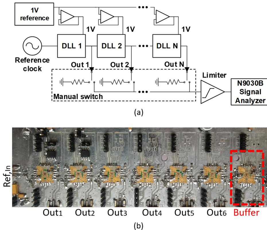
Figure 3.54: Cascaded DLL jitter (a) test setup and (b) photo.
