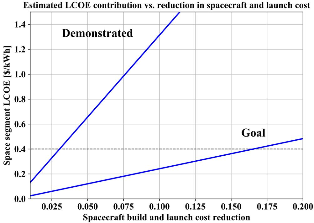
Figure 3.5: Space segment contribution to LCOE vs. reduction in the cost of build and launch of an SSP spacecraft.
