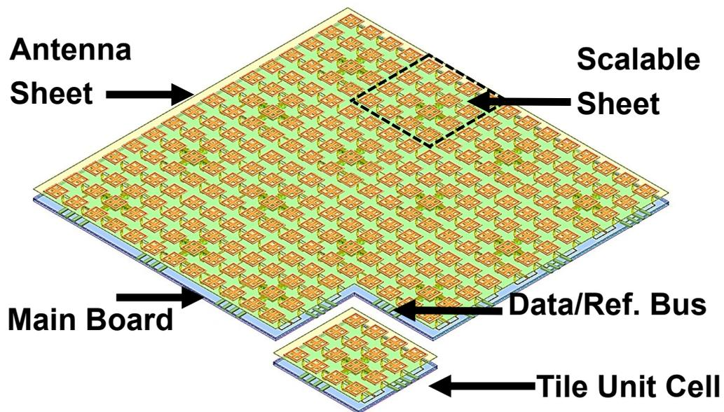
Figure 3.59: Multiple tile unit-cells combined on the same flexible laminate to form a larger array.
