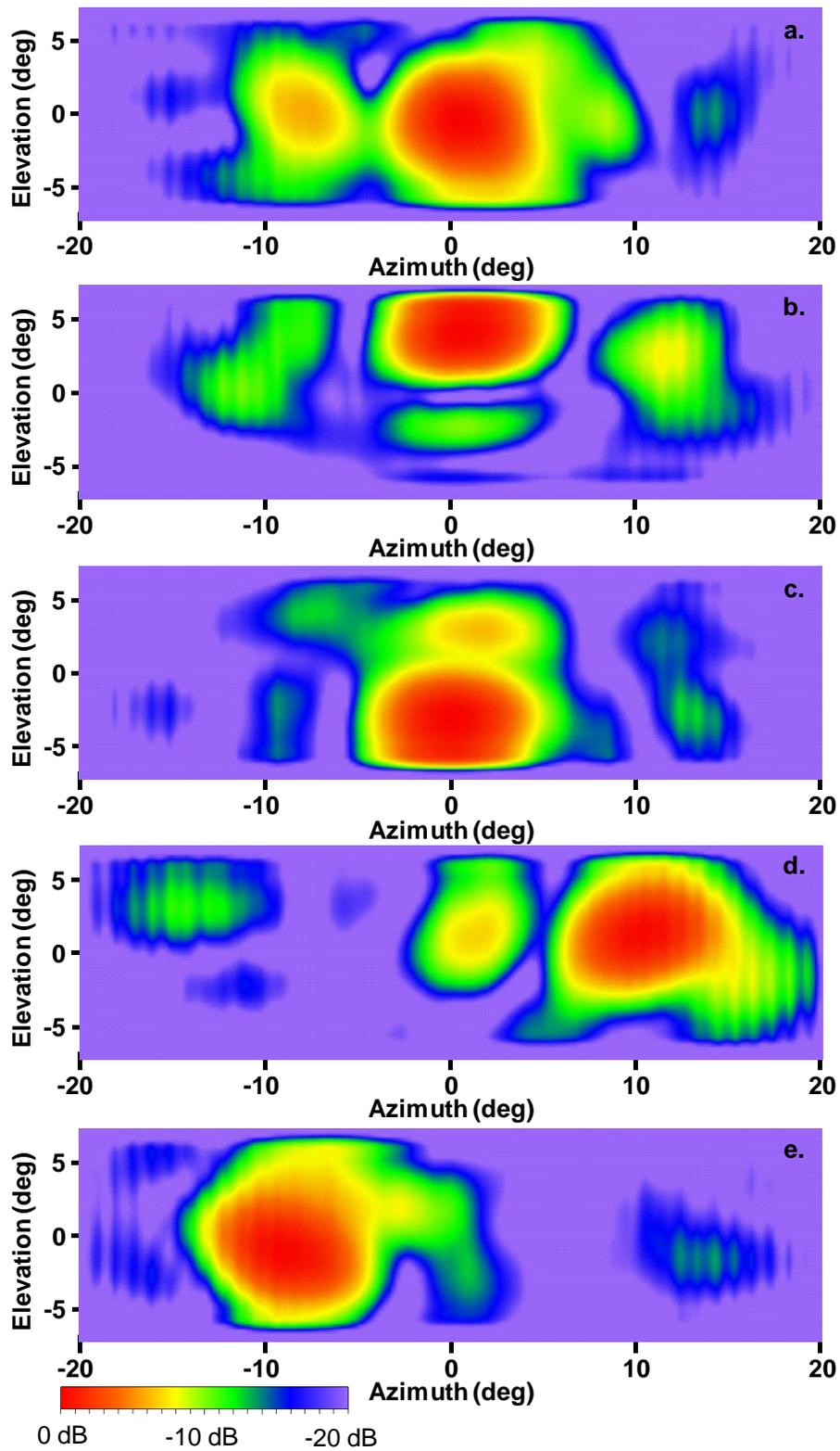
Figure 3.90: Antenna pattern of a steered phased array beam: (a) Broadside, (b) up, (c) down, (d) right, and (e) left.
