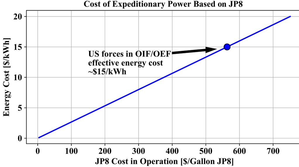
Figure 3.2: Cost of expeditionary power. Both JP8 cost and the JP8 cost of transport to destination affect total cost in operation [40].
