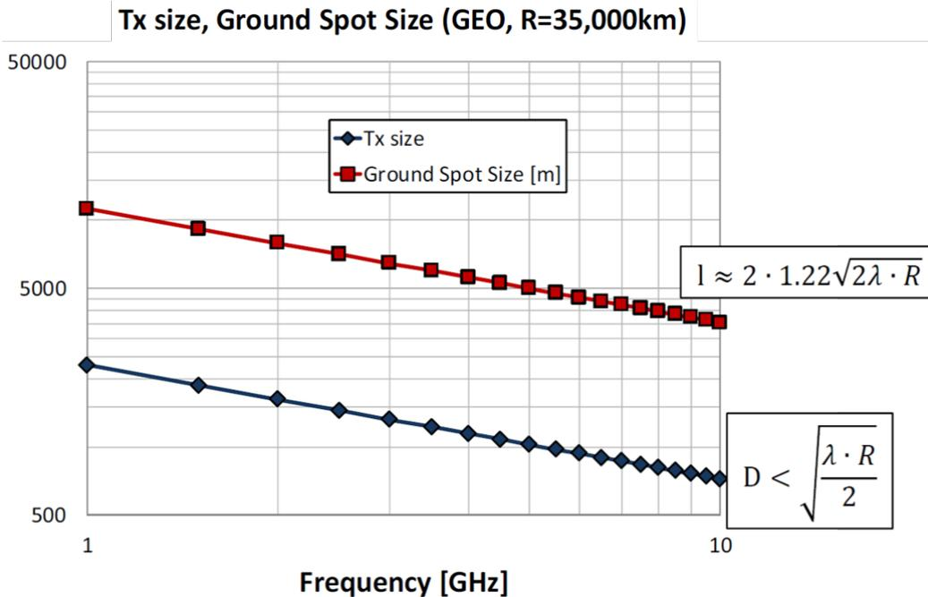
Figure 3.8: SSP array size and its far-field spot size versus frequency of operation (Fig. courtesy of Dr. F. Bohn).
