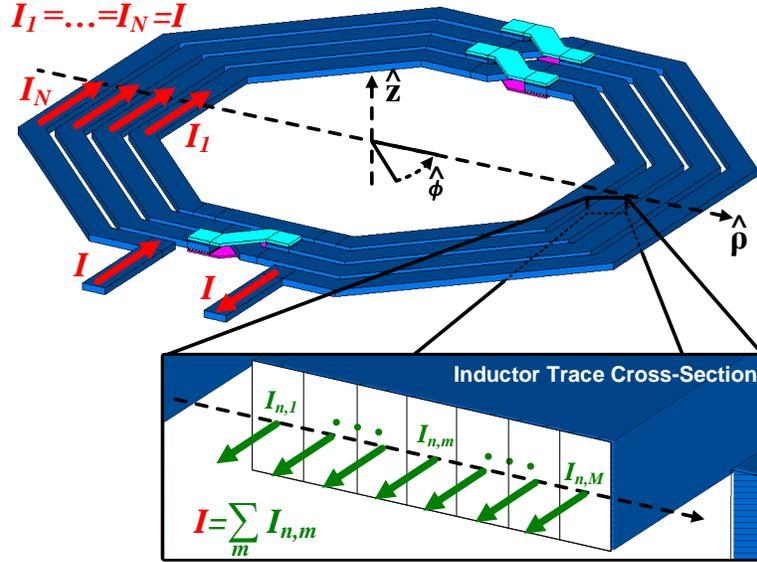
Figure 2.3: Planar inductor segmentation as one-dimensional current-loops.
