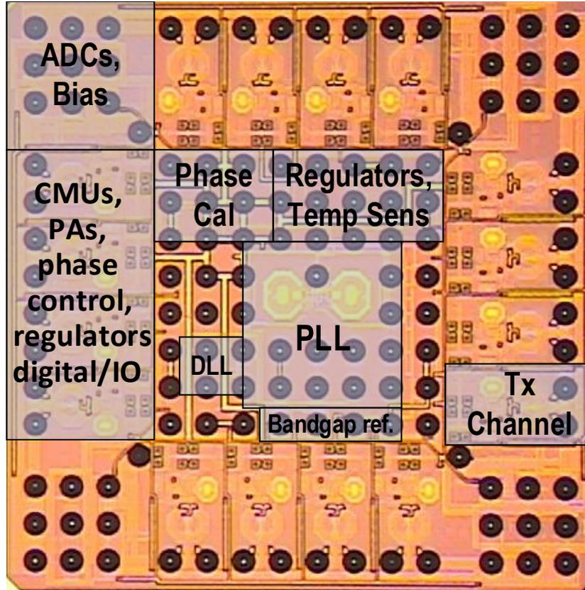
Figure 3.32: Die photo of the phased array transmitter RFIC.
