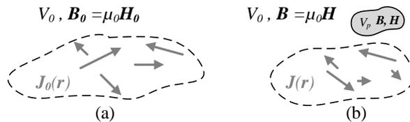
Figure 2.1: Arbitrary current density in volume  $V_0$  (a) with, and (b) without a magnetic particle  $V_p$  in the volume.
