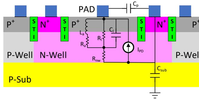
Figure 4.6: Small signal model of a CMOS PD (recreated from [106]).
