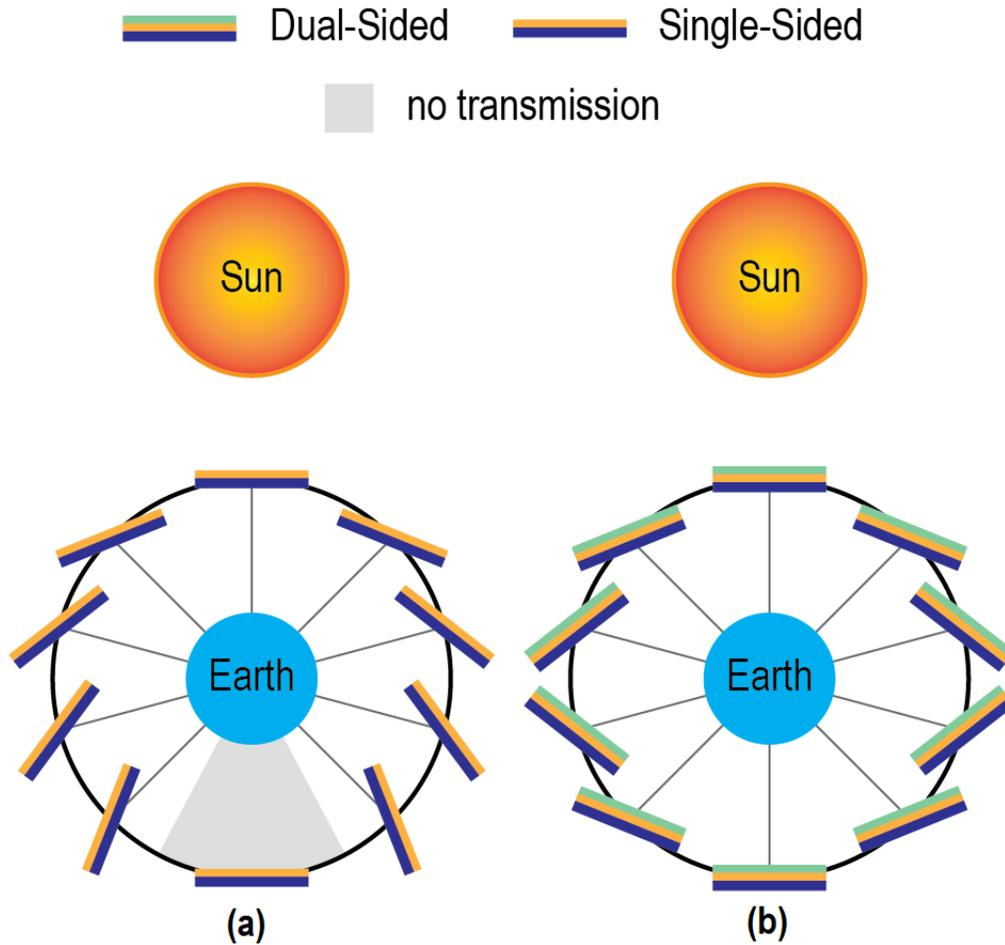
Figure 3.13: Comparison of (a) a single-sided RF/PV vs. (b) a dual-sided RF/PV SSP spacecraft coverage [41].
