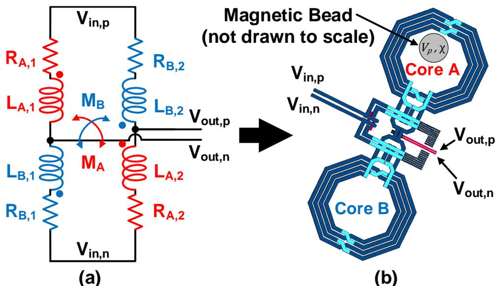
Figure 2.6: A coupled inductive bridge. (a) Circuit schematics. Inductors with the same color share a core. (b) Physical implementation with a magnetic perturbation near one of the cores (not drawn to scale).
