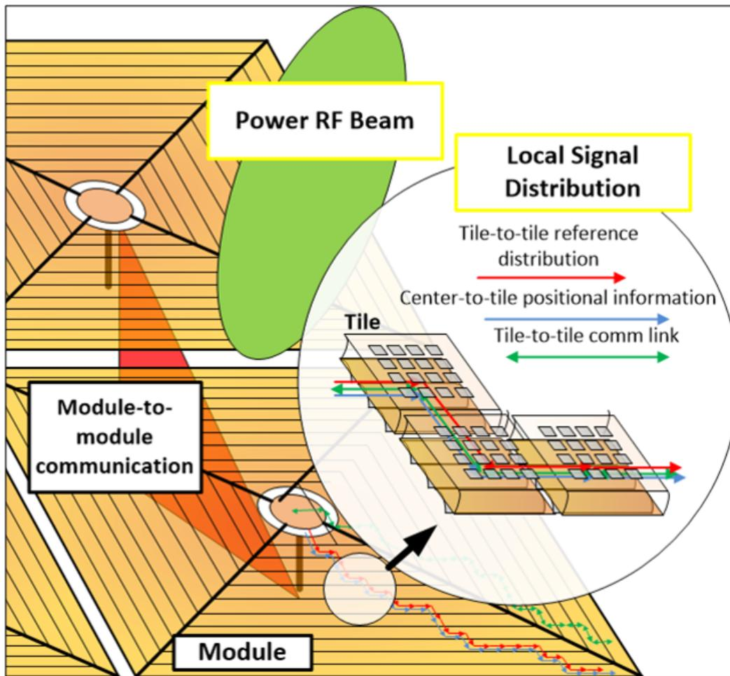
Figure 3.34: Conceptual inter-tile communication and reference distribution (Fig. courtesy of Dr. F. Bohn).
