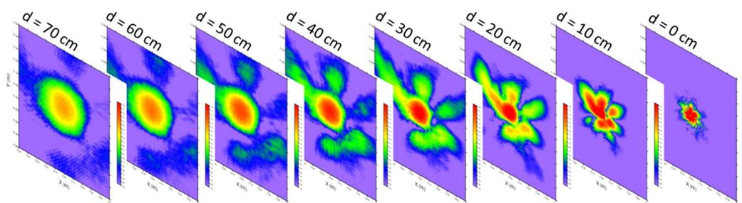
Figure 3.78: Phased array transmitter tile broadside hologram shows the evolution of the radiated field in space [84].
