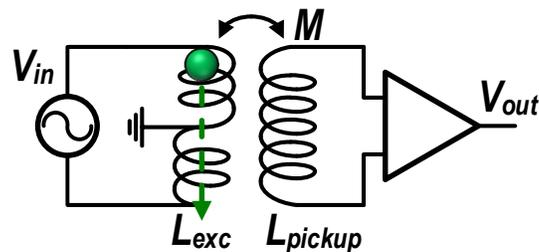
Figure 2.5: An example of a magnetic perturbation travelling in the vicinity of a transformer-based inductance-shift sensor.
