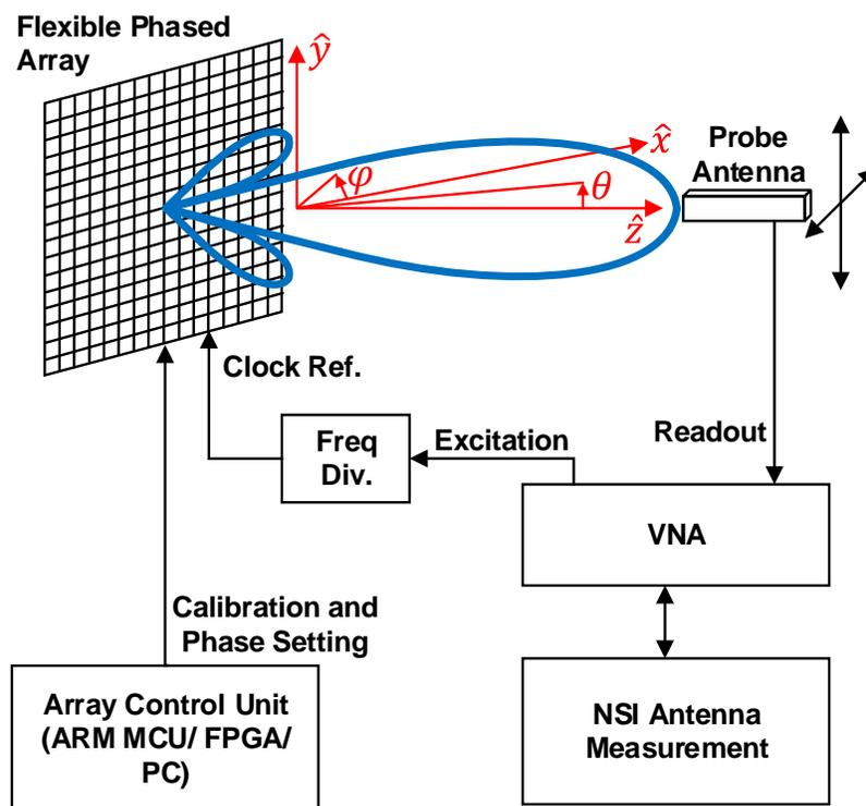
Figure 3.73: Array pattern measurement setup.
