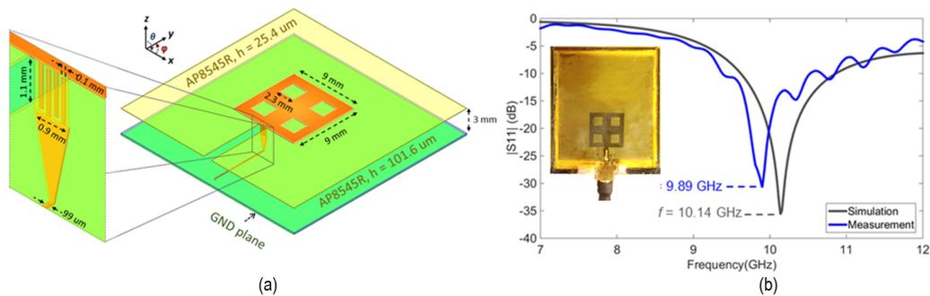
Figure 3.63: Vacuum-suspended patch antenna: (a) designed and (b) fabricated/measured [84].
