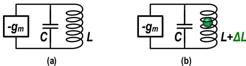
Figure 2.4: An oscillator circuit (a) with and (b) without a magnetic perturbation in the inductor core.
