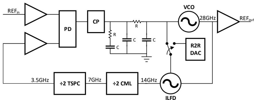
Figure 4.14: An  $\times 8$ , 3.5 GHz to 28 GHz PLL schematic
