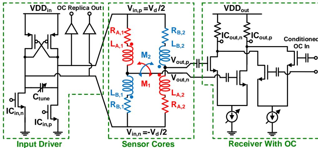
Figure 2.16: Simplified schematics of the fabricated IC.
