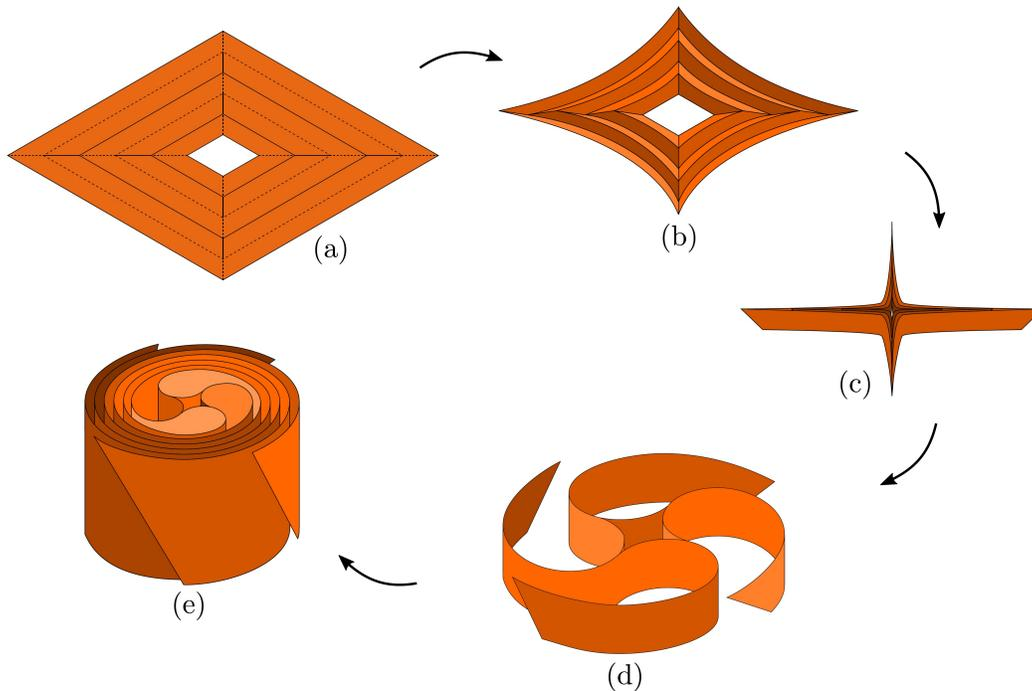
Figure 3.12: SSP spacecraft packaging: (a) Deployed, (b) collapsed plain, (c) folded inwards, (d) collapsed sideways and rolled, and (e) packed [59].
