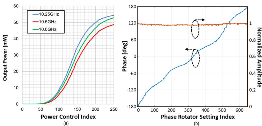
Figure 3.56: RFIC output: (a) power and (b) phase shift range [84].
