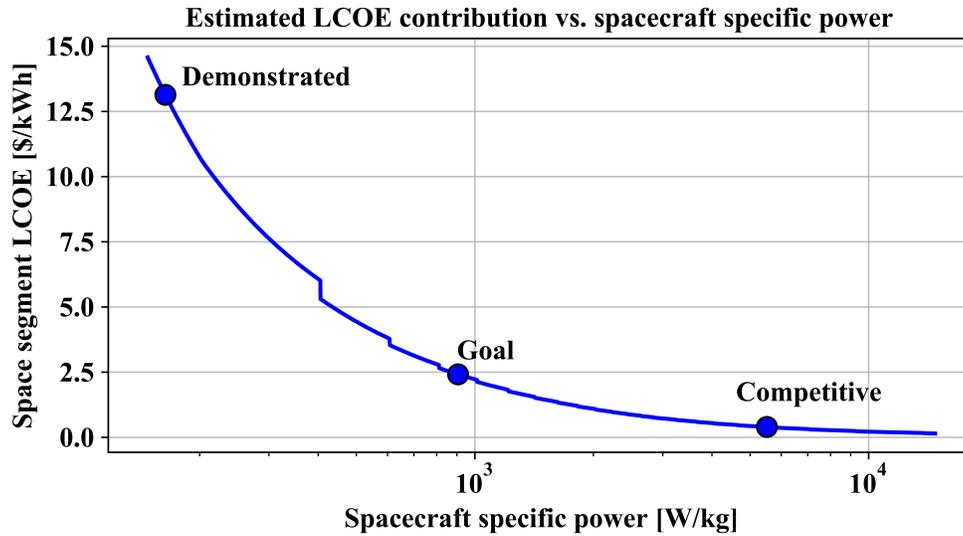
Figure 3.4: Space segment contribution to LCOE vs. spacecraft specific power.
