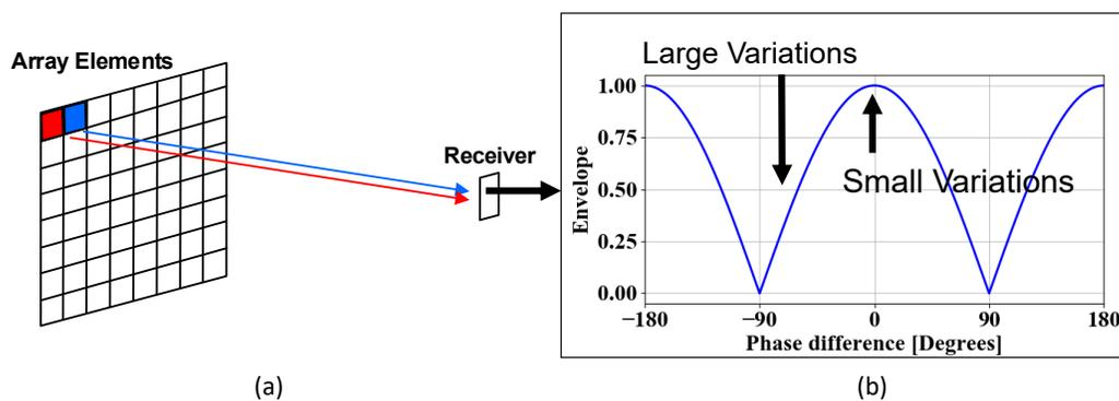
Figure 3.87: The challenges in calibration of large arrays. (a) Physical problem setup and (b) implication on receiver dynamic range.
