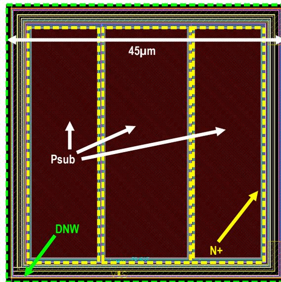
Figure 4.9: Photodiode layout.
