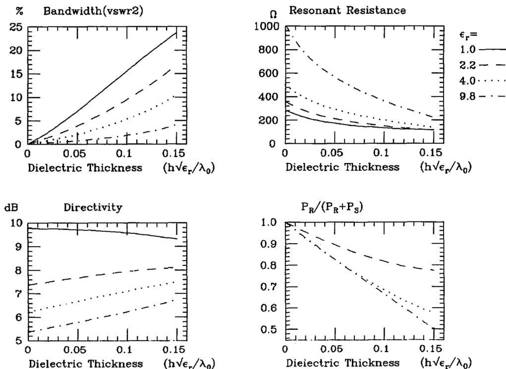
Figure 3.62: Bandwidth, directivity, radiation resistance, and efficiency with respect to surface waves excitation for a resonant square element as a function of dielectric thickness for different  $\epsilon_r$  [85].
