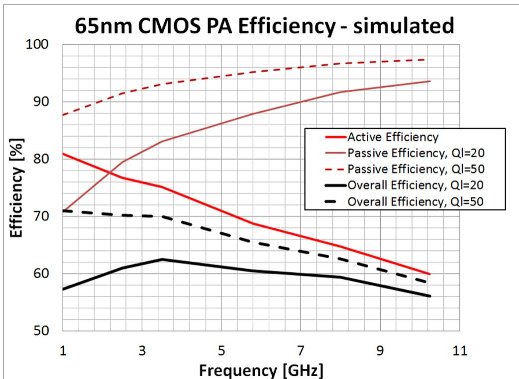
Figure 3.7: Power amplifier efficiency versus frequency as a combination of passive and active component efficiencies (Fig. courtesy of Dr. F. Bohn).
