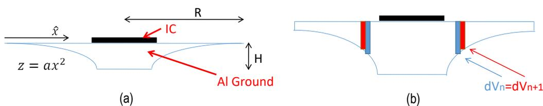
Figure 3.17: Quadratic ground plane profiles. (a) Zero edge thickness. (b) Equal volume.
