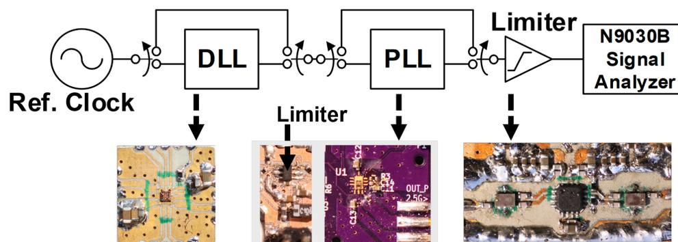
Figure 3.51: Cascaded PLL and DLL measurement setup.
