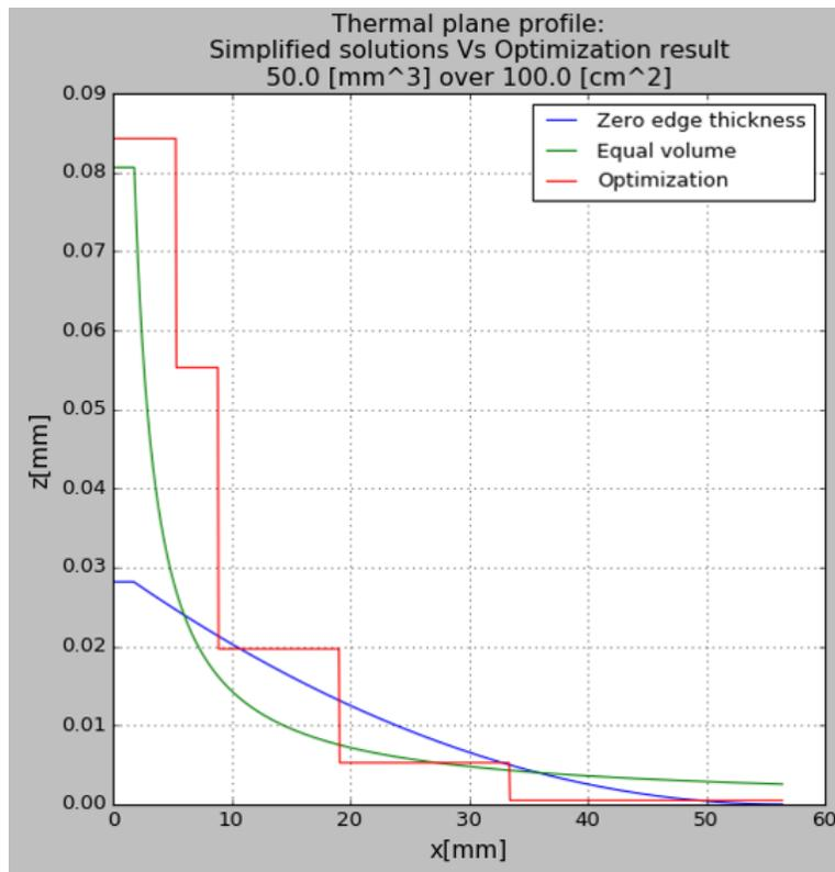
Figure 3.18: Varying ground thickness for each of the thermal conduction improvement schemes.
