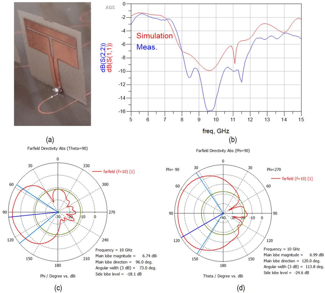
Figure 3.69: Vertical sheet antenna (a) test structure (the plastic support should be removed or changed in the final design), (b) input matching, (c) antenna pattern 0°, (d) antenna pattern 90°.
