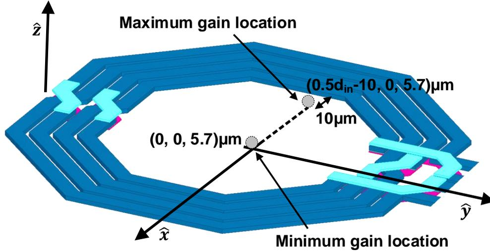
Figure 2.14: Bead location for the calculation of maximum and minimum gain parameters.
