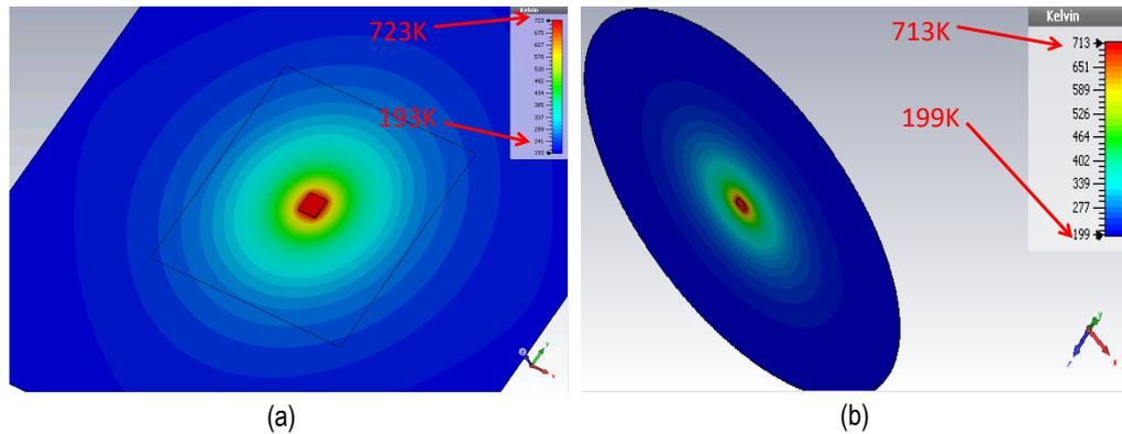
Figure 3.15: IC temperature in space due to heat dissipation on (a) a square tile and (b) a circular tile.
