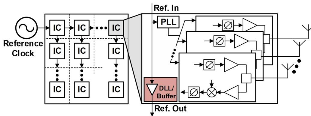
Figure 3.35: Clock distribution to CMOS-driven phased array.
