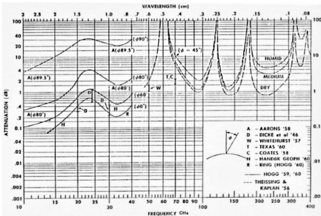
Figure 3.9: FCC's graph of RF attenuation through the atmosphere [57][58]
