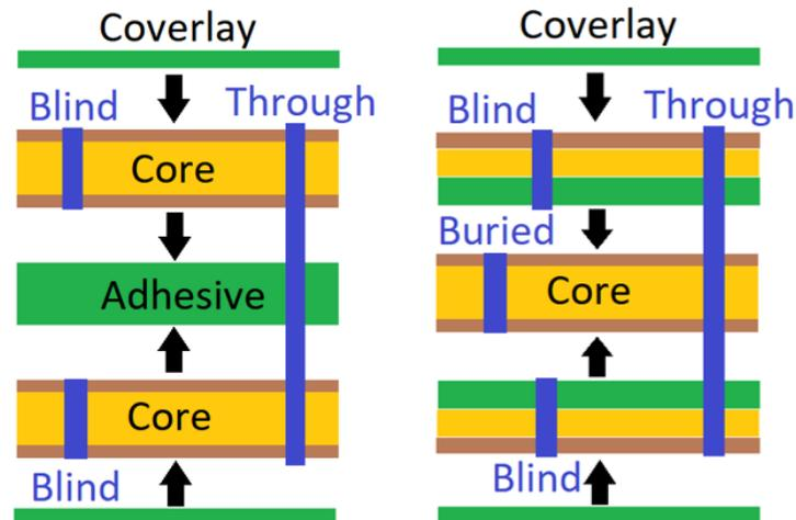
Figure 3.72: Fabrication options for a flexible 4-layers PCB.
