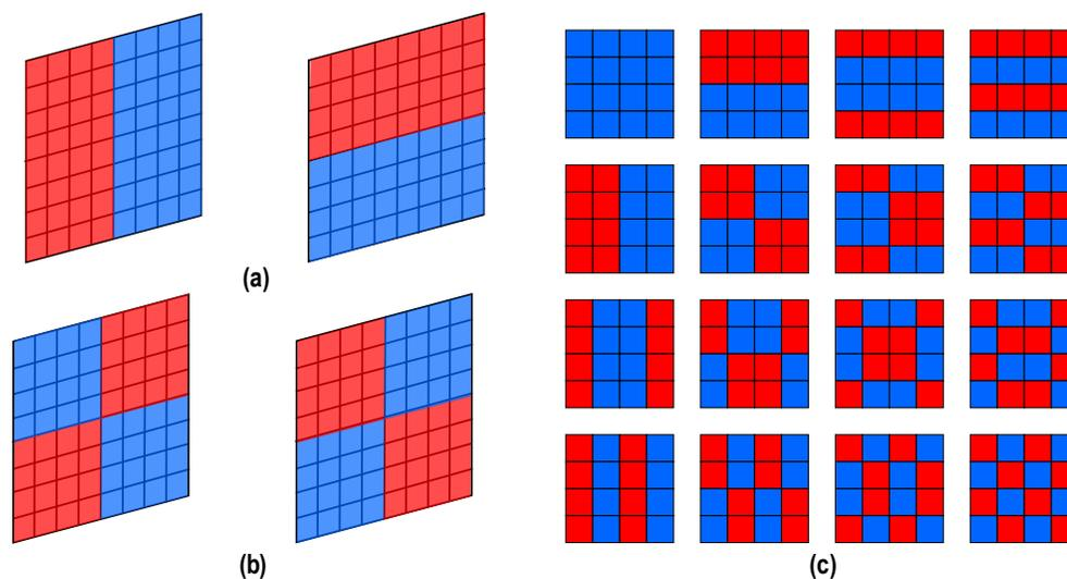
Figure 3.88: Selecting groups of elements for phased array calibration/focusing: (a) half the array elements and (b) fourth of the array elements. (c) An example for a selection of groups of elements in a 16-element array to span an orthogonal phase space.
