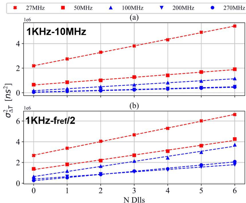
Figure 3.55: Cascaded DLL jitter. (a) 1kHz - 10MHz measurement, and (b) 1kHz- $f_{ref}/2$  measurement. Red and blue curves indicate locking to inverted/non-inverted output, respectively.
