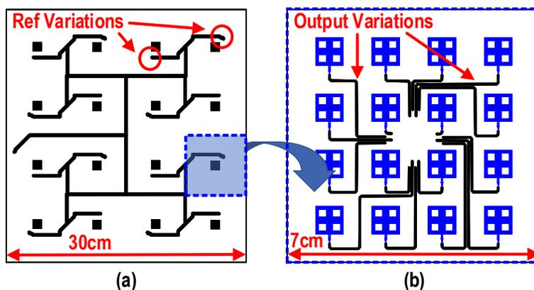
Figure 3.33: Length variations due to (a) reference distribution routing and (b) output antenna traces.
