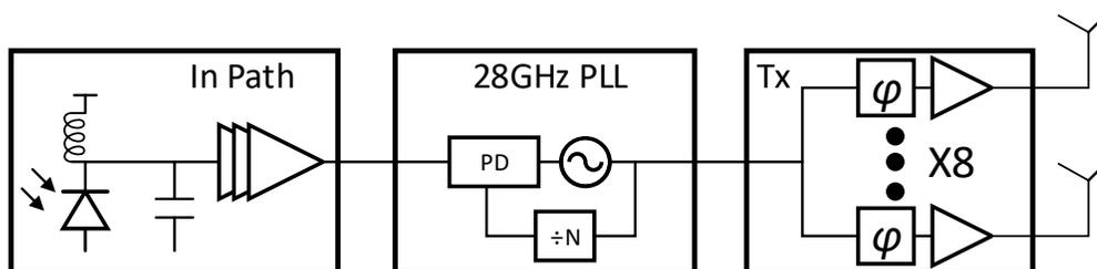
Figure 4.5: Optical reference chip top block diagram.
