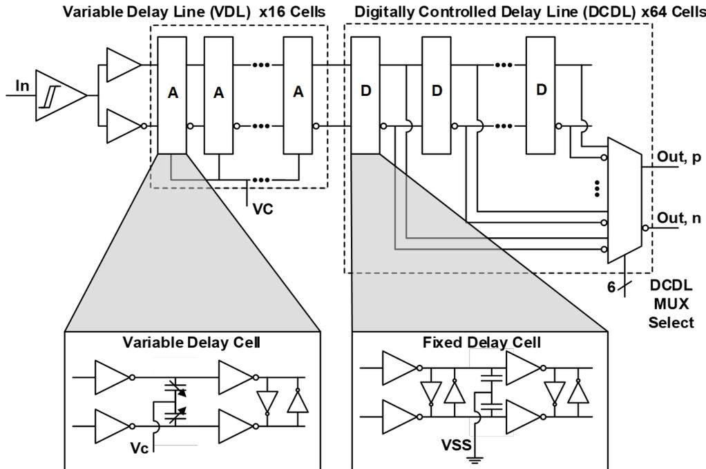
Figure 3.40: Hybrid delay line structure.
