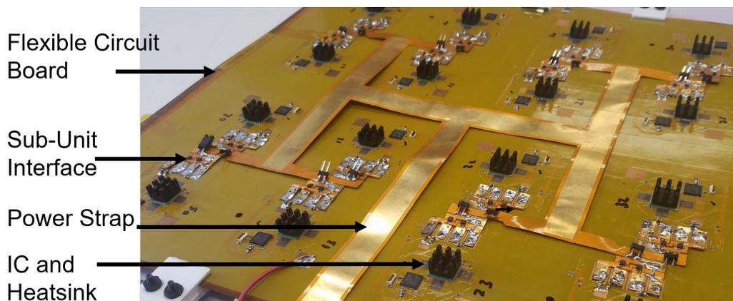
Figure 3.84: Power strap and supply interface for the flexible phased array transmitter.
