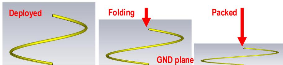
Figure 3.70: Collapsible spiral spring concept.
