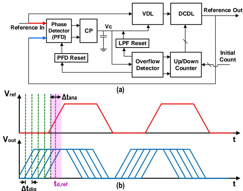
Figure 3.38: Hybrid DLL function. (a) Schematic and (b) hybrid phase tracking.
