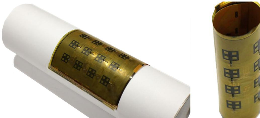
Figure 3.66: Antenna packing curvature limit due to different radii of the two flexible sheets.
