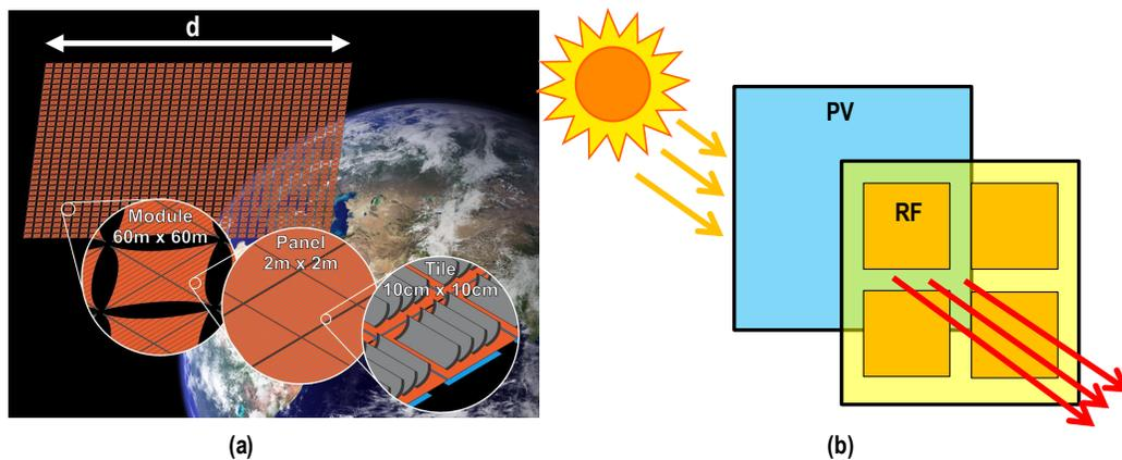
Figure 3.11: Conceptual SSP array: (a) Array, spacecraft, panel and tile levels and (b) concept of operation of an SSP sheet PV-RF power conversion system.
