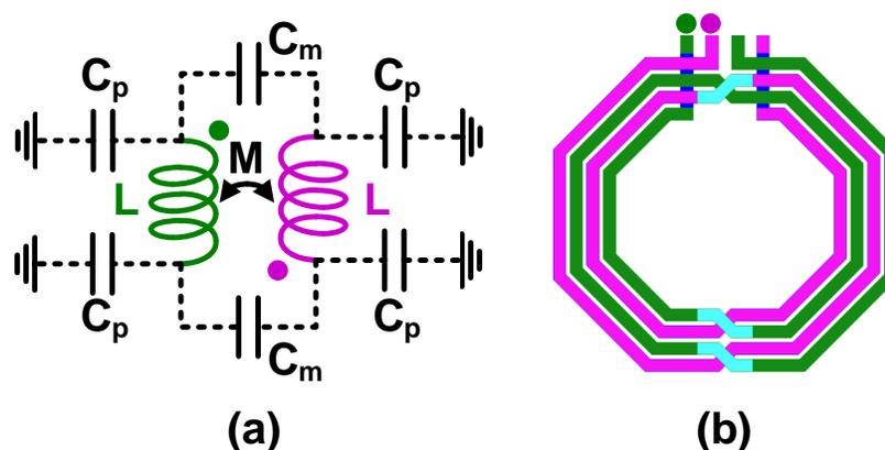
Figure 2.9: A high frequency (a) coupled inductor model and (b) exemplary 2-turn layout.
