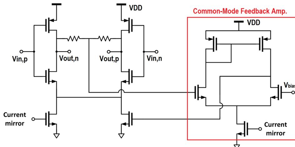
Figure 4.12: A common-mode stabilized inverter amplifier (Fig. courtesy of C. Ives).
