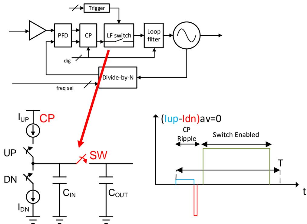
Figure 3.44: Pass-through switch structure for up/down mismatch spur prevention.
