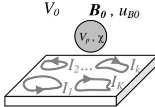
Figure 2.2: Magnetic bead with volume  $V_p$  and susceptibility  $\chi$  in a space  $V_0$  with an unperturbed magnetic energy density of  $u_{B0} = B_0^2/2\mu_0$ .
