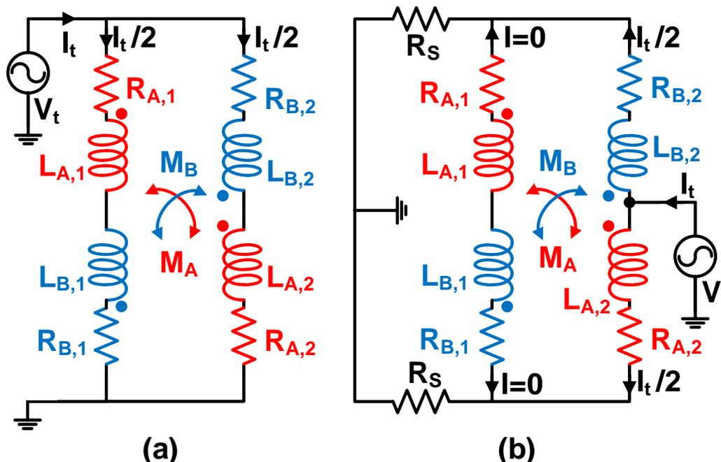
Figure 2.7: Schematic circuits of the sensor's (a) input impedance test circuit and (b) output impedance test circuit.
