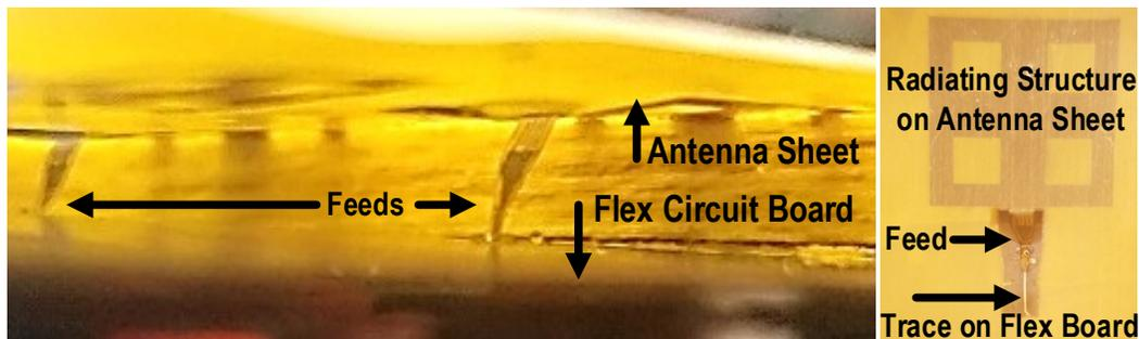
Figure 3.65: Flexible patch antenna sheet and feed above ground.
