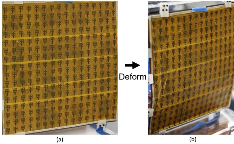
Figure 3.91: A flexible phased array transmitter: (a) flat and (b) deformed.
