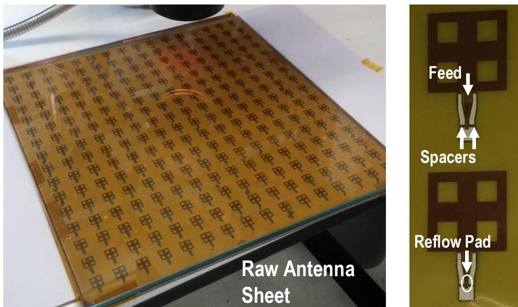
Figure 3.85: Antenna sheets: (a) a raw sheet and (b) a close-up on the board interface.
