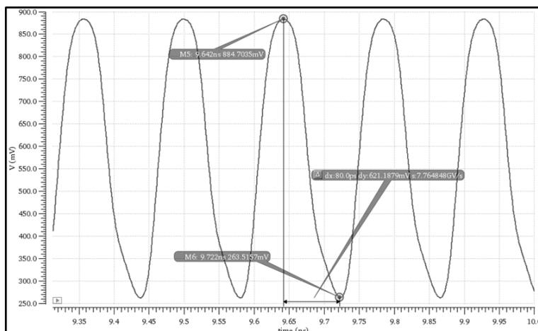
Figure 4.13: Transient simulation of the input chain's output (Fig. courtesy of C. Ives).
