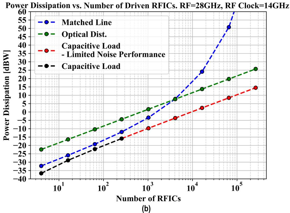
Figure 4.3: Comparison of distribution network power loss for different distribution schemes at (a) 28GHz and (b) 10GHz.
