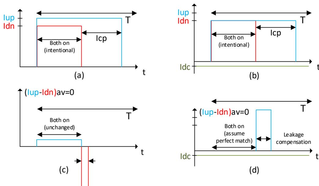
Figure 3.43: Reference spur sources: (a) Charge pump mismatch and (b) DC current leakage. Periodic charge transients on control voltage line (c) due to up/down mismatch and (d) DC leakage.
