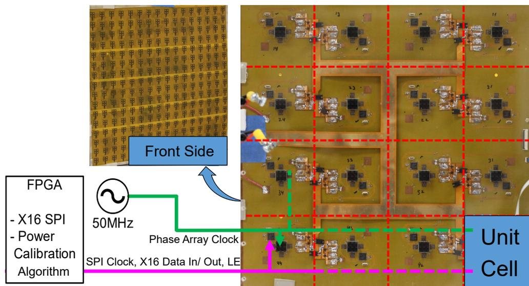
Figure 3.83: An assembled flexible phased array transmitter.
