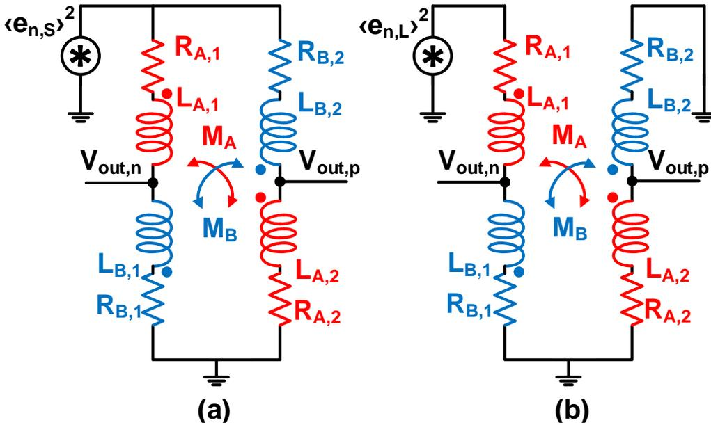
Figure 2.8: Schematic circuits of the sensor's (a) excitation noise and (b) single inductor equivalent thermal noise.
