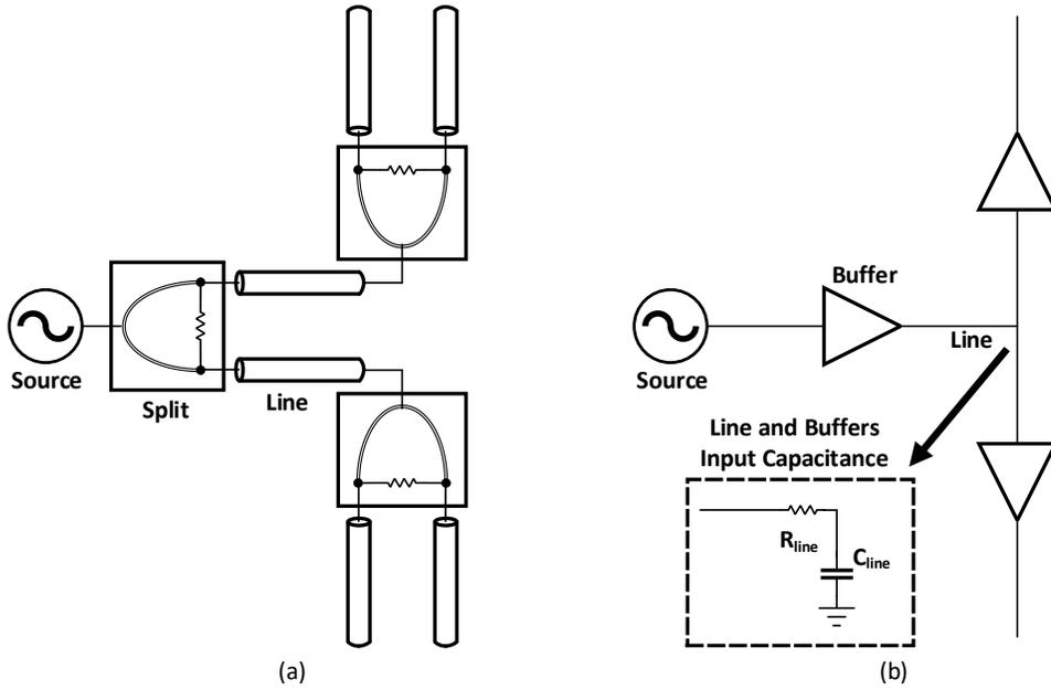
Figure 4.1: High frequency clock distribution schemes: (a) RF based and (b) laser based.
