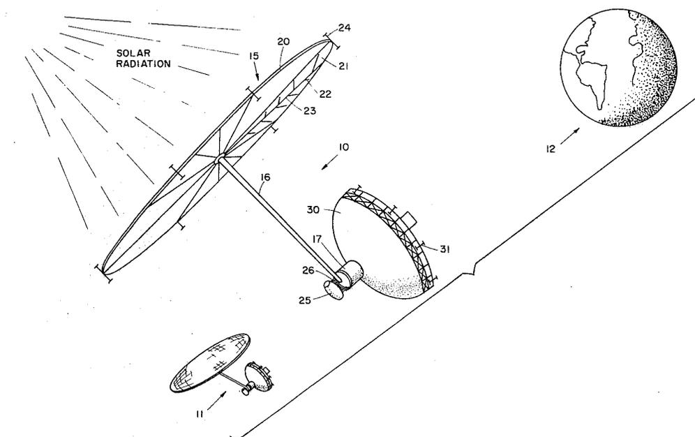
Figure 3.1: Glaser's original patent drawing of a solar power satellite.
