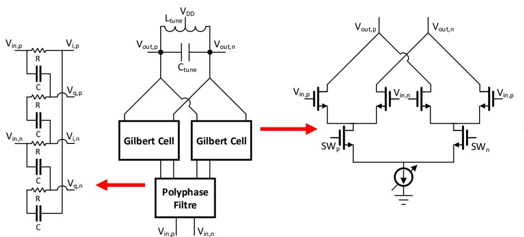
Figure 4.19: Output channel vector modulator phase shifter schematic.
