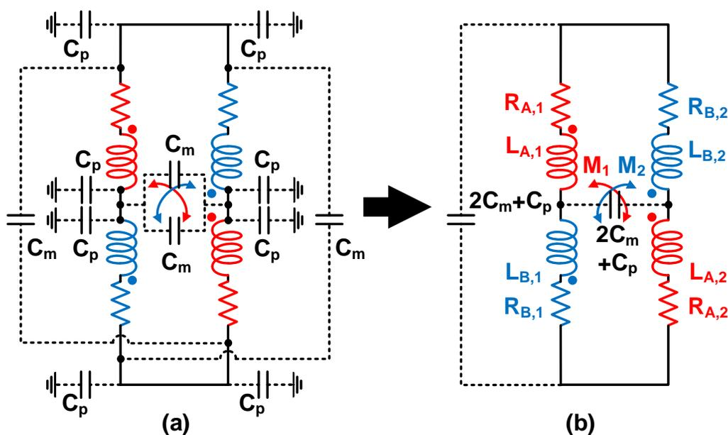
Figure 2.10: A high frequency (a) coupled bridge model and (b) equivalent circuit.
