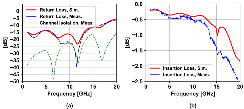
Figure 3.61: Chip interposer measuring (a) return loss and (b) insertion loss.
