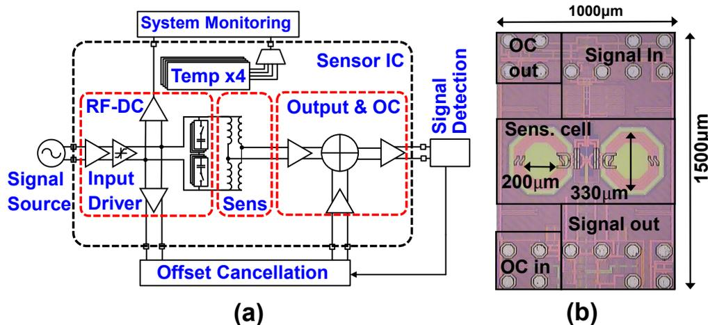
Figure 2.19: Top level view: (a) simplified measurement system schematics and (b) the chip die photo.
