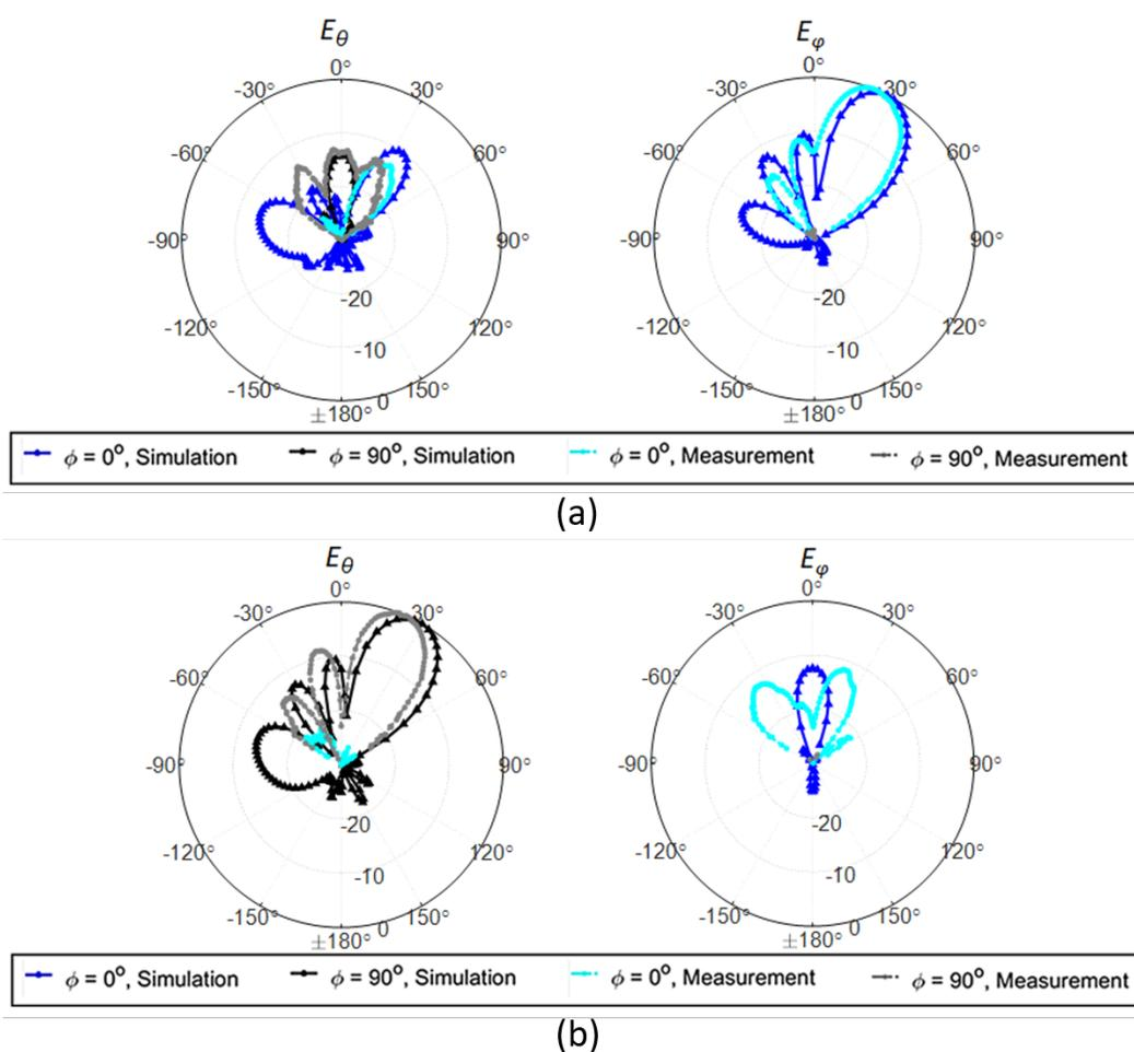
Figure 3.77: Steered beam pattern (a) up and (b) left [84].
