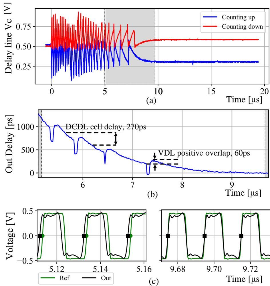
Figure 3.50: Hybrid lock process at different time scales. (a) Loop filter control voltage, (b) time delay between reference and output clocks, and (c) time domain waveforms (adjusted).
