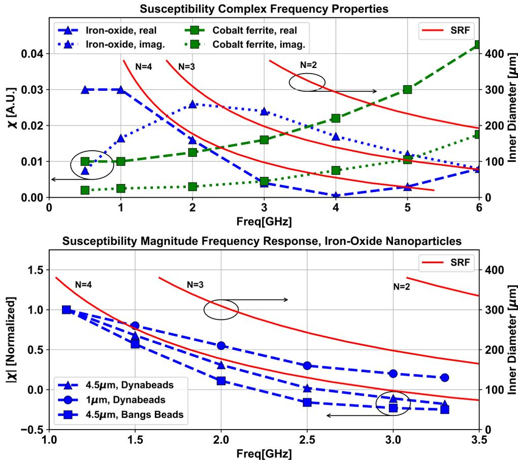
Figure 2.11: Top: complex frequency response of two types of magnetic bead [9]. Bottom: change in magnitude of  $\chi$  vs. frequency [15] for three bead types.
