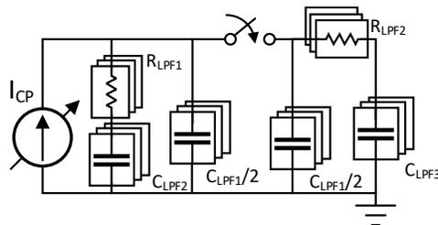
Figure 3.42: A variable loop filter for the optimization of the PLL noise performance at different frequencies.
