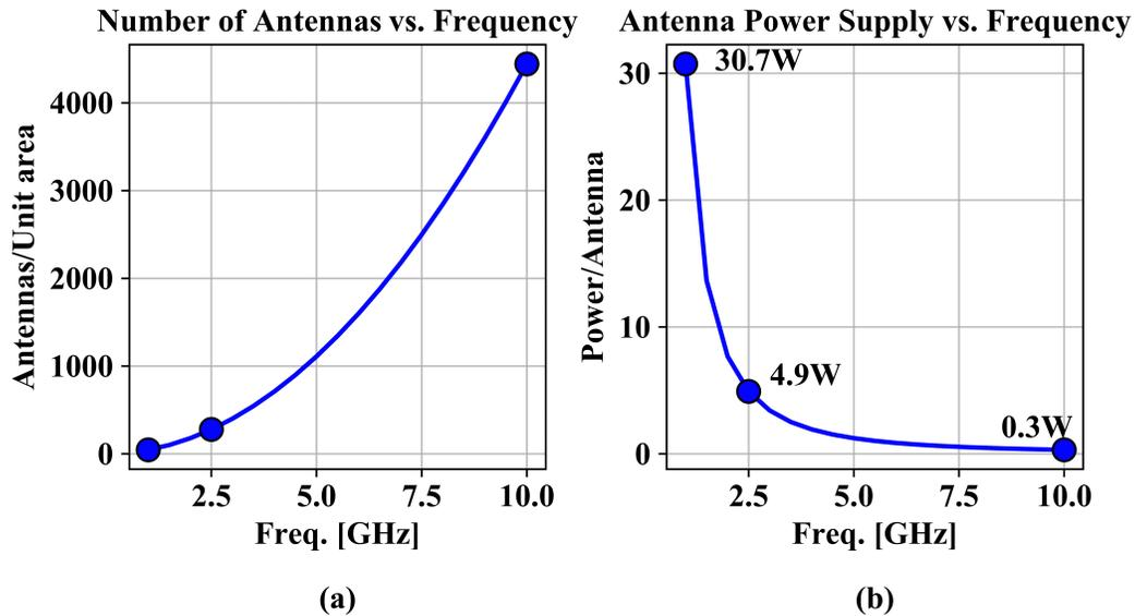
Figure 3.10: Change in (a) number of antennas per unit area and (b) power supply to be radiated by each antenna vs. frequency of operation.
