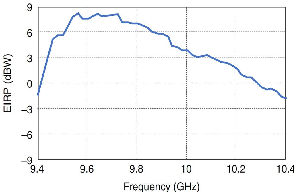
Figure 3.79: Phased array transmitter tile EIRP (image reproduced from [84]).
