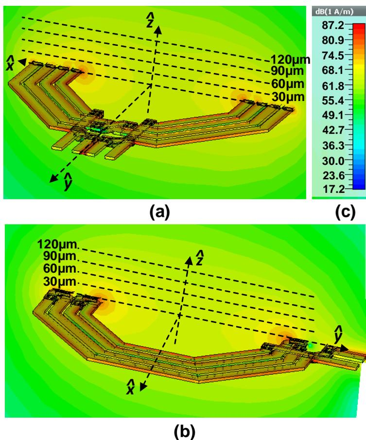
Figure 2.15: Simulated magnetic field intensity with core inductors shorted in series. (a) On  $xz$ -plane, (b) on  $yz$ -plane, with (c) recorded values in  $\text{dB}(A \cdot \text{m}^{-1})$  (to increase contrast).
