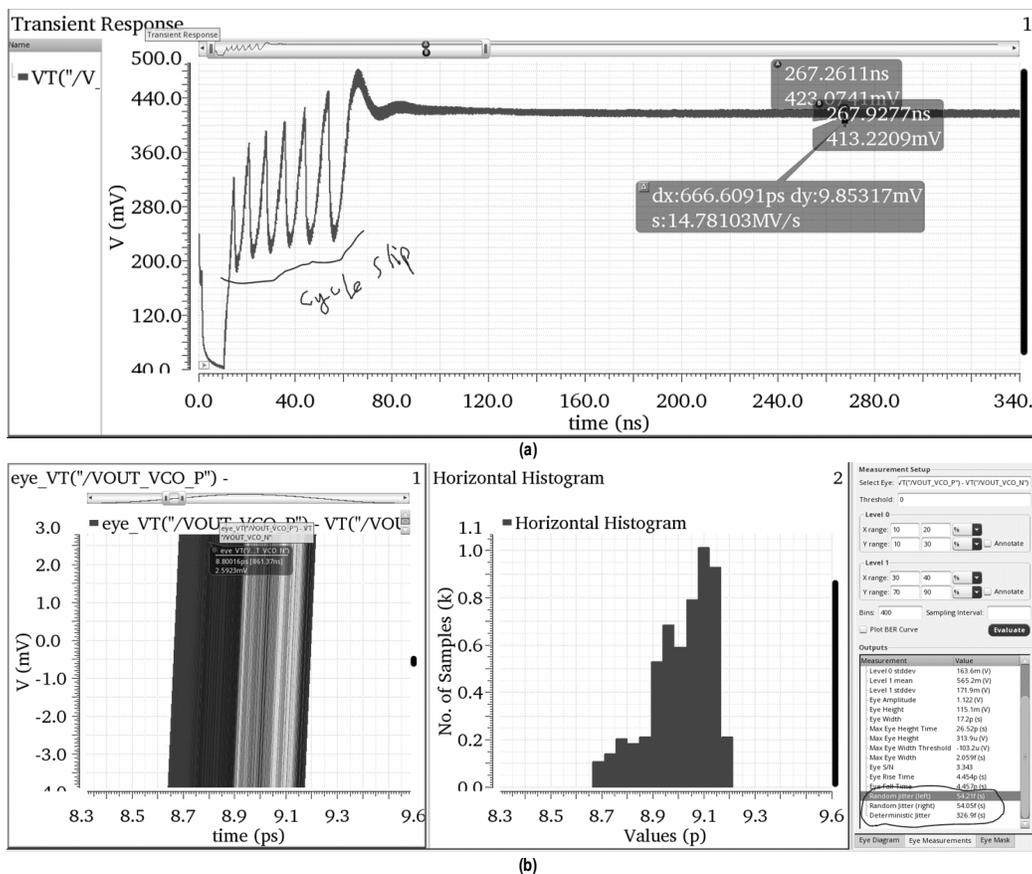
Figure 4.18: 28GHz PLL simulation of (a) transient VCO control voltage and (b) transient jitter. Estimated jitter is  $\approx 60$  fs.
