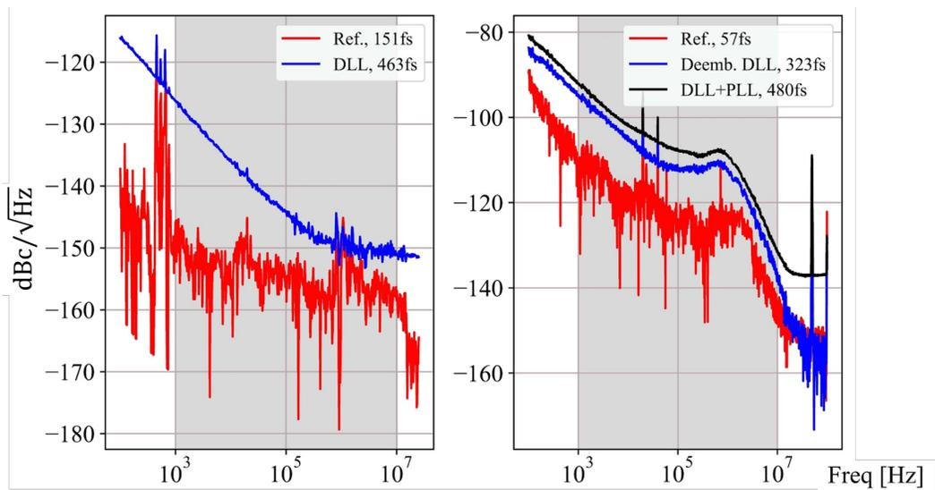
Figure 3.52: Noise performance. (a) 50MHz DLL phase noise and rms jitter, and (b) 2.5GHz post PLL phase noise and rms jitter. The red curves are the rms measurement uncertainty.
