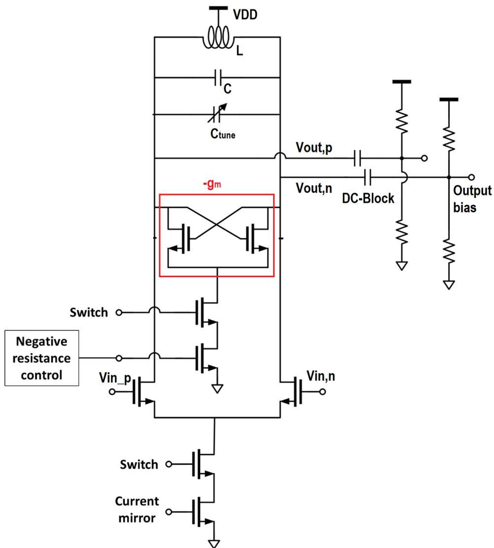
Figure 4.11: PD LNA with a gain-boost  $-g_m$  cell (Fig. courtesy of C. Ives).
