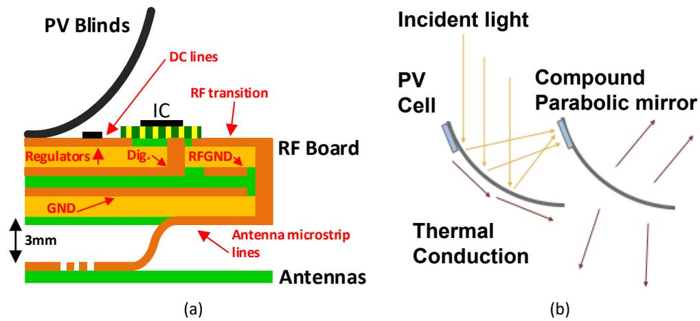
Figure 3.80: Integrated tile: (a) structure and (b) PV reflector concept.
