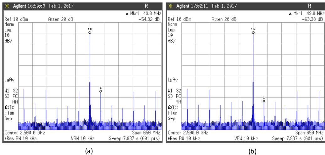
Figure 3.46: PLL spur reduction switch measurement.
