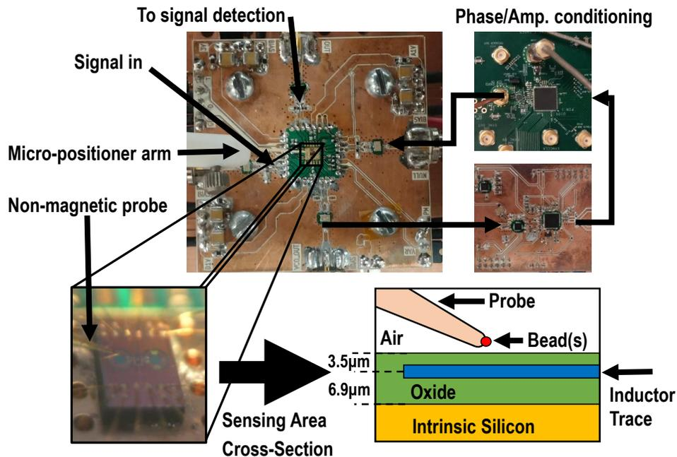
Figure 2.24: Measurement system, including OC circuitry.
