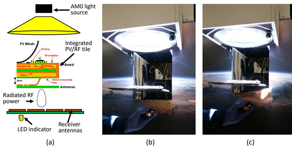
Figure 3.82: Testing an integrated RF-PV tile under AM0 light source. (a) Measurement setup, (b) demonstration of RF lighting an indicator LED. (c) Power is not transferred when line-of-sight is lost.
