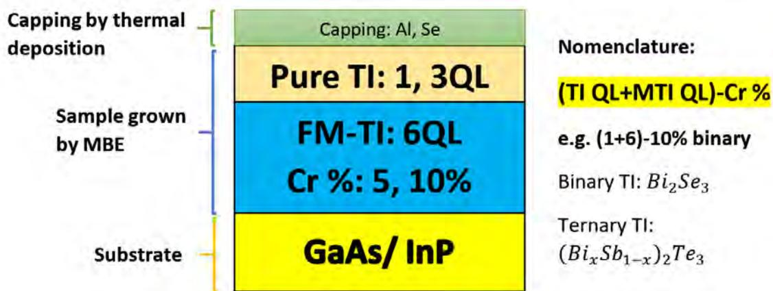
**Figure 3.4:** Schematic structure (side view) of a bilayer TI/MTI sample and its nomenclature.
