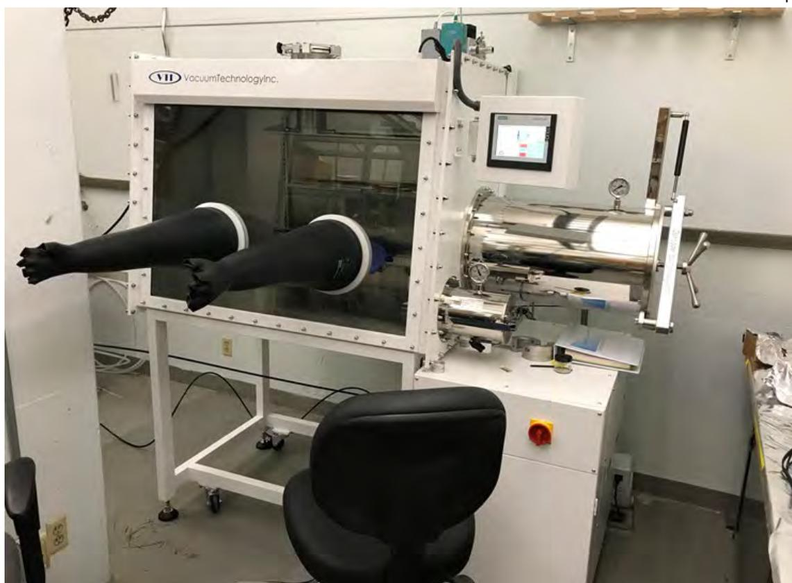
**Figure 2.18** Real image of the new glove box. With the latest design, operation inside the glovebox is much more convenient than that inside the old glovebox.
