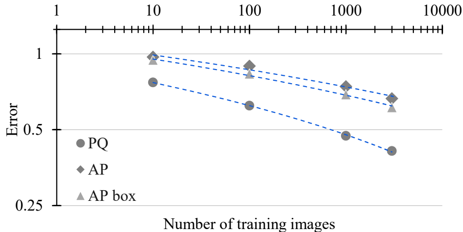
Figure 4.3: Model performance vs training set size on Cityscapes. We train UPSNet-50 models on various Cityscapes subsets ranging from 10 to 2,975 images. PQ : panoptic quality. AP : mean average precision of instance segmentation evaluated at 0.5:0.95. AP box : mean average precision of detection evaluated at 0.5:0.95. Dashed curves are log-linear fits. Panoptic segmentation, instance segmentation, and instance detection performance are summarized by PQ, AP, and AP box, respectively.
