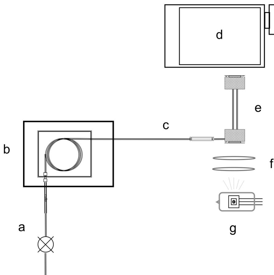
Figure 7.1. Pyrolysis-GC-UV system. a) pyrolyzer, b) SRI 8610 gas chromatograph, c) transfer line, d) Chromex 250is spectrometer, e) absorption cell, f) silica lenses, g) deuterium lamp.
